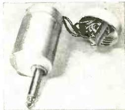
shown in the photo so that, when the canister is closed, the jack won't interfere with the plug. (Also, the offset phono plug allows the adapter to be used with receivers, such as the Drake SW-4A, that have a panel extension.) Wire the two "signal" contacts on the jack and the "signal" contact on the plug together. Do the same for the "common" contacts. Finally, screw on the canister top, and the adapter is ready to use. —A. A. Wicks
