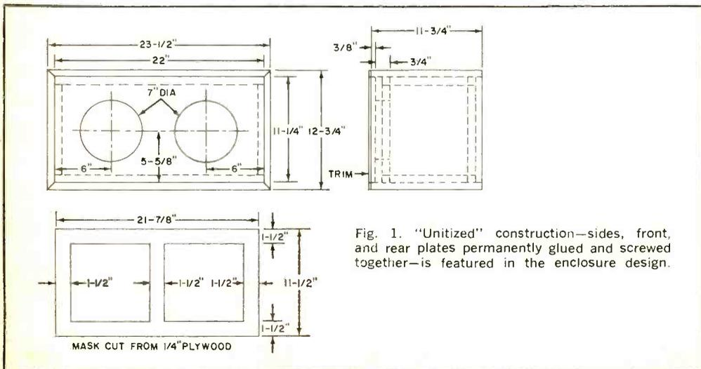
Fig. 1. "Unitized" construction—sides, front, and rear plates permanently glued and screwed together—is featured in the enclosure design.
