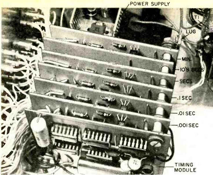
Fig. 9. Timing module and DCU circuit boards should be stacked for space conservation and neatness. Use 1/2"-long insulated spacers (or metal spacers and fiber washers) between each board for adequate separation. Board designations from bottom to top are M2 through M8.
