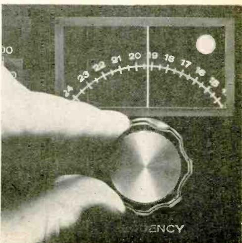
Galaxy R-530 uses "phase lock" principle to set 59 separate tuning bands each 500 kHz wide. The R-530 is the only all-band SWL receiver reported on in this article.
