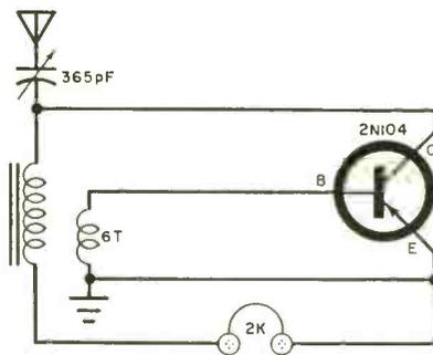
BCB loopstick with about six turns of #22 wire wound at one end of the coil. You may have to reverse the connections to the secondary winding to get best results.
