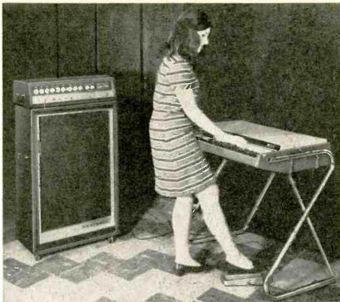
The combo organ is played standing up, using right or left foot to control volume. Organ must be fed into power amplifier. Legs are detachable and can be carried in their own case. A cover snaps over the keys and the organ becomes a second suitcase. In background is Heathkit TO-17 high-power amplifier featuring variety of inputs and speaker unit.
