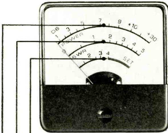
1. Built-in SWR bridge lets you tune your antenna for maximum output.
