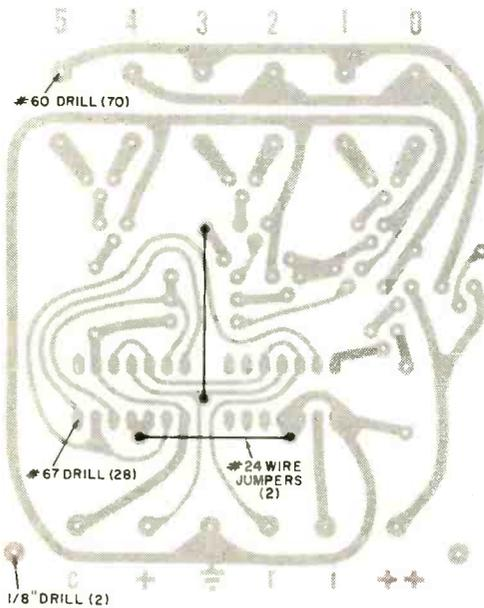
Fig. 3. Drill the PC board as shown here, and add the two insulated jumpers on component side of board.
