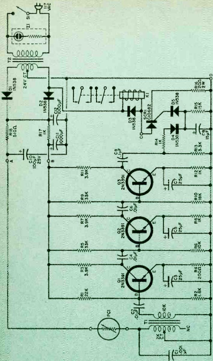
Fig. 8. Because the demodulator is a high-gain amplifier, take care that the input circuit is not loaded where it can pick up stray signals. This could lead to erratic operation. The lettered and open small circles on the diagram are the printed-board connections.
