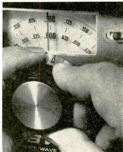
Drake SW-4A and R-4B has two separate adjustments for setting dial accuracy. Hairline can be moved by button in upper right. Skirt of tuning knob may be slipped so that 0-25 scale agrees with hairline and pointer.
