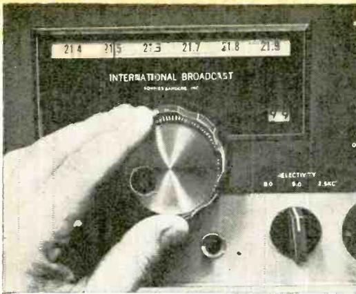
Squires-Sanders IBS receiver has the eight main international broadcast bands calibrated on a slide rule dial. Figures visible in window are on digital rotary wheels and denote kilohertz. Three position selectivity control is also seen. This custom-made receiver is used by the VOA.
