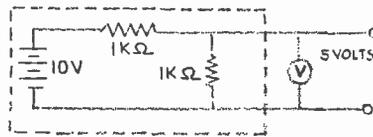
With the switch open and the load disconnected, the output is 5 volts with 5 mA in the output resistor. Closing the switch puts the 2000-ohm load in parallel with the output resistor so that the 6 mA now drawn from the source divides: 4 mA through the output resistor and 2 mA through the load resistor.
