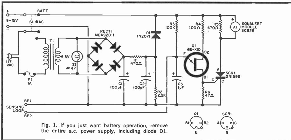
circuit that does not allow the Prowler Howler to sound off until the circuit is broken. Depending on the installation, there are several ways in which the closed loop can be produced. A typical home installation is shown in Fig. 3. For windows and doors, you can stretch a length of very fine wire (#38 magnet wire is recommended) across the opening, with each end secured by a piece of
