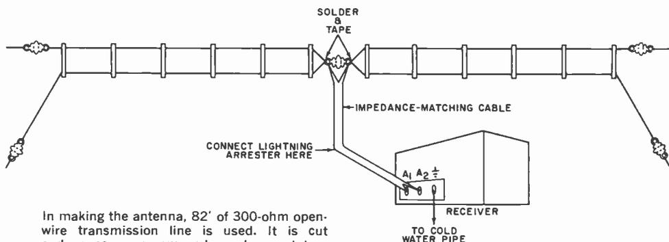
In making the antenna, 82' of 300-ohm open-wire transmission line is used. It is cut and spacers are removed as shown at top, folded and connected together as at bottom.
