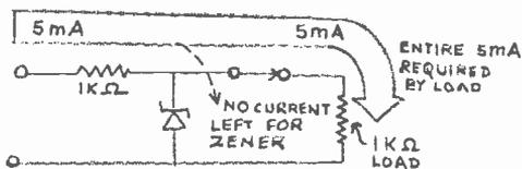
With no current available for the zener diode, it ceases to conduct, and the voltage across the load begins to decrease with further decreases in load resistance.
