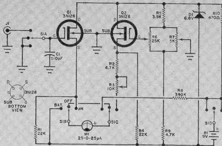
Fig. 1. The symmetrical configuration of the differential amplifier circuit cancels errors caused by temperature and drain-voltage variations in MOSFET'S.
