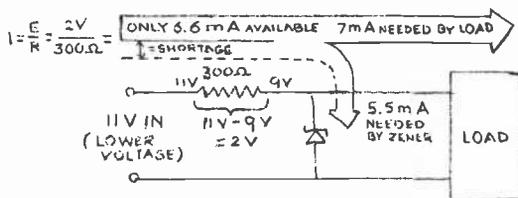
This leaves only 2 volts, dropped across the source resistor, to drive the current through the resistor. As a result, current drops to about 6.67 mA.
