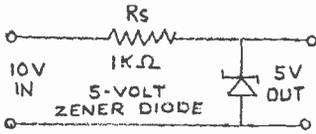
As before with the two 1000-ohm resistors in the circuit, the voltage divides exactly in half so that 5 volts appears at the output. What happens when the input potential is raised to 15 volts? Oddly enough, the output remains at 5 volts as a result of the regulatory ability of the zener diode.
