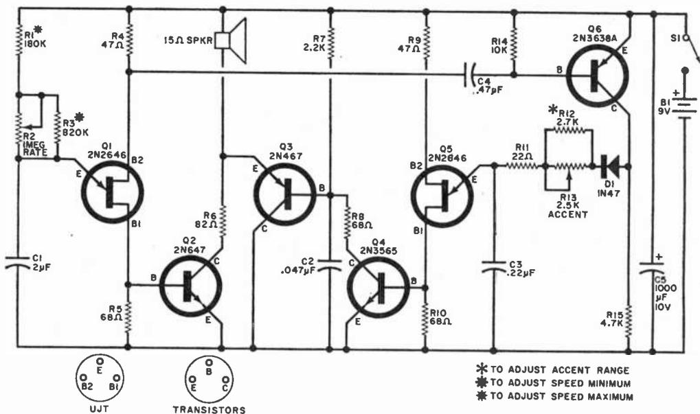
Fig. 1. Beat rate is established by relaxation oscillator Q1, amplified by Q2. The beat is accentuated by circuit Q3 to Q6.
