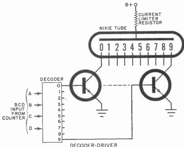
**Testing.** Connect the DCU to a test circuit such as that shown in Fig. 6. Operating the zero-reset switch should cause the Nixie tube to indicate the numeral zero. Operating the nine-reset switch should produce a nine indication on the tube. (The nine-reset connection is used in "nines complement" decimal operations.) Operating the decimal-point switch should cause either the right or the left decimal point to glow. Reset the unit to zero before making the next test.
