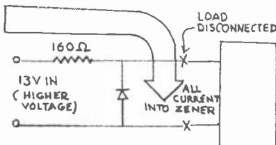
Fortunately, Ohm's law shows that a  $\frac{1}{4}$ -watt resistor will adequately handle the current. Now we have a regulator circuit we can build with confidence.
