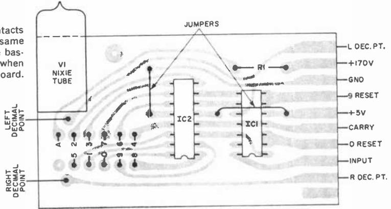
or used with a PC-board edge connector. After mounting and soldering *IC1* in place, install the second jumper.
