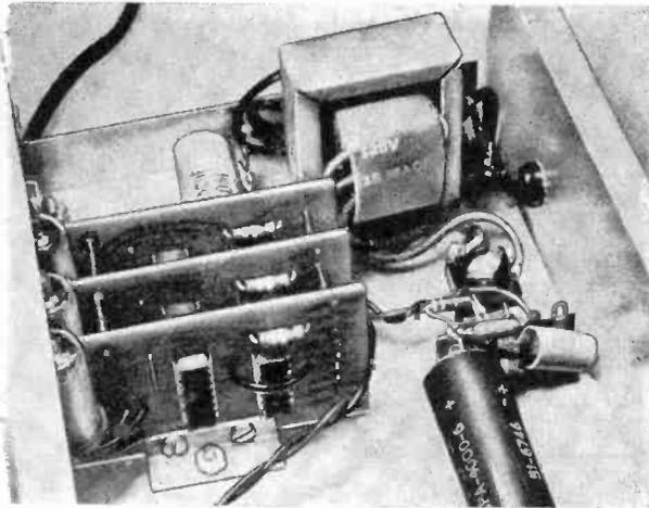
Fig. 5. Terminal strips and point-to-point wiring should be employed when assembling power supply.
