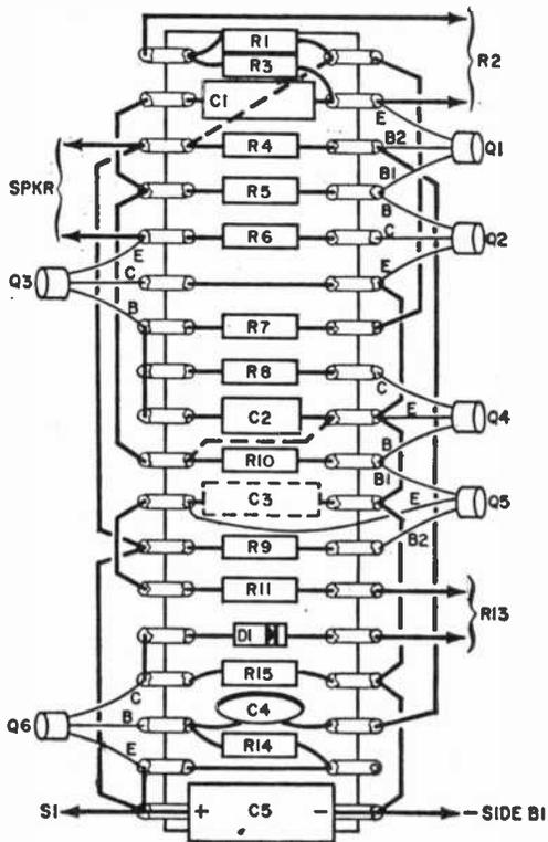
Fig. 3. Route capacitor C3 and wiring indicated by dashed lines along the underside of the tag strip.
