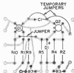
Fig. 3. To protect MOSFET's against damage, connect temporary jumpers as shown until meter is fully assembled.
