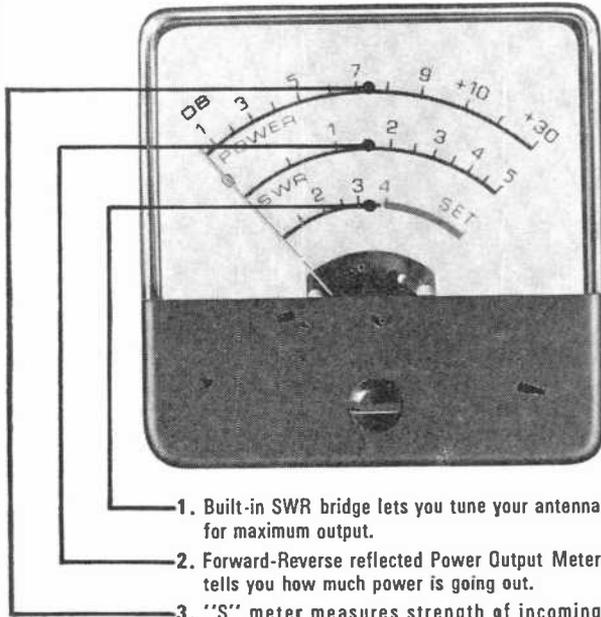
1. Built-in SWR bridge lets you tune your antenna for maximum output.
