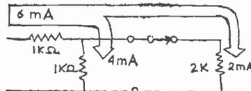
Using Ohm's law,  $E_{out} = 2000 \times 0.002 = 4$  volts. What happens is that the load resistance shunts the output resistance, decreasing the total resistance "seen" by the source and reducing the voltage drop across the load.
