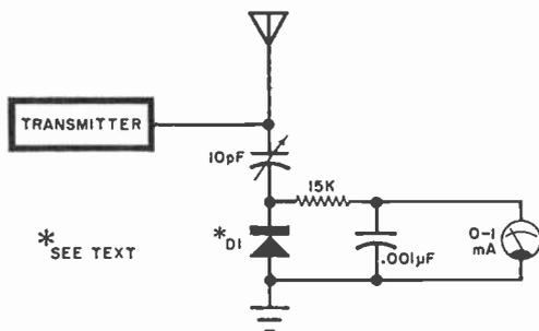
cause it also tells what the antenna is doing, the circuit shown above can be wired into your rig. The diode, DI, can be almost any signal diode you have at hand.
