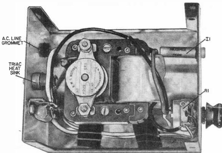
Fig. 3. When testing the magnetic stirrer with the top off, be sure not to touch any of the wiring since all of the circuit is connected to the a.c. power line. Do not use the metal chassis as a common tie point for any of the circuit.
