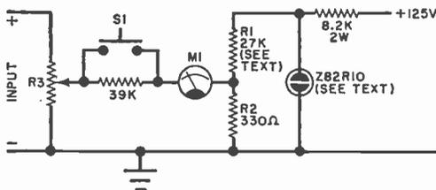
Fig. 14. The neon lamp specified here provides a reference voltage across  $R2$  of  $1 \pm 0.012$  volt. This is compared to the input in the null-indicating meter, making a highly accurate precision voltmeter.
