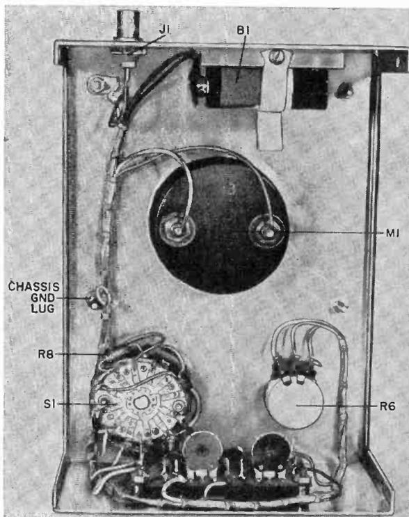
Fig. 5. After components and circuit board are mounted in their respective locations on the metal box, wire them together. To obtain a neat, professional appearance, use lacing cord to bundle the wires into harness configuration as shown in this photo.
