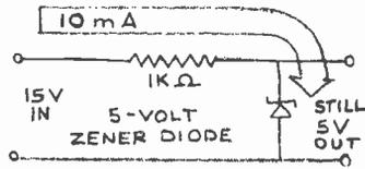
This shows that, while a resistor behaves according to Ohm's law, the zener diode disregards it, changing its effective resistance as needed to provide a constant output voltage.
