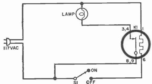
With *S1* at OFF, lamp and *K1* receive power until thermal action opens relay's bimetallic contacts.
