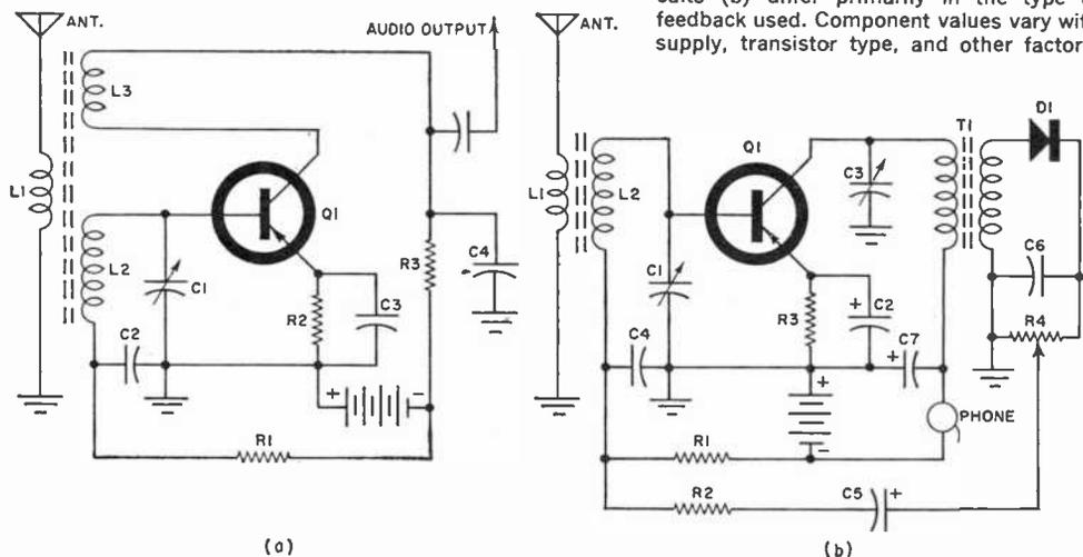
Fig. 4. Regenerative (a) and reflex circuits (b) differ primarily in the type of feedback used. Component values vary with supply, transistor type, and other factors.
