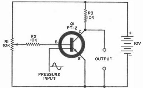
Fig. 3. The Pitran is a pressure-sensitive transistor which can be used in a standard transistor audio-amplifier circuit for various applications.
