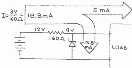
We have paid a price for our regulator, however, in the form of 13.8 mA wastage current through the zener diode. The advantage is that the receiver will operate reliably no matter what happens.
