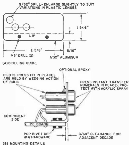
Fig. 12. Arrange lamp mounting holes in two closely spaced, staggered columns to obtain small size.
