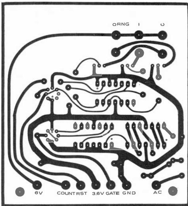
Fig. 6. Actual-size etching guide must be copied exactly as shown to insure proper component fit. Small dots near solder terminals indicate IC indexes.
