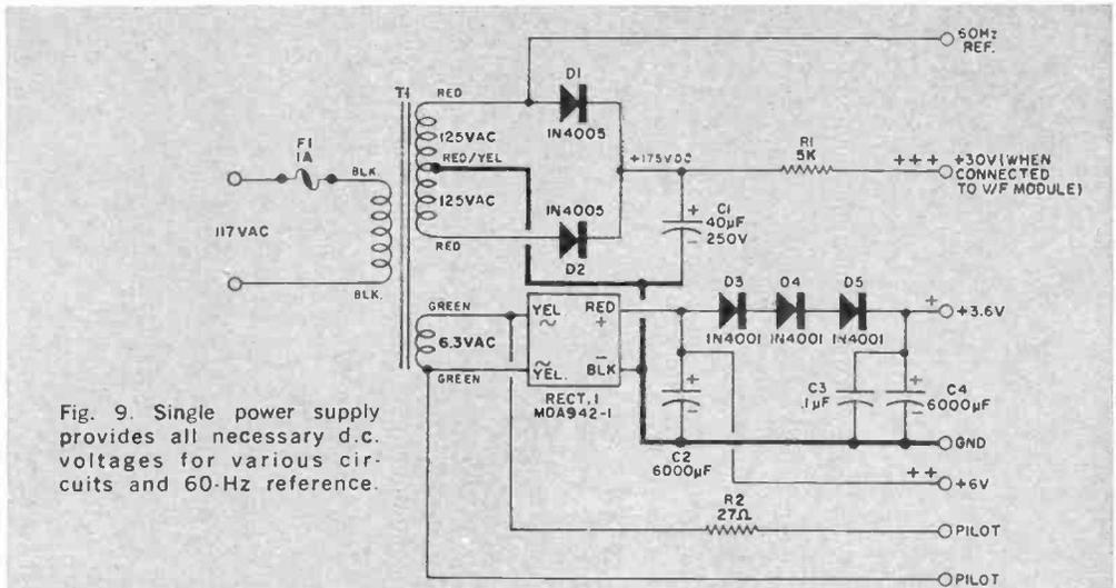
Fig. 9. Single power supply provides all necessary d.c. voltages for various circuits and 60-Hz reference.
