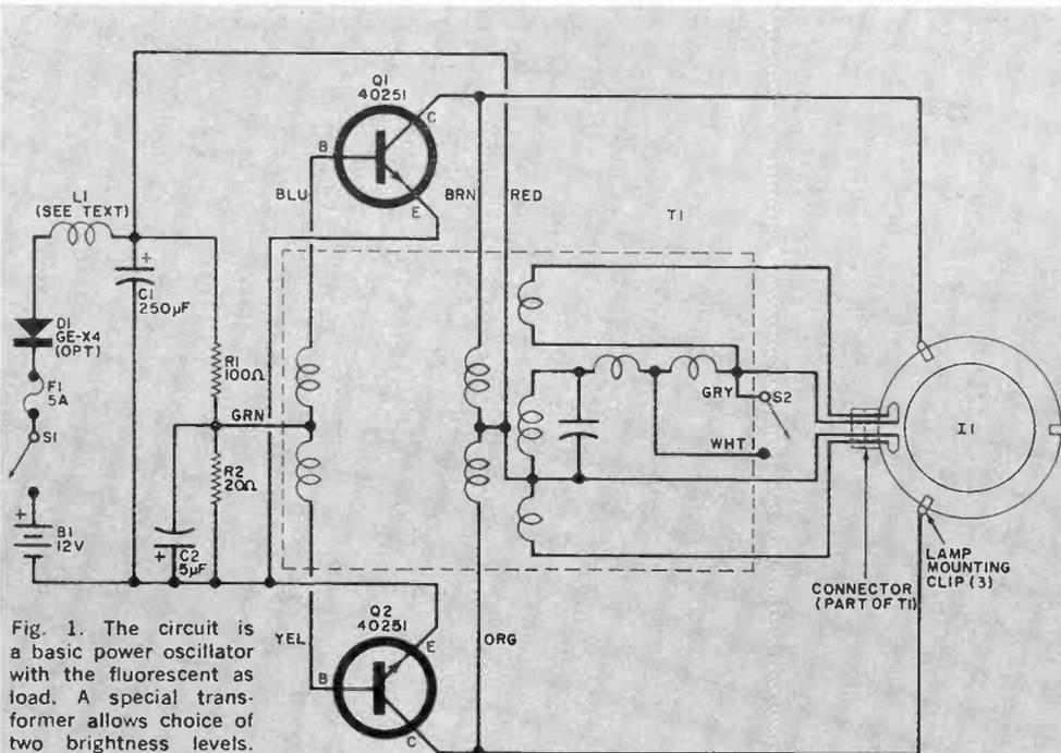
Fig. 1. The circuit is a basic power oscillator with the fluorescent as load. A special transformer allows choice of two brightness levels.
