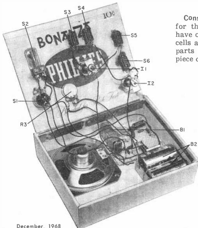
**Construction.** Many of the parts needed for the Gadget Box you will probably have on hand. Except for the speaker, D cells and holder, lamps, and controls, all parts can be mounted on a 3"-square piece of perforated board, using flea clips (Continued on page 109)
