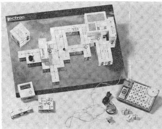
Raytheon-Lectron (upper left) and Denshi-Block kits form a class by themselves. Components in each are housed inside plastic, component-keyed cubes or blocks. Raytheon-Lectron kit is large and easy to work with, while Denshi-Block is compact and portable.
