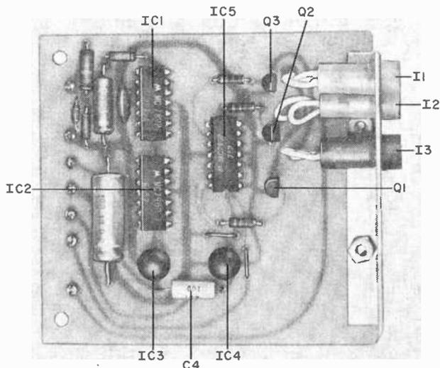
Photo of author's prototype shows properly wired Gate module board with indicator lamps and bracket in place and optional solder terminals at left; external wiring can be soldered directly to board.
