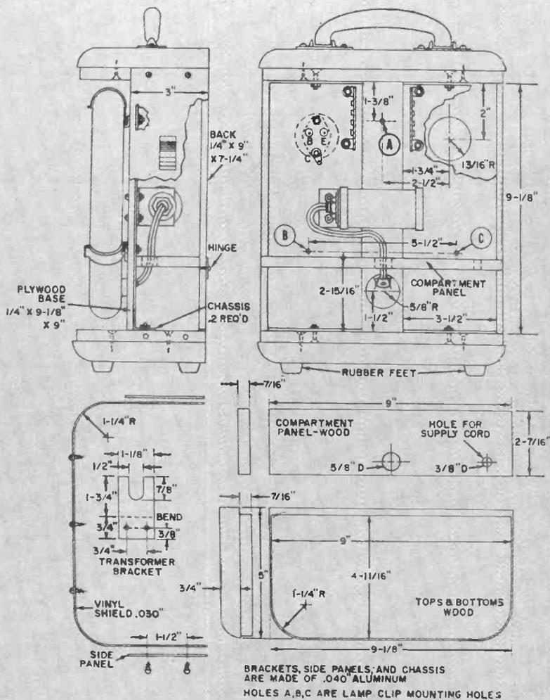
Fig. 2. If you want to duplicate the author's prototype, follow the construction details shown here. Note that the two transistors are mounted through the wooden front panel and the metal chassis. All wiring is done after components are mounted.
