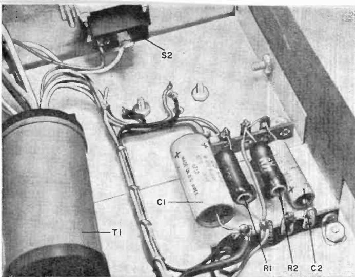
Resistors and capacitors are mounted between two terminal strips. Note how a wire harness makes for a clean, neat internal arrangement. This photo also shows the two isolated metal chassis and the method of wiring the power transistors. Both the emitter and base connections are soldered direct to the transistor leads; the collector connection is made to a solder lug under the collector (and case) mounting hardware.
