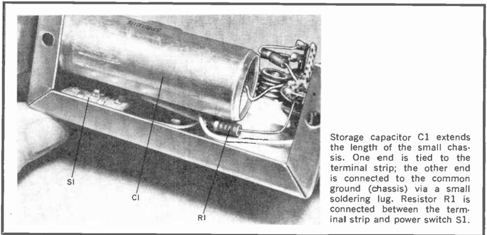
Storage capacitor C1 extends the length of the small chassis. One end is tied to the terminal strip; the other end is connected to the common ground (chassis) via a small soldering lug. Resistor R1 is connected between the terminal strip and power switch S1.
