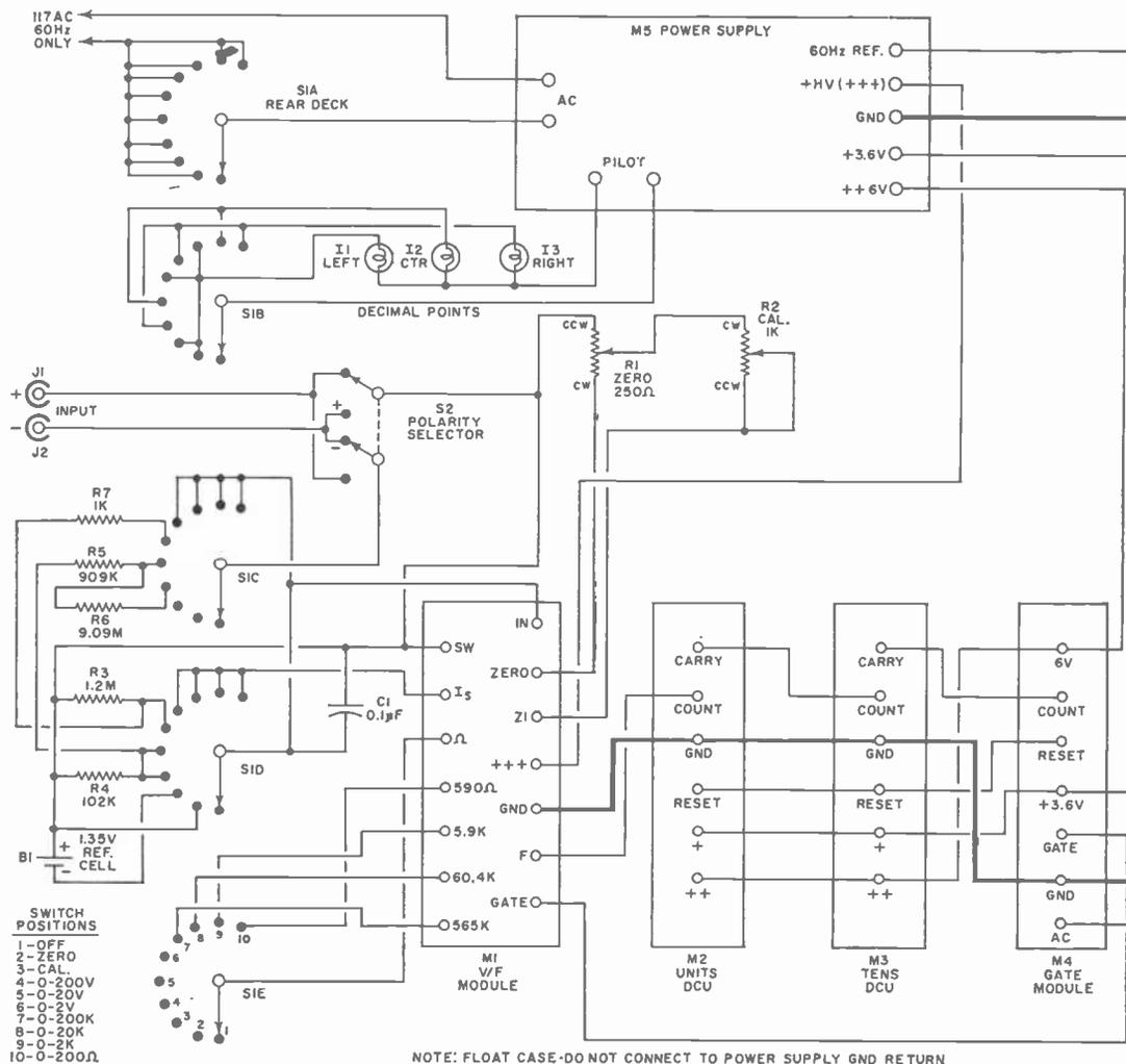
Fig. 13. The heavy line connecting the GND terminals in this overall wiring diagram is NOT a chassis ground; it is a convenient floating common bus.
