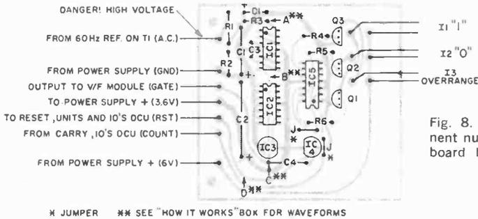
Fig. 8. Double and triple check component numbers, values, and orientation on board both before and after soldering.
