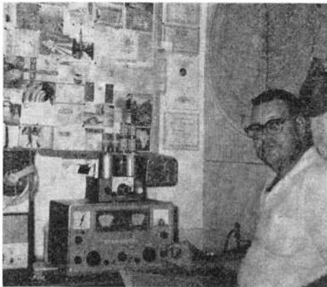
Del Hirst, WPE5CFU, Snyder, Texas, has a Hammarlund HQ-100 receiver. Atop it is a homemade W6SAI preselector and at left is an Airline monaural, dual-track tape recorder. Del has 99 states verified.
