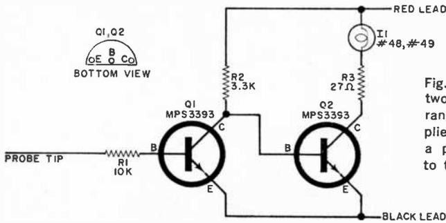
Fig. 1. The probe is a simple two-transistor lamp driver arrangement. With no signal applied, the lamp is lit. When a positive voltage is applied, to the tip, the lamp goes out.
