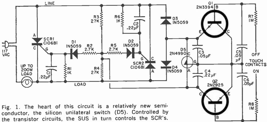
Fig. 1. The heart of this circuit is a relatively new semiconductor, the silicon unilateral switch (D5). Controlled by the transistor circuits, the SUS in turn controls the SCR's.
