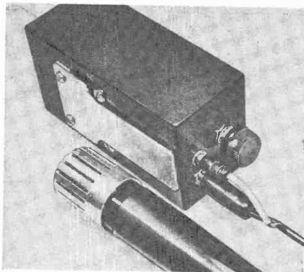
A metal strap arrangement can be mounted on the rear of the plastic case so that the wireless microphone can be carried on the user's belt. The microphone can be hand carried or mounted on a neck strap for lavalier mike.
