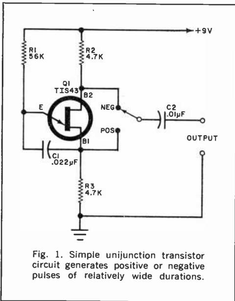
Fig. 1. Simple unijunction transistor circuit generates positive or negative pulses of relatively wide durations.
