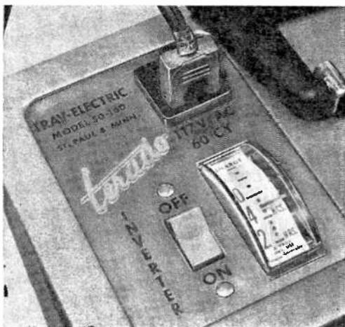
Faceplate contains a dual function meter. When battery is charging, the meter reads approximate charging current. When discharging, the meter reads the approximate time the inverter will operate—if the battery was fully charged to begin with. Your reviewer found the meter readings ambiguous since meter action did not appear linear.
