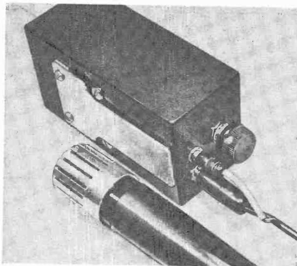
A metal strap arrangement can be mounted on the rear of the plastic case so that the wireless microphone can be carried on the user's belt. The microphone can be hand carried or mounted on a neck strap for lavelier mike.
