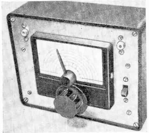
The marine-band converter provides for reception of transmissions on the 2-to-3-MHz band on any conventional AM broadcast-band radio. Coupling is through the antenna input terminals on BCB receiver.
