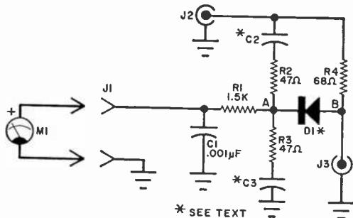
With system completely set up, reactive imbalances between A and B cause up-scale meter deflection.
