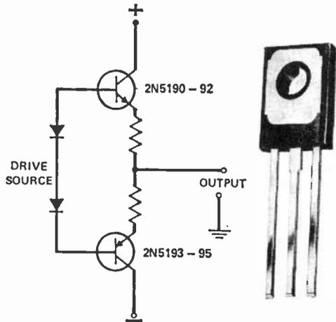
Fig. 4. Complementary silicon transistors have 4-ampere, 35-watt ratings in voltages from 40 to 80.
