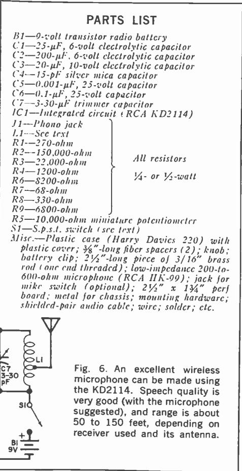
Fig. 6. An excellent wireless microphone can be made using the KD2114. Speech quality is very good (with the microphone suggested), and range is about 50 to 150 feet, depending on receiver used and its antenna.
