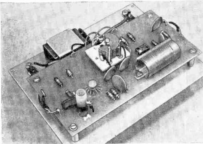
Interior of the marine-band converter shows the neat construction that can be obtained. Although it looks like a PC board, this unit uses perf-board wiring.
