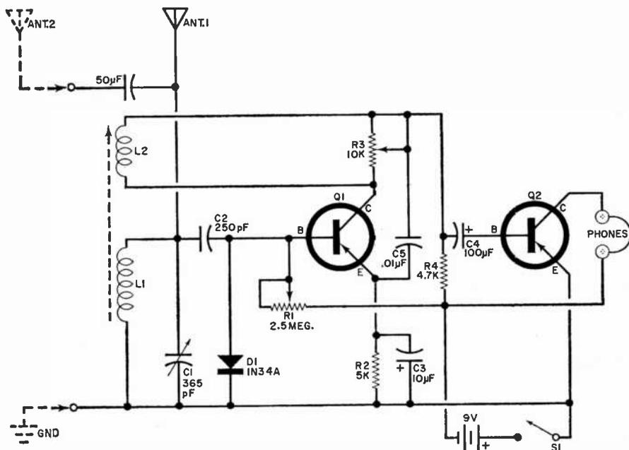
Fig. 2. In this two-transistor receiver circuit, regenerative feedback is used in Q1 portion of the circuit while Q2 serves as a capacitively coupled audio amplifier. Use 2000-ohm phones.
