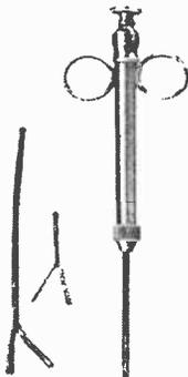
that eliminates most of the time and effort normally required for the preparation of the conductors in shielded cable. The point of the tool is inserted between the braid and inner conductor, parting the shield from the inside without breaking wires. A plunger is then depressed, ejecting the inner conductor through the previously formed exit hole. No trimming of the conductors is needed, so the
