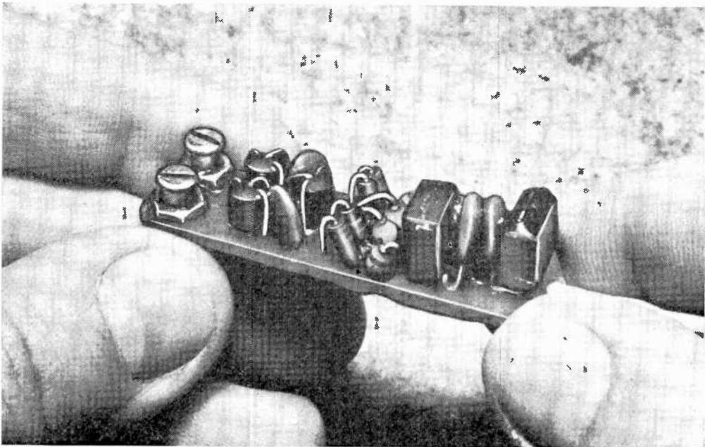
Once the board has been completed and tested, it should be encapsulated with an insulating material to prevent possibility of electrical shock. Only the two screws at left are exposed for external contacts.
