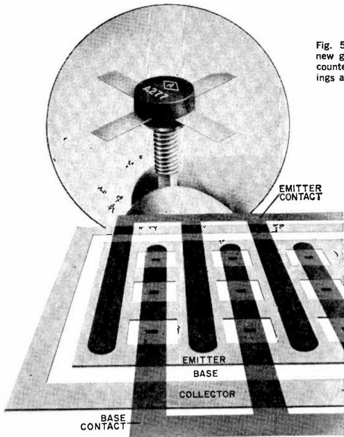
Fig. 5. R.f. power transistors have new geometry to carry overloads encountered in VHF transmitters. Ratings are 12.5 or 28 volts, 3 to 22 W.
