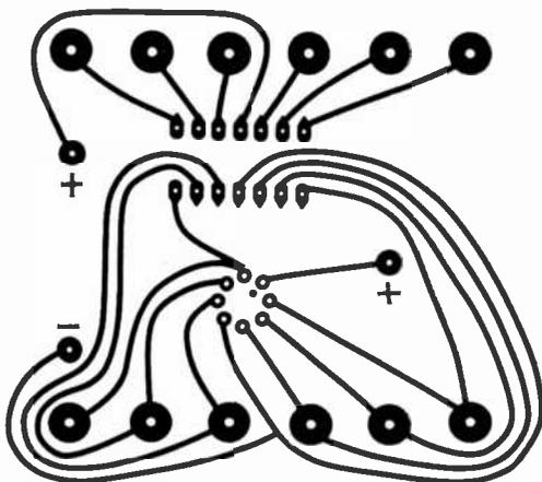
Fig. 6. Actual-size foil pattern for the socket-contact board. Switch S1 cutout and mounting holes are dependent on the particular switch you are using.
