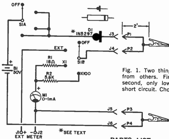
Fig. 1. Two things make this ohmmeter different from others. First it requires no zero control; second, only low current can flow, even with a short circuit. Choice of D1 determines the current.
