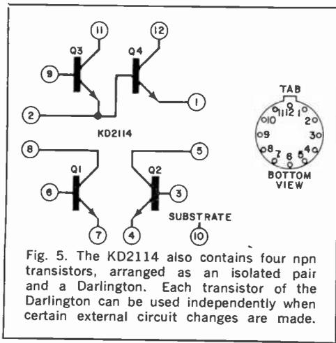
Fig. 5. The KD2114 also contains four npn transistors, arranged as an isolated pair and a Darlington. Each transistor of the Darlington can be used independently when certain external circuit changes are made.
