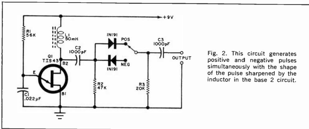
Fig. 2. This circuit generates positive and negative pulses simultaneously with the shape of the pulse sharpened by the inductor in the base 2 circuit.
