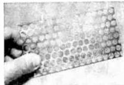
stock. This material, which forms the outer wall of the filter, can be cut to size with tin snips or heavy-duty scissors.
