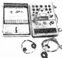
meter circuit and neon lamps. The Model 88A utilizes "grid circuit tests" to make up to eleven simultaneous checks for leakage, shorts, and grid emission or current reversal—not to mention tube merit and filament continuity. Setup data for multiple tests are arranged on handy flip-over cards. The card system is automatically kept current free of charge for registered owners.
