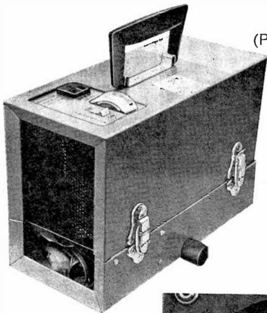
Self-contained Trav-Electric inverter weighs about 29 lb. A 43-plate garden tractor wet battery is inside protective metal case. The battery may be recharged from either 117-volt a.c. line or cigarette lighter socket in your car. Both recharging cables are tucked inside case when not in use. Rubber bumpers on sides of case help protect the supply while in transit.
