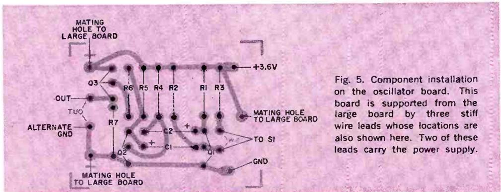
Fig. 5. Component installation on the oscillator board. This board is supported from the large board by three stiff wire leads whose locations are also shown here. Two of these leads carry the power supply.
