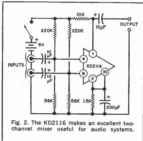
Fig. 2. The KD2116 makes an excellent two-channel mixer useful for audio systems.
