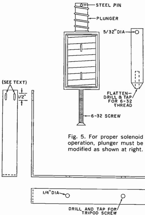
Fig. 5. For proper solenoid operation, plunger must be modified as shown at right.
