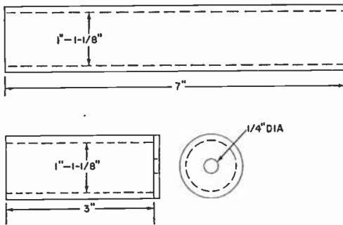
Fig. 3. Fabricate light shields illustrated here from mailing tube; note aperture disc on short tube.
