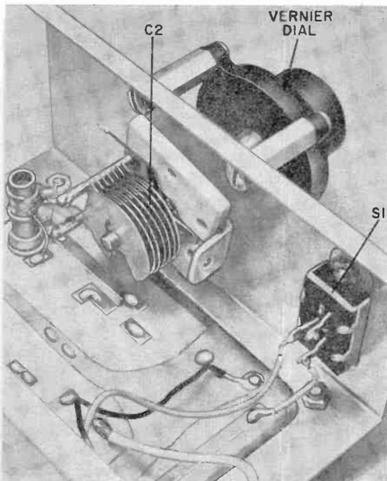
Before mounting vernier dial, rotate shaft of C2 until capacitor plates are fully meshed and knob on vernier dial is on zero position so that C2 and vernier dial rotate stop-to-stop in unison.
