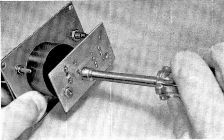
Once the circuit is assembled, secure it to the meter screw terminals. Electrical connections to the meter are made via printed circuit wiring. Drill a small hole through the PC board to provide screwdriver access to R2.
