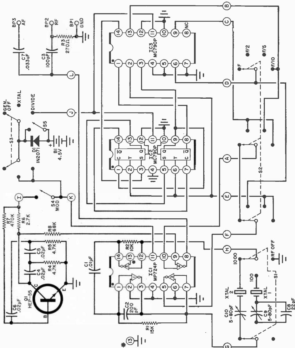
Fig. 1. The circuit consists of a switch-selectable crystal oscillator followed by a switch-selectable countdown module up of JK flip-flops. This enables a broad range of r.f. outputs. A built-in audio modulator helps identify r.f. signal.
