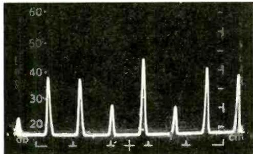
These waveforms were taken from a Squires-Sanders "Bandscanner." Upper left shows spread of 10-kHz pips centered at 7250 kHz (hump due to receiver tuning). Upper right shows 20-kHz pips centered at 25,850 kHz. Lower left are 10-kHz pips centered at 25,850 kHz, and lower right are 50-kHz pips centered at 25,850 kHz. In all cases, the pips are clean and distinct, permitting accurate frequency calibration down to 10 kilohertz.
