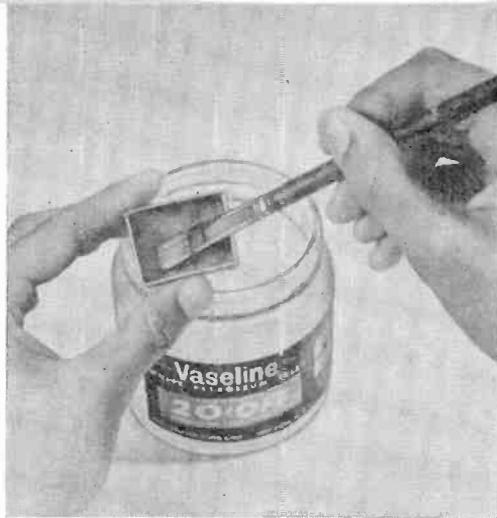
To prevent potting compound from adhering to form, liberally coat all interior surfaces of the form with Vaseline using a brush or a scrap stirrer.
