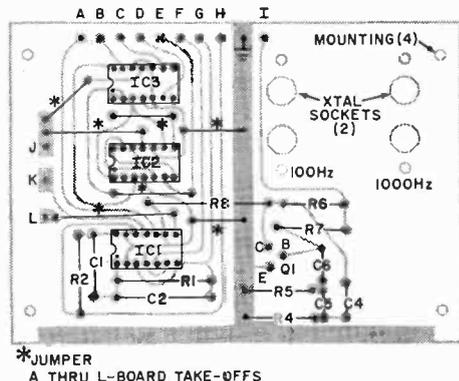
Fig. 3. Component installation. Observe notch and dot code on IC's to ensure proper installation. The values of  $R7$  and  $R8$  may have to be adjusted, so mount them on flea clips to facilitate changes.
