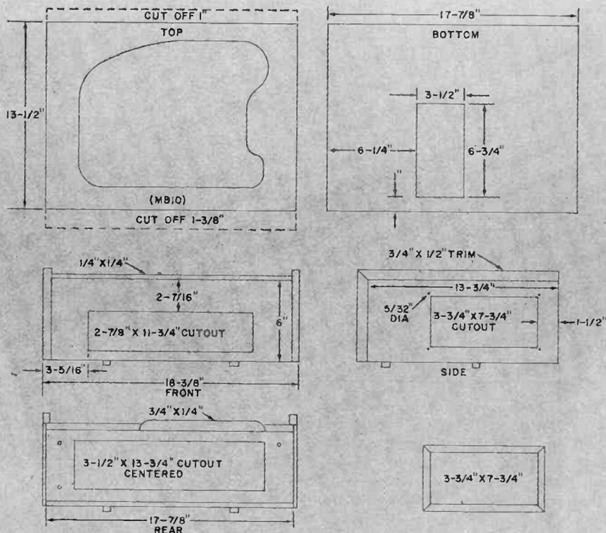
Fig. 1. Be sure, when removing excess material from the MB10 turntable base board, that the assembly is oriented as shown in the drawing at the upper left.
