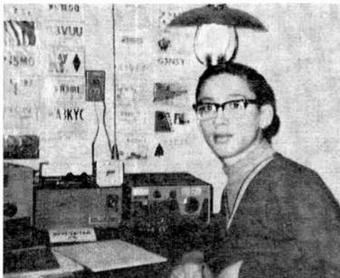
Tom, WN3KQA, Aliquippa, Pa., has 48 states and 11 countries using a Heathkit HX-11 transmitter, a Drake R-4A receiver and 40- and 15-meter dipoles.
