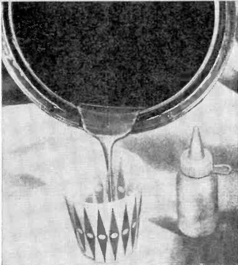
Using wood stirrer and paper cup, mix just enough resin compound and hardener to pot circuit adequately. (See mixing instructions on resin can.)
