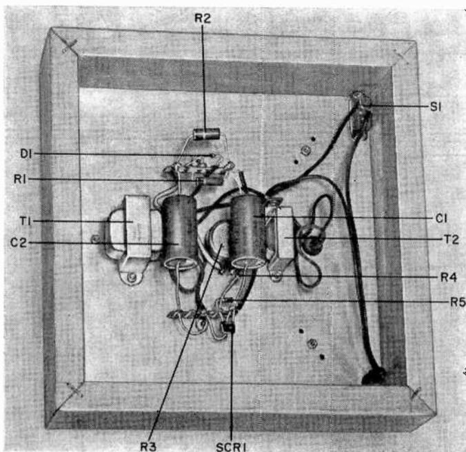
The author's PPFL before installing the music portion. The added components can be fitted into one of the empty corners. It is not necessary to mount the fluorescent lamp on this chassis, and almost any type of lamp holder will suffice. Just make sure that the lamp cannot be accidentally broken.
