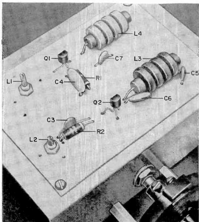
All components in converter circuit (except B1, C2, S1, and J1) mount directly on circuit board. Note orientation of case flats and leads on both transistors.
