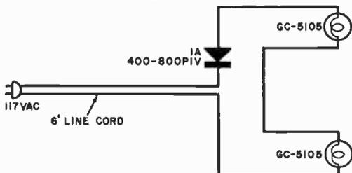
The diode can be any rectifier type; polarity is not important. With diode cutting the voltage in half, small lamps put out more than enough light.
