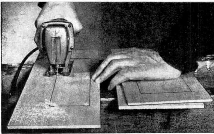
Sabre saw is best for making cutouts in thin plywood. If sabre saw is not handy, carefully use crosscut keyhole saw.
