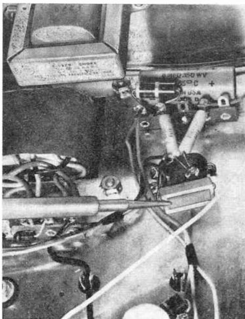
Pointer shows filter resistor to be removed and replaced with filter choke mounted to side of chassis.
