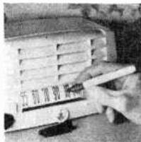
and the enamel cracks and falls out of the marking grooves. It is a messy and sometimes impossible job to clean some cabinets—notably plastic types—without causing further damage to the markings. However, in the case of white and ivory cabinets
