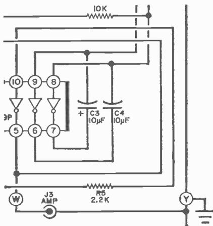
"Build the Two-Tone 'Waverly' Alarm" (February 1970). The schematic diagram, Fig. 1 on page 30, shows  $R_6$  and  $R_7$  connected to the incorrect pins on  $IC_1$ . In the partial diagram above the correct connections are shown.
