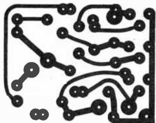
Fig. 2. Actual size printed circuit etching guide is shown at left. Photo below shows component placement (except S1) on board.
