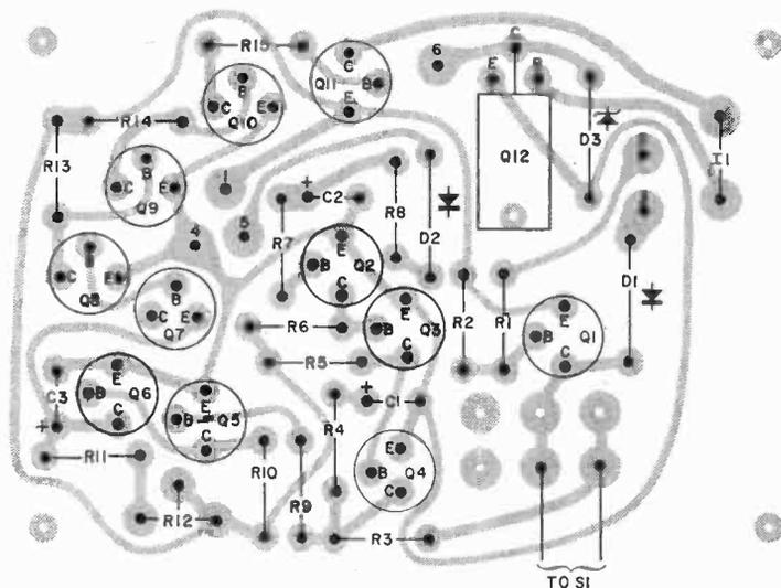
A printed circuit board (Fig. 2) should be used in the construction. (See Parts List if you want to buy one already etched and punched.) Mount the components on the board as shown in Fig. 3.
