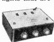
electronic signal. High-power outputs (500 watts/channel) provide power sufficient to transform a large room into a total light/sound environment. The light organ employs three
