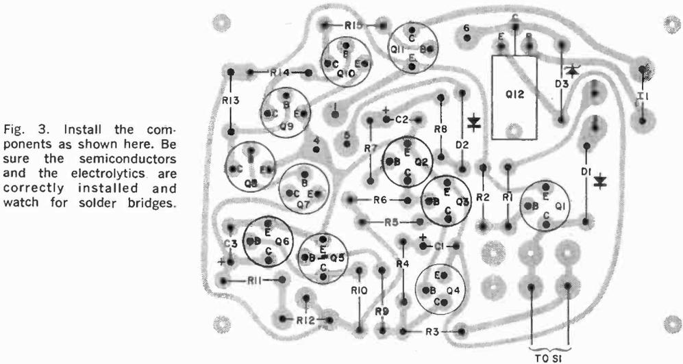
Fig. 3. Install the components as shown here. Be sure the semiconductors and the electrolytics are correctly installed and watch for solder bridges.
