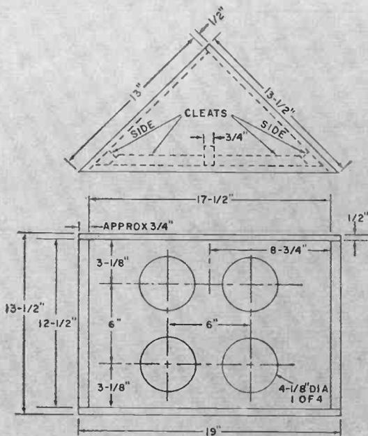
Fig. 1. Due to small size and triangular configuration, enclosure can be almost entirely assembled with nails only.
