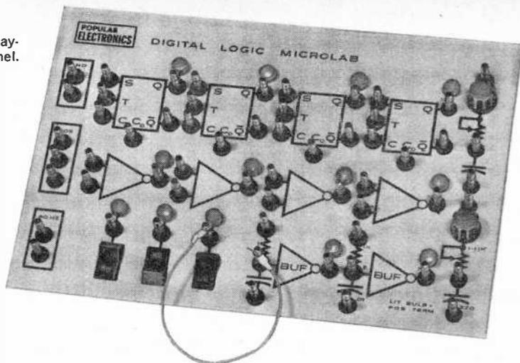
pushbuttons or slide switches. The latter are bounceless and can drive all logic blocks. If desired, certain blocks may be interconnected to form oscillators for driving or test purposes.
