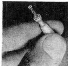
in blind places. But with a length of scrap irradiated polyvinyl chloride ("heat-shrinkable" PVC) tubing, you can fashion your own nut starters for virtually any size hardware. All you need do is select a size tubing that just fits the hardware. Insert the nut at one end of the tubing, flush with the tubing's edge. Apply heat until the tubing shrinks snugly around the nut. —Stephen E. Maziarz
