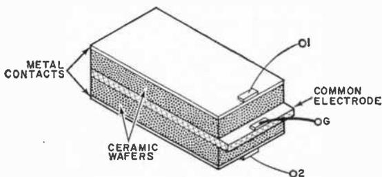
to input signals in a narrow frequency range. The other, designated an adaptive ferroelectric transformer, responds to input signals covering a broad frequency spectrum.
