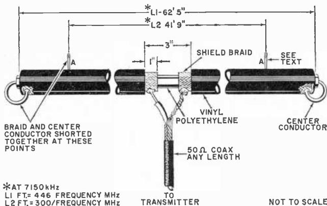
Homebrew dipole made of coax has a standing wave ratio very close to 1:1 over the entire 40-meter band. Large effective diameter helps to broaden the antenna's frequency response.
