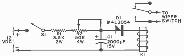
**Reader's Circuit.** Quite often, any of a variety of circuits may be used to achieve a specific goal. A good example of this can be found in the stirring "Saga of the Slow-Kick Windshield Wiper." The slow-kick operation is to provide slow wiper movement for use under such marginal driving conditions as mist or drizzle, where there is inadequate moisture to lubricate the wiper blades in continuous action, yet enough to require occasional cleaning.
