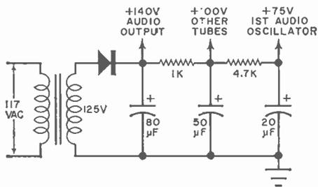
Half-wave rectification and RC filtering are hallmarks of most inexpensive receiver power supplies.
