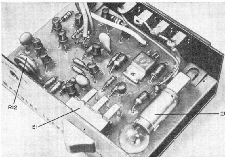
When mounting the PC board in the metal chassis, make sure that you can gain screwdriver access to *R12* so that delay time can be externally adjusted as desired. If you have no need to vary this time, the chassis hole can be eliminated.
