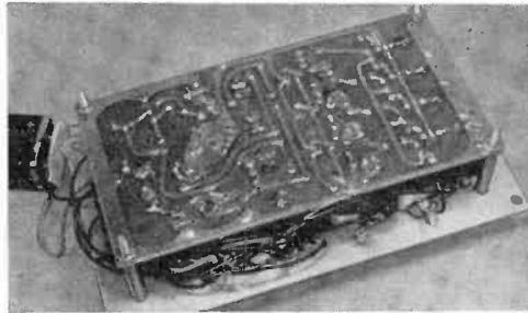
The Four-Trace Pre-Amp is constructed on a PC board, with controls and jacks mounted on metal front panel. Complete pre-amp, with battery, fits compactly within plastic case that is provided.
