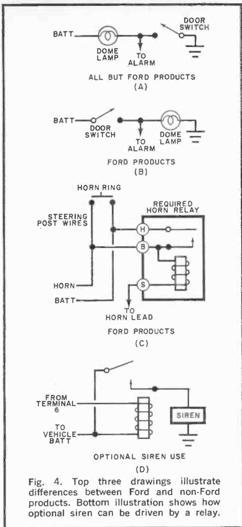
(ground). Connect the lead from terminal 5 to either side of the fuse that supplies the radio (or any other accessory that is powered only when the ignition key is in either the ignition or accessory position).
