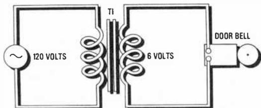
In this door bell circuit, which kind of transformer is T<sub>1</sub>—step-up or step-down?
