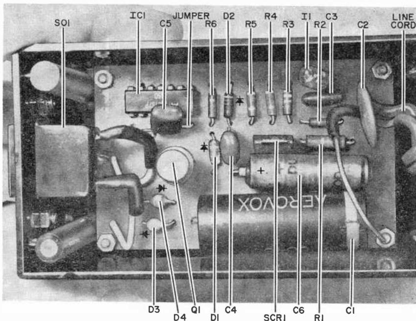
circuit board (see Fig. 2 for etching guide and part location photograph) and mounted inside a plastic case that is equipped with an aluminum cover. The metal cover will then serve as a convenient touch plate.
