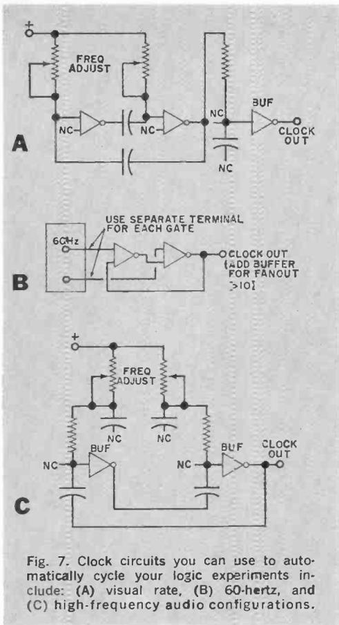
Fig. 7. Clock circuits you can use to automatically cycle your logic experiments include: (A) visual rate, (B) 60-hertz, and (C) high-frequency audio configurations.
