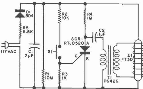
Fig. 3. Relatively simple electronic photoflash circuit uses low-cost plastic-encapsulated SCR.
