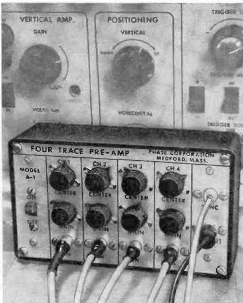
Four coaxial cables terminated in alligator clips are used to connect channels to multiple inputs. One output cable goes directly to vertical input on single-trace scope, while the other provides the scope with sync from the signal at channel 1.
