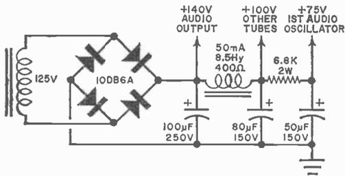
Full-wave bridge rectification and LC filtering remove most of the a.c. ripple from the d.c. output.
