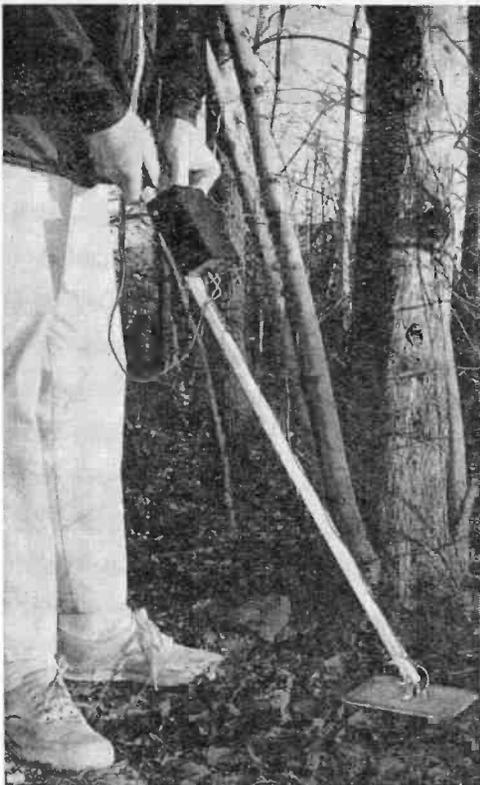
The metal/mineral locator is very light in weight and easy to use. Angle of search coil plane may be changed to suit convenience of user. Support pole is in two pieces and can be folded up into a relatively small package to fit in a car trunk.
