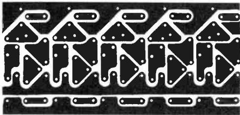
Now, using your template and/or rule, start filling in hole locations and foil patterns in the same sequence as in your conductor pattern diagram. Condense the areas on which the components are to be mounted for maximum space utilization. However, do not be afraid to assign a component more space than it requires if you want to preserve symmetry of the layout or to prevent thermal problems.
