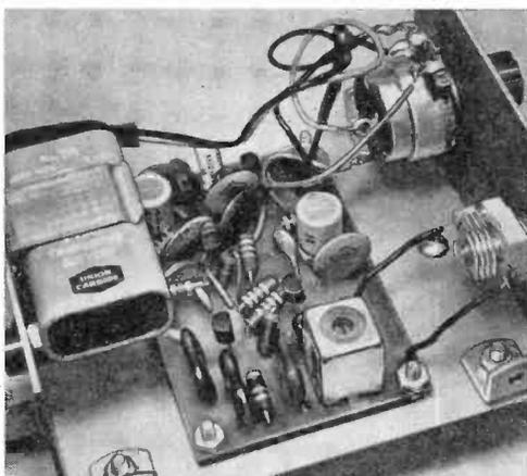
Most of electronics package is on a PC board. Use care in soldering in the 5 transistors (3 FET's). Assembly of board took your reviewer about 1½ hr.
