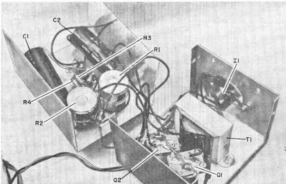
Due to simplicity of circuit, point-to-point wiring, using stranded hookup wire, is best for assembling project. Mount controls on front, lamp and lens assembly to top of chassis box.
