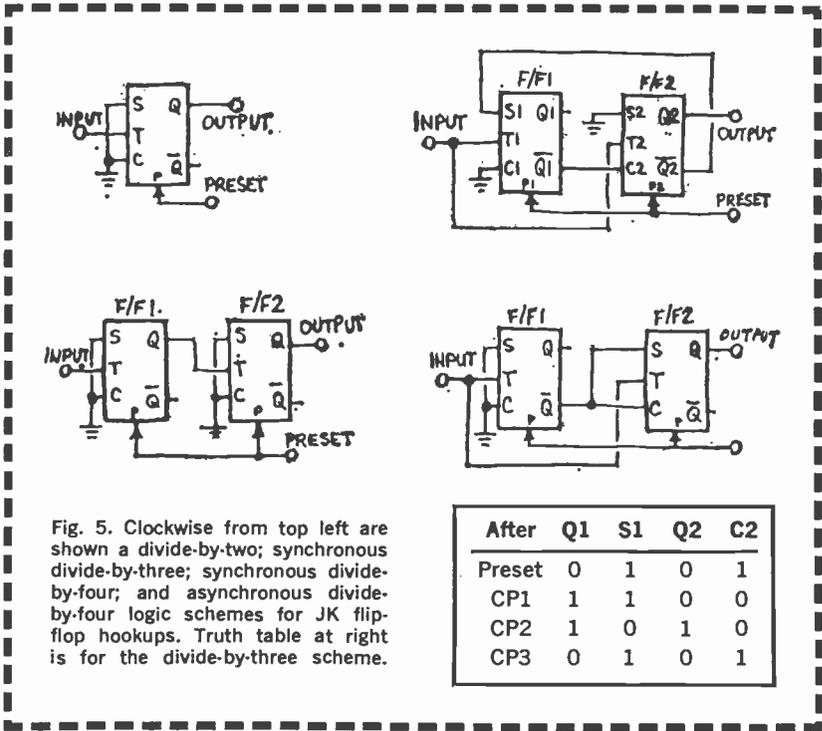
Fig. 5. Clockwise from top left are shown a divide-by-two; synchronous divide-by-three; synchronous divide-by-four; and asynchronous divide-by-four logic schemes for JK flip-flop hookups. Truth table at right is for the divide-by-three scheme.
