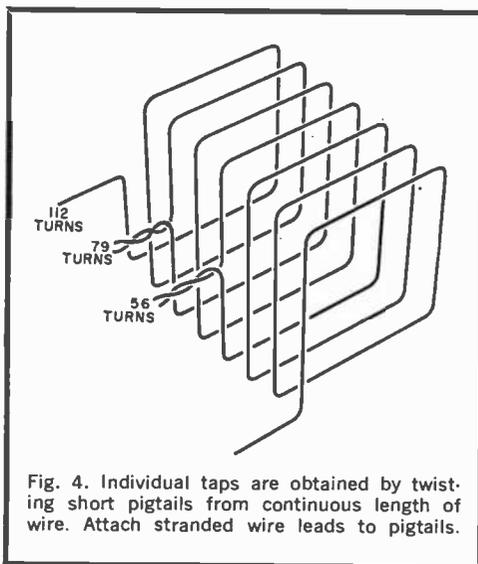
Fig. 4. Individual taps are obtained by twisting short pigtails from continuous length of wire. Attach stranded wire leads to pigtails.
