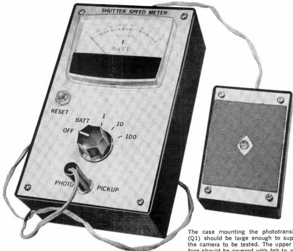
The case mounting the phototransistor ( $Q1$ ) should be large enough to support the camera to be tested. The upper surface should be covered with felt to avoid scratching the face of the tested camera.
