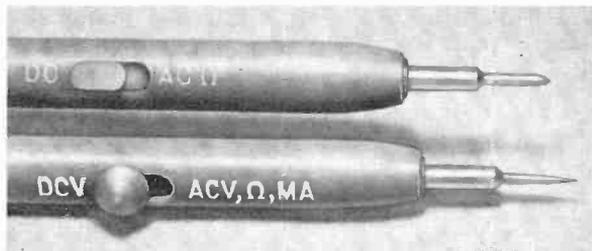
**PROBES—NEW and OLD:** Triplet made two minor and one major change on the test probe. There is a bigger slide switch button, brighter and bigger lettering and a needle point vs the old tip pin of the 602 probe. Alligator clips are supplied.
