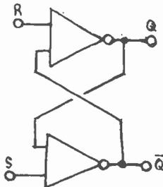
Fig. 2. Schematic and logic diagrams of SR flip-flop are shown above. All possible circuit states are indicated in truth table.
