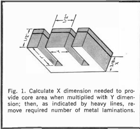
Fig. 1. Calculate X dimension needed to provide core area when multiplied with Y dimension; then, as indicated by heavy lines, remove required number of metal laminations.
