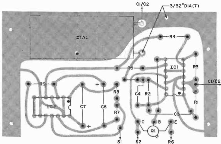
symmetrical cross-coupled astable multivibrator, using electrolytic capacitors  $C6$  and  $C7$ . Resistors  $R7$  and  $R8$  supply gate input bias. The output from  $G6$  is fed to  $G7$  through  $R9$ . The output of  $G7$  is directly coupled to output stage  $G8$ , the signal from which is fed to the buffer and driver in  $IC1$  through  $R4$  and  $R5$ . Resistor  $R9$  decouples the multivibrator, thereby helping to maintain the symmetry of the modulating signal.
