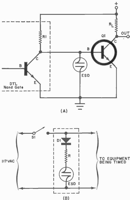
Fig. 5. Energy Storage Device (ESD) can have effective capacitance of up to 50 F! So new, special schematic symbol had to be evolved. In (A) is a time control circuit; (B), running time integrator.
