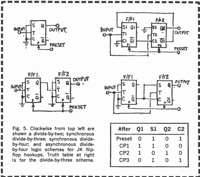
The JK flip-flop is not responsive to positive-going pulses or to steady-state signals of either polarity at the T input.
