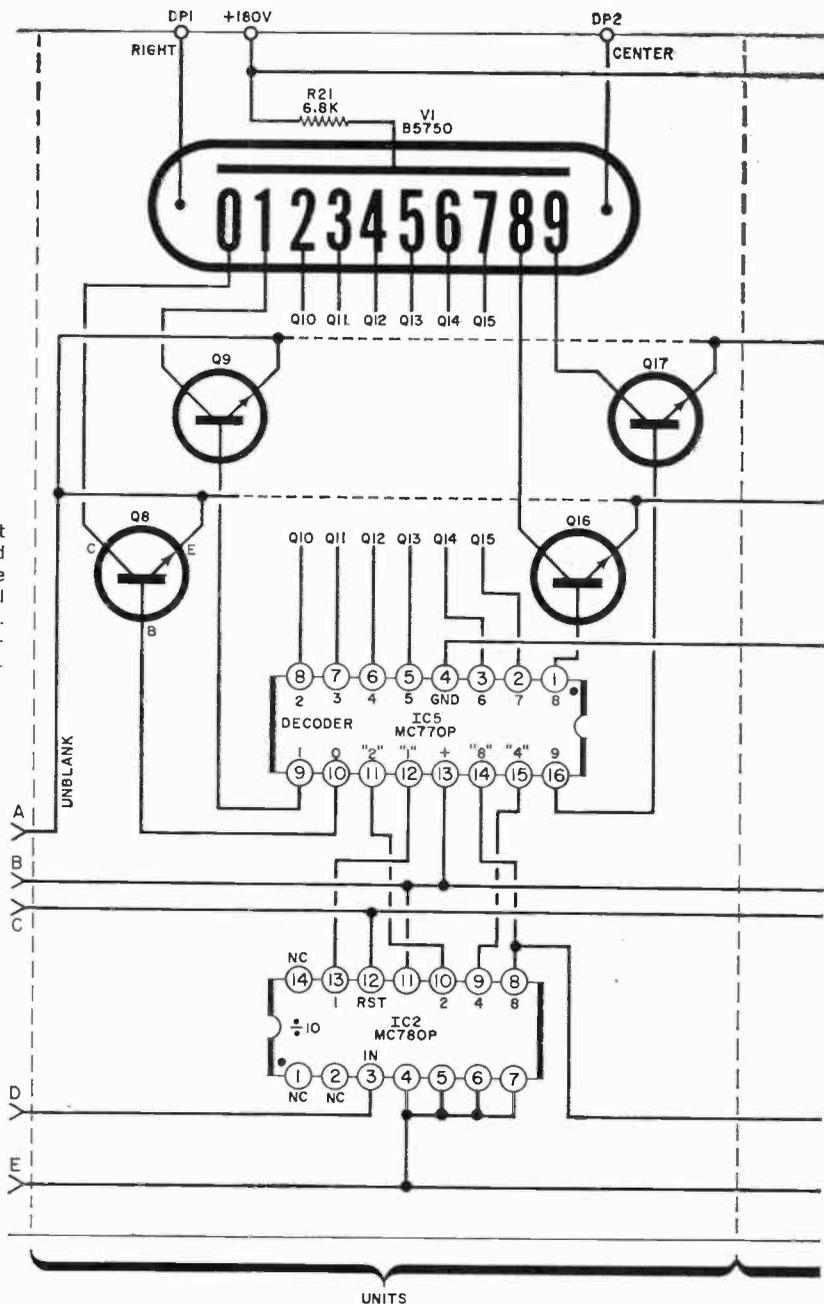
The second half of the circuit contains the units, tens, 1, and overrange indicators. Only the units decade is shown in detail as the tens decade is similar. The overrange indicator is connected to terminal marked "X".
