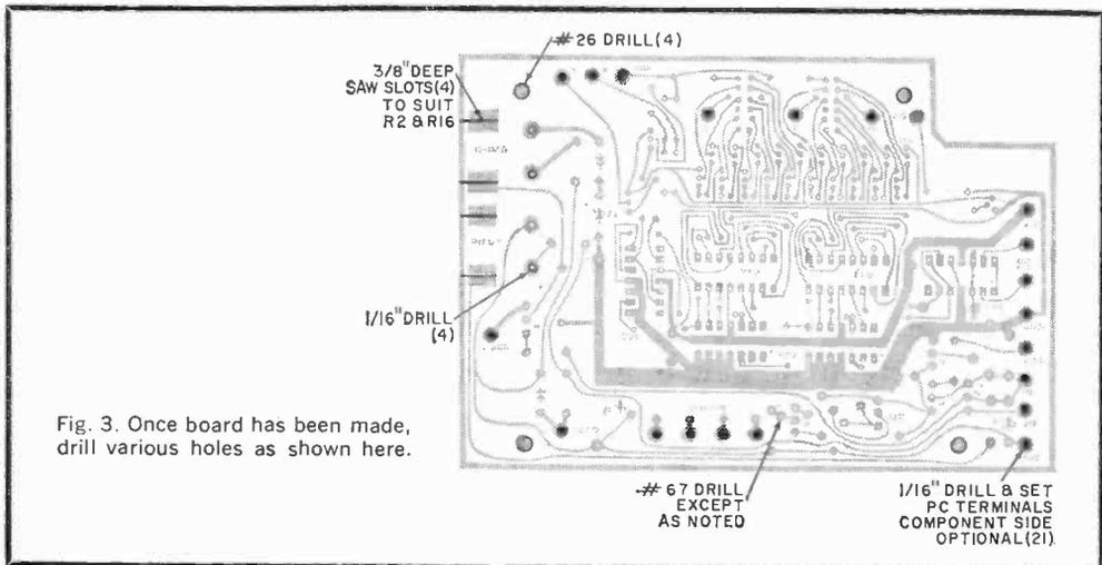
Fig. 3. Once board has been made, drill various holes as shown here.
