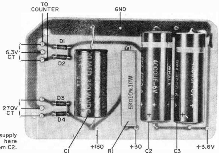
Fig. 8. Install the power supply components as shown here making sure *R1* is away from *C2*.
