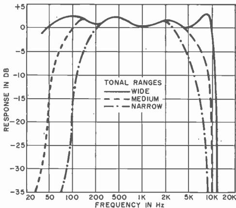
Frequency responses used in the Chinn and Eisenburg tests. Most people preferred the narrow band which rolled off at 3500 Hz. (See reference 1.)
