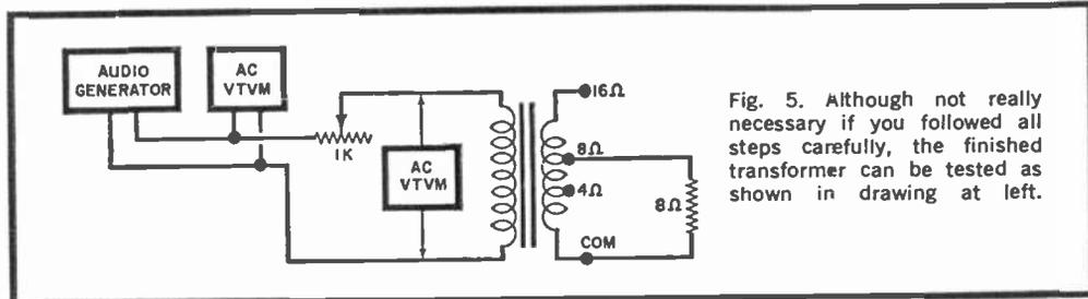
Fig. 5. Although not really necessary if you followed all steps carefully, the finished transformer can be tested as shown in drawing at left.
