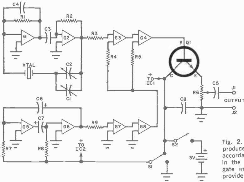
Fig. 2. Each gate is used to produce the output signal in accordance with the flow shown in the logic diagram. Unused gate inputs are grounded to provide good circuit stability.
