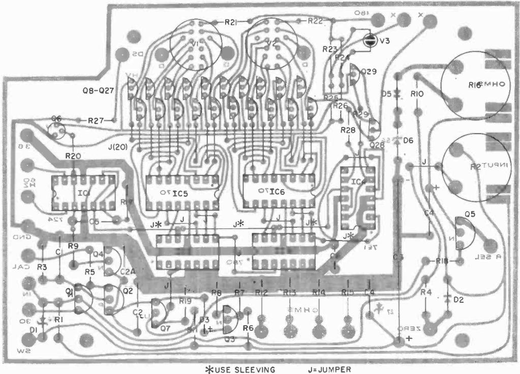
Fig. 4. Take your time when installing the components to make sure you insert the IC's and transistors properly. Certain jumpers are insulated to remove the possibility of shorts when all components are installed.
