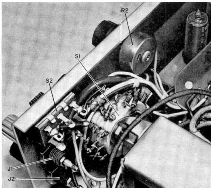
The various front-end resistors are wired point-to-point directly on the switch. This can be done before the switch is mounted, but be sure to double check the assembly before installation. Keep all wiring short and make sure no part shorts against the metal chassis.
