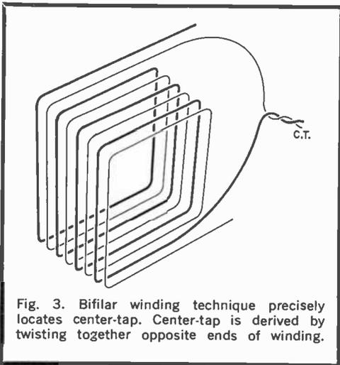
Fig. 3. Bifilar winding technique precisely locates center-tap. Center-tap is derived by twisting together opposite ends of winding.
