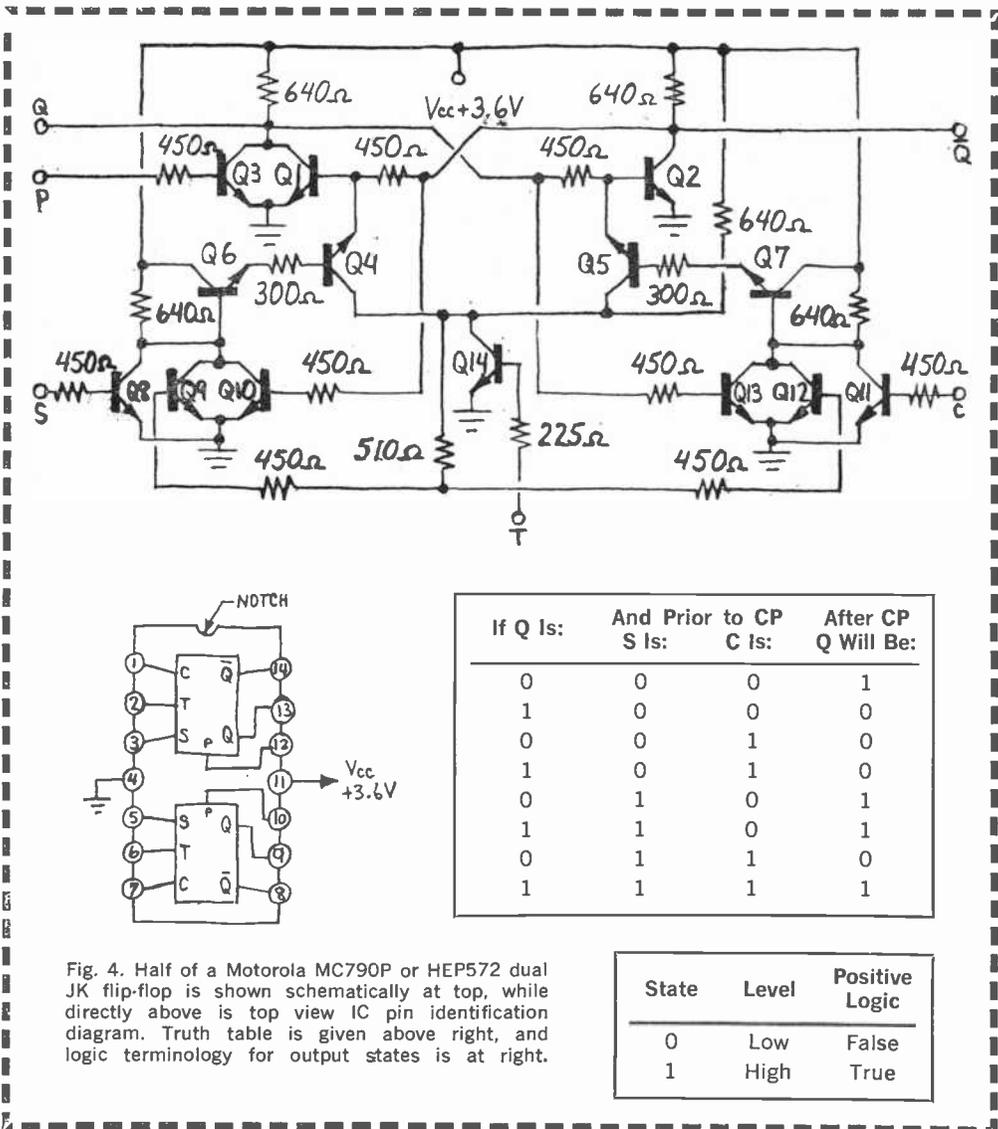
Fig. 4. Half of a Motorola MC790P or HEP572 dual JK flip-flop is shown schematically at top, while directly above is top view IC pin identification diagram. Truth table is given above right, and logic terminology for output states is at right.
