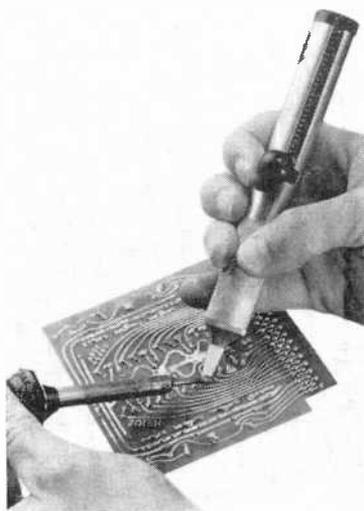
**TECHNI-TOOL DESOLDERING PUMP**—One-hand operation is the major claim for the imported *Techni-Tool Inc.* T-2 Desoldering Pump. Built in an aluminum housing, the T-2 can be primed using your thumb and released by your index finger. There is no external plunger so this hazard is removed from the lab bench. Teflon replaceable tips are available from the distributor. Cleaning of the T-2 is easy since it is easily disassembled into 3 separate parts.
