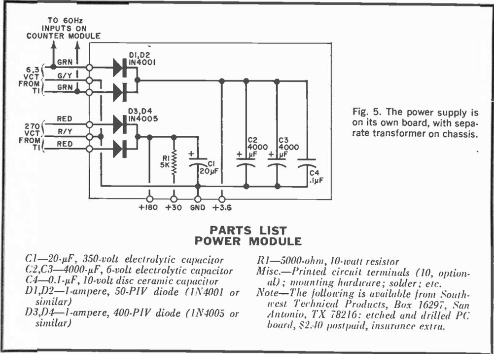
Fig. 5. The power supply is on its own board, with separate transformer on chassis.
