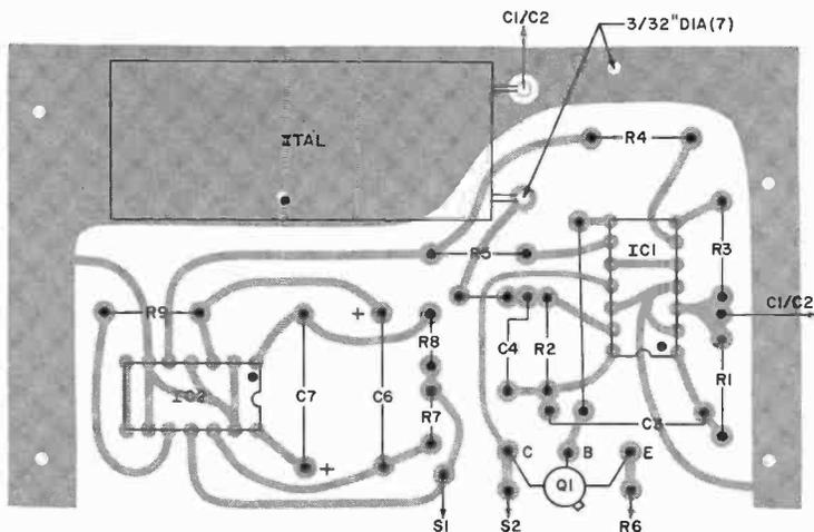
symmetrical cross-coupled astable multivibrator, using electrolytic capacitors *C6* and *C7*. Resistors *R7* and *R8* supply gate input bias. The output from *G6* is fed to *G7* through *R9*. The output of *G7* is directly coupled to output stage *G8*, the signal from which is fed to the buffer and driver in *IC1* through *R4* and *R5*. Resistor *R9* decouples the multivibrator, thereby helping to maintain the symmetry of the modulating signal.
