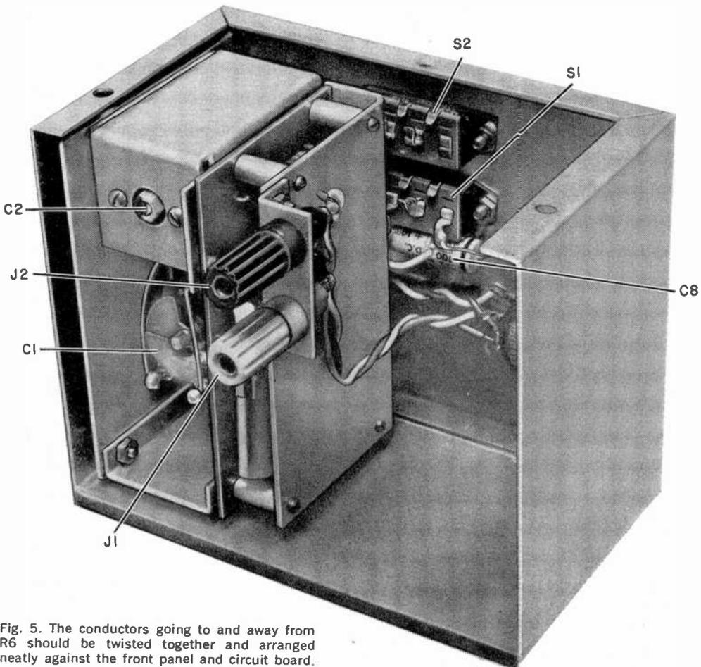
Fig. 5. The conductors going to and away from *R6* should be twisted together and arranged neatly against the front panel and circuit board.
