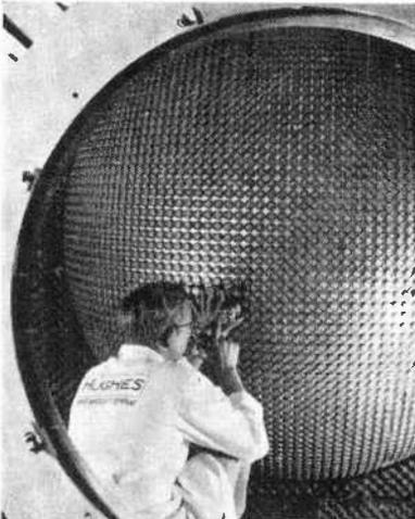
Hughes Aircraft ADAR receiving array consists of a microwave optical system with individual 2°-beamwidth horn feeds. Computer selects beam to track many targets.
