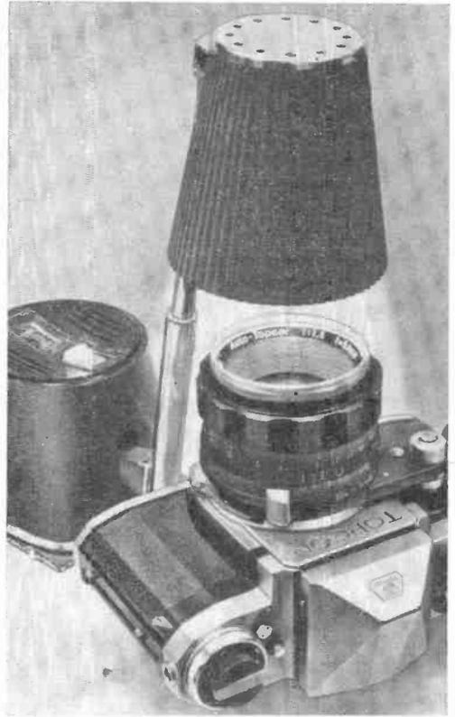
**Operation.** Before using the Shutter Speed Tester, always check the battery condition and then depress  $S2$  to zero the meter. Make sure the camera lens is wide open. To test the camera shutter speed, remove or open
