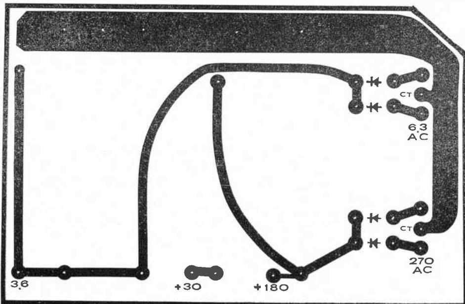
Fig. 6. Actual size foil pattern for the power supply.
