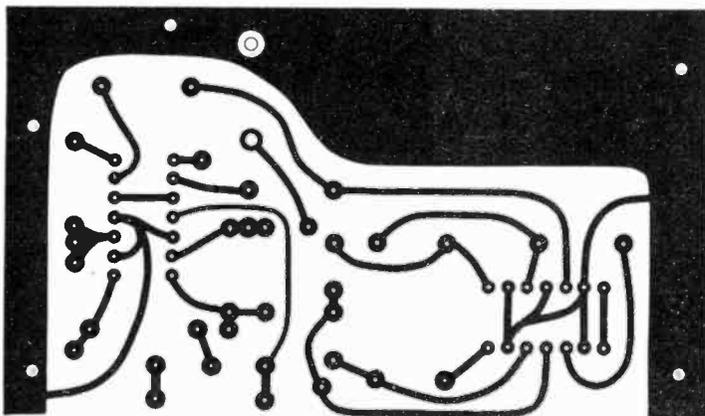
Actual size printed circuit board etching guide is shown above, while at right is component placement/orientation guide.
