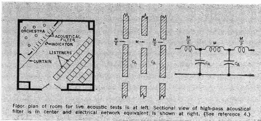
Floor plan of room for live acoustic tests is at left. Sectional view of high-pass acoustical filter is in center and electrical network equivalent is shown at right. (See reference 4.)
