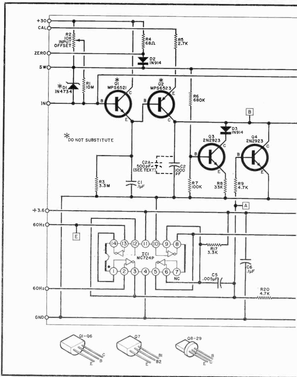
**Counter Module Construction.** The schematic of the counter module is shown in Fig. 1. A printed circuit board is essential for this module. You can purchase one as mentioned in the Parts List or you can make your own using the etching guide shown in Fig. 2 and the drilling instructions in Fig. 3.
