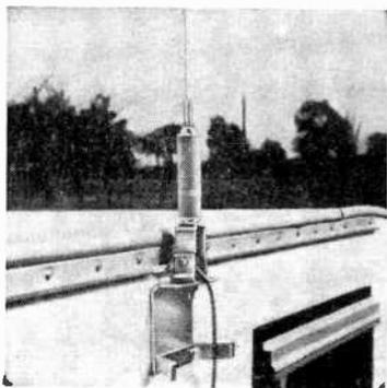
**ANTENNA SPECIALISTS MOBILE CB ANTENNA**—Outdoorsmen who use citizens two-way radio (CB) will welcome the new Model M-189 from *The Antenna Specialists Co.* It can be mounted on almost any level or slanted surface because of a special swivel base and full 90° vertical adjustment. Thus it is easy to install on campers, trailers, trucks, buses, etc. The antenna has a high-efficiency loading coil, is completely weatherproof, and has a tapered stainless steel whip.
