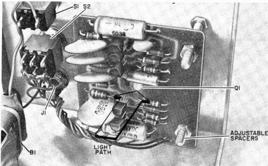
Like transmitter, assemble receiver board on four adjustable spacers so that the window of Q1 is at the focus of the lens. Once again, make sure batteries do not obstruct light.
