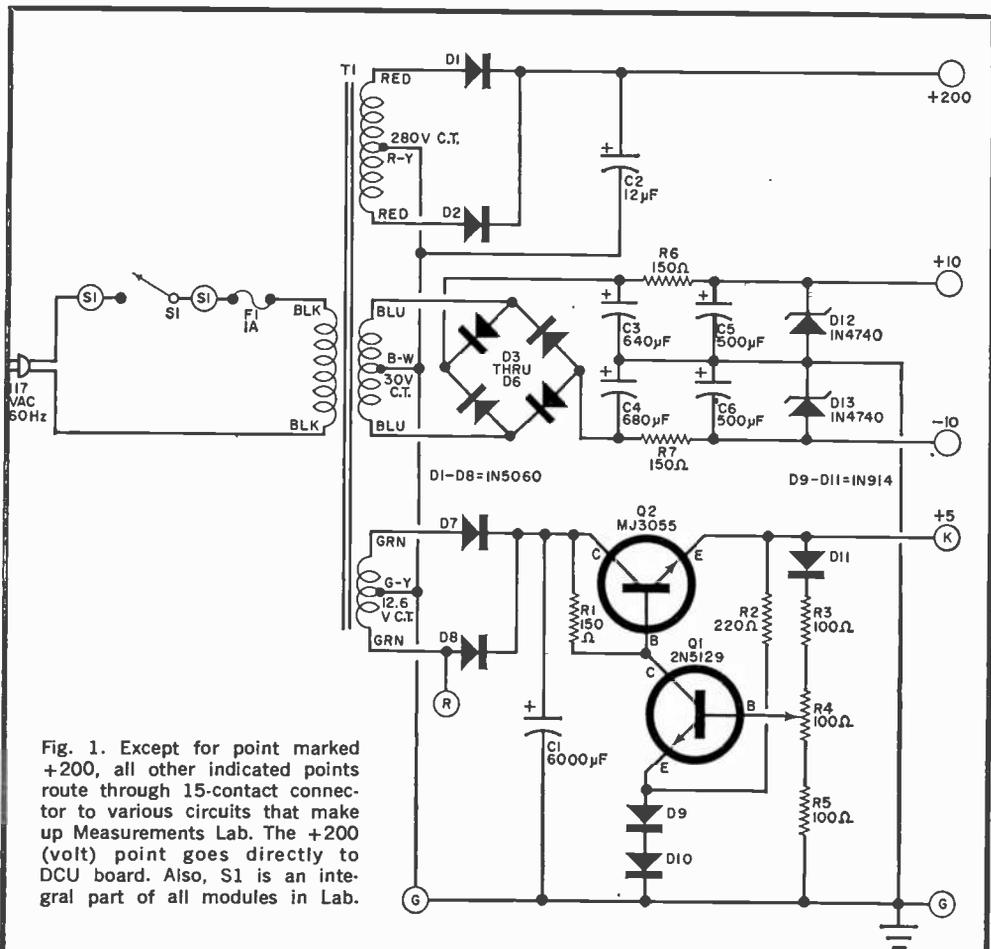
Fig. 1. Except for point marked +200, all other indicated points route through 15-contact connector to various circuits that make up Measurements Lab. The +200 (volt) point goes directly to DCU board. Also, S1 is an integral part of all modules in Lab.
