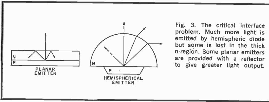
Fig. 3. The critical interface problem. Much more light is emitted by hemispheric diode but some is lost in the thick n-region. Some planar emitters are provided with a reflector to give greater light output.
