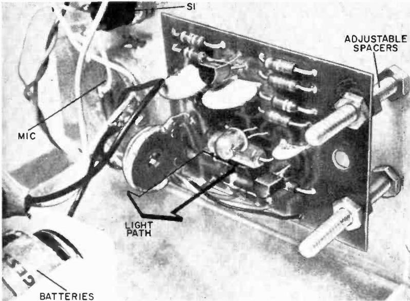
Assemble the transmitter on four adjustable spacers so that the window of the LED can be placed at the focal point of the lens. When assembling complete chassis be sure to mount the batteries so that they do not obstruct light path between the LED and the lens. Although the prototype has the microphone on chassis, a remote mike can be used. Even S2 can be mike-mounted push-to-talk switch. Oscillator switch S1 is rarely used, so can remain mounted on chassis.
