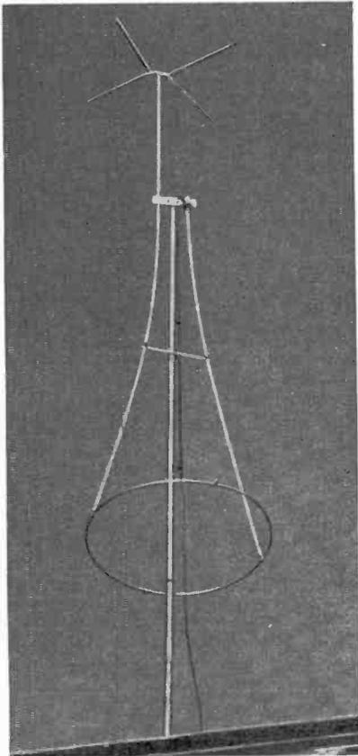
The Avanti Astro-Plane may be thought of as inverted colinear with short radials (top, above) and a trombone matching section below. Shortened top-loading radials are made of pre-bent seamless aluminum tubing. Liberal use of lock washers (see photo at right) practically eliminates the possibility of wind or ice loading bending the radials.
