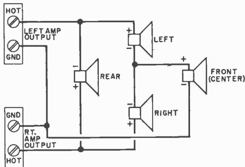
Fig. 3. Dynaco's recommended loudspeaker hook-up for Hafler four-channel playback. All speakers should be identical, and the two stereo channels should be modified to provide 6 dB of separation (unless a separate summing amplifier is used to drive the front center loudspeaker).
