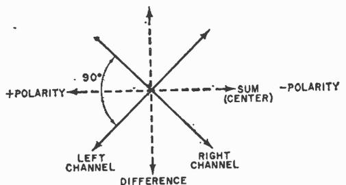
Fig. 1. Stylus motions in two-channel disc groove. Dotted arrows are resultants of left/right axes.
