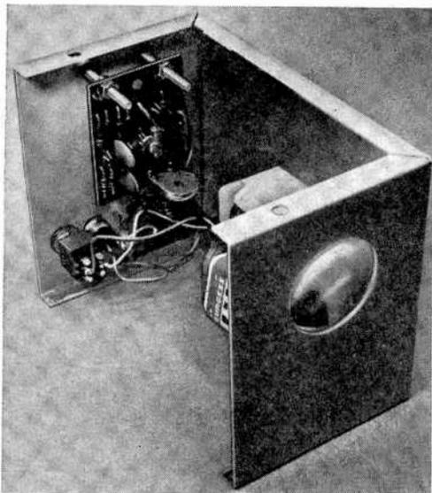
In assembling the transmitter, arrange the board and lens mounting so that the LED window is on the center line of the lens. The text explains how to adjust the board to make the lens focus at the window of the light-emitting diode on board.
