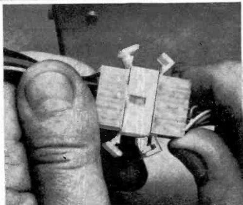
A 15-contact Molex connector is recommended for use in Digital Measurements Lab for positive electrical contact.
