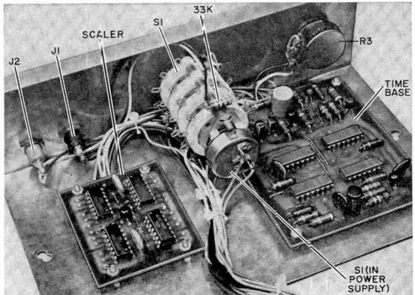
Fig. 10. Time Base and Scaler circuit boards fasten to chassis with 4-40 machine hardware and spacers. A 33,000-ohm resistor ( $\frac{1}{2}$ -watt) is used to limit current through decimal point in readouts. Wires connect to foil sides of boards.
