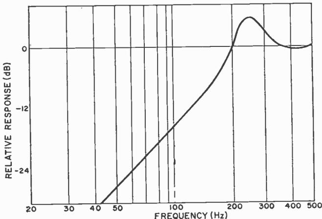
Generalized response curve of a cheap speaker in a sealed box has a resonance peak at 245 Hz. Amplitude of peak would depend upon speaker and enclosure properties.
