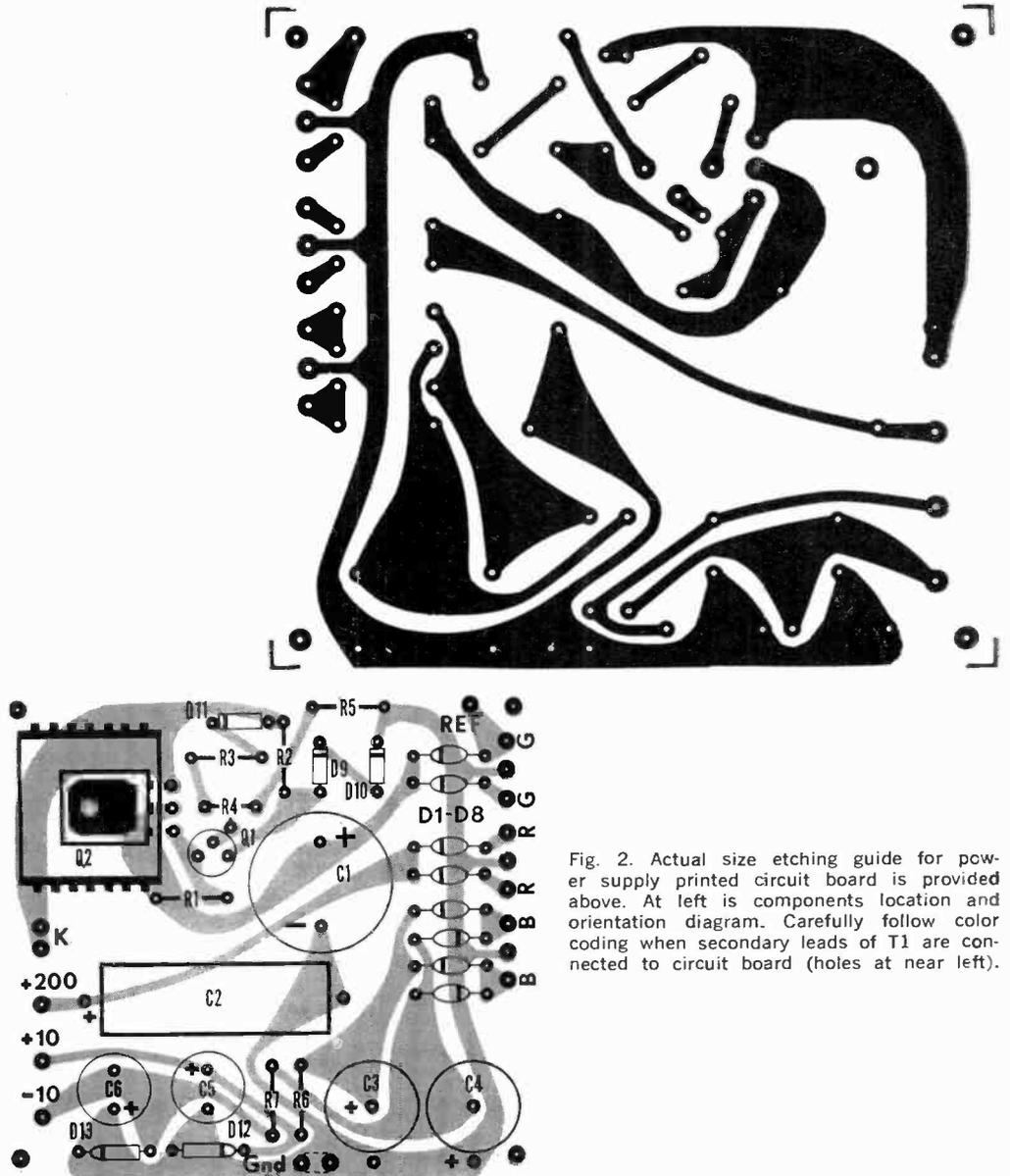
Fig. 2. Actual size etching guide for power supply printed circuit board is provided above. At left is components location and orientation diagram. Carefully follow color coding when secondary leads of T1 are connected to circuit board (holes at near left).
