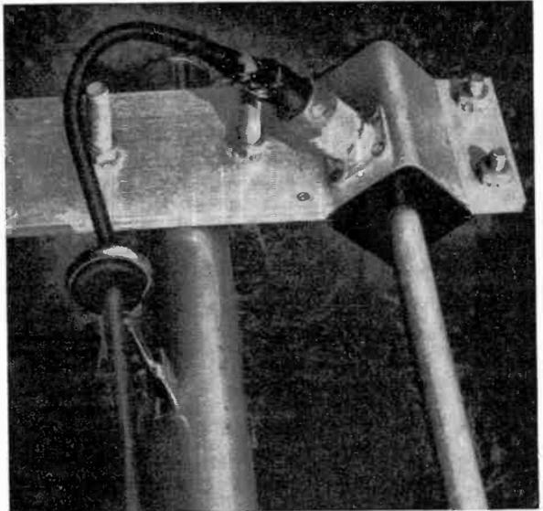
Don't forget to caulk coax cable plug when it is attached to the Astro-Plane input connector. The liberal use of caulking prohibits moisture from corroding the silver plating on the connector and keeps it from entering the coaxial cable.
