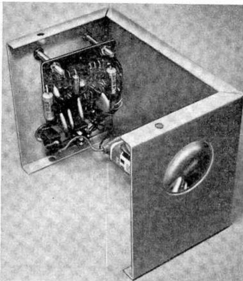
The receiver must be assembled in a manner similar to the transmitter—with the window of Q1 at the focal point of the lens. In both receiver and transmitter, once the focus has been attained, a drop of cement on screws will prevent slippage.
