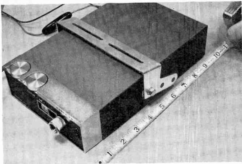
The Cobra 24 is one of the slightly deeper mobile CB transceivers. This may present a mounting problem in some automobiles. To be on safe side, allow a minimum of 12" (including the coax cable connector) if you don't want a transceiver that projects too far out from under the dashboard of your car.
