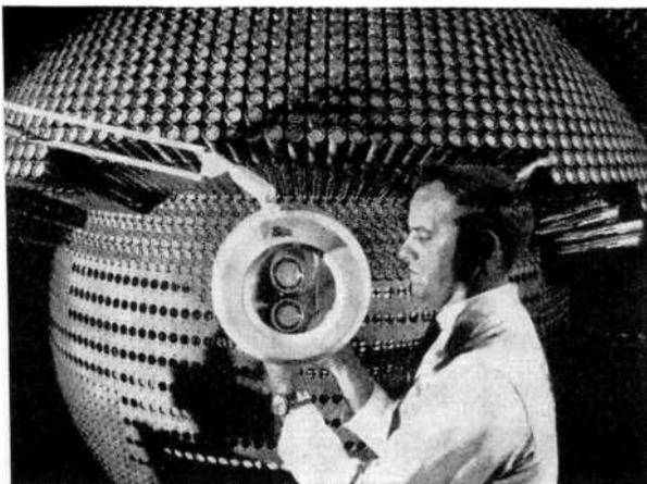
tion of the beam is broadside to the face of the array. By introducing a different phase displacement in the current delivered to each antenna, however, the beam can be moved almost instantaneously from one position to another.
