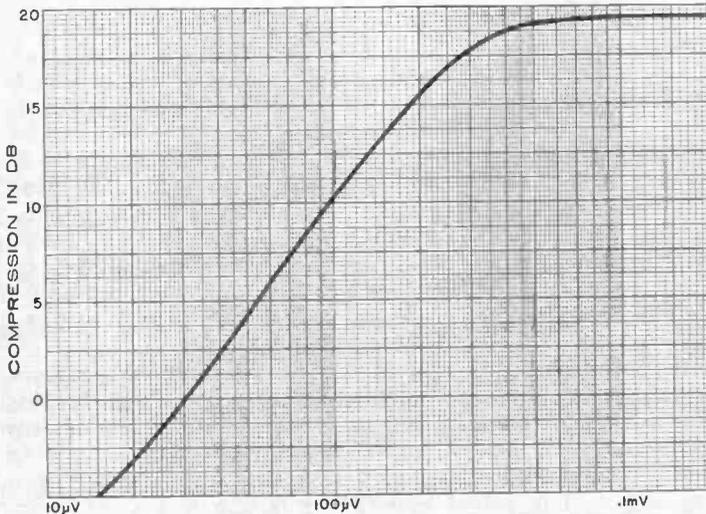
Input versus compression showing the smooth curve of an excellent nondistortion setup.
