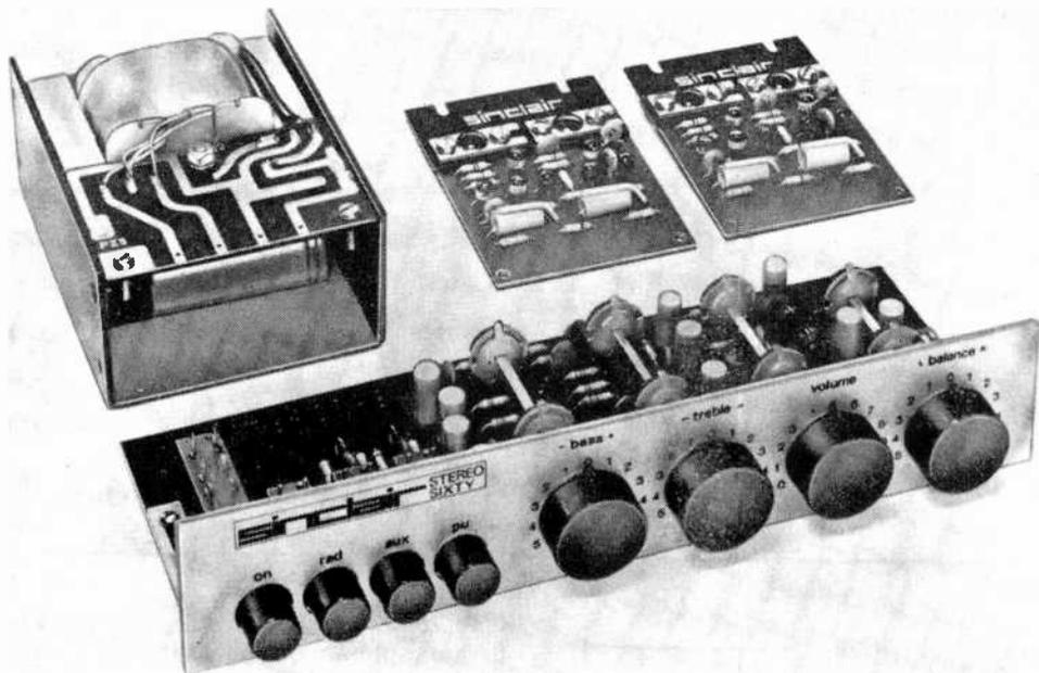
To complement the Z-30, Audionics also has made available a suitable power supply, and a preamplifier/control unit that includes all the necessary tone and balance controls, with pushbuttons for selecting the various inputs. As shown above, this combination is called the "Stereo 60." In addition, there are also available a high- and low-pass active filter unit for scratch and rumble attenuation, a 50-watt amplifier module similar to the Z-30 unit, and a new IC having an output of 6 watts
