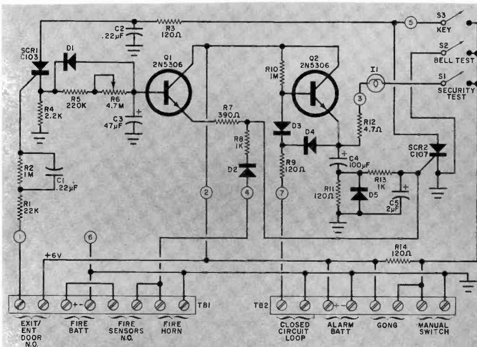
Fig. 1. Unlike other alarms, this one features a 5- to 50-second delay to allow legitimate entry without ringing the gong. This same circuit is also used for fire warning when used with the appropriate sensors.
