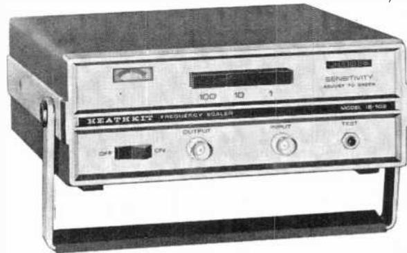
usual Heath standards. It is all solid-state, with eight IC's and seven transistors (including one FET), and it has an excellent built-in regulated power supply. It has the same dimensions as the IB-101 counter—8¼" wide, 9" deep, and 3⅝" high. It weighs seven pounds and fits nicely on top of (or under) the counter.
