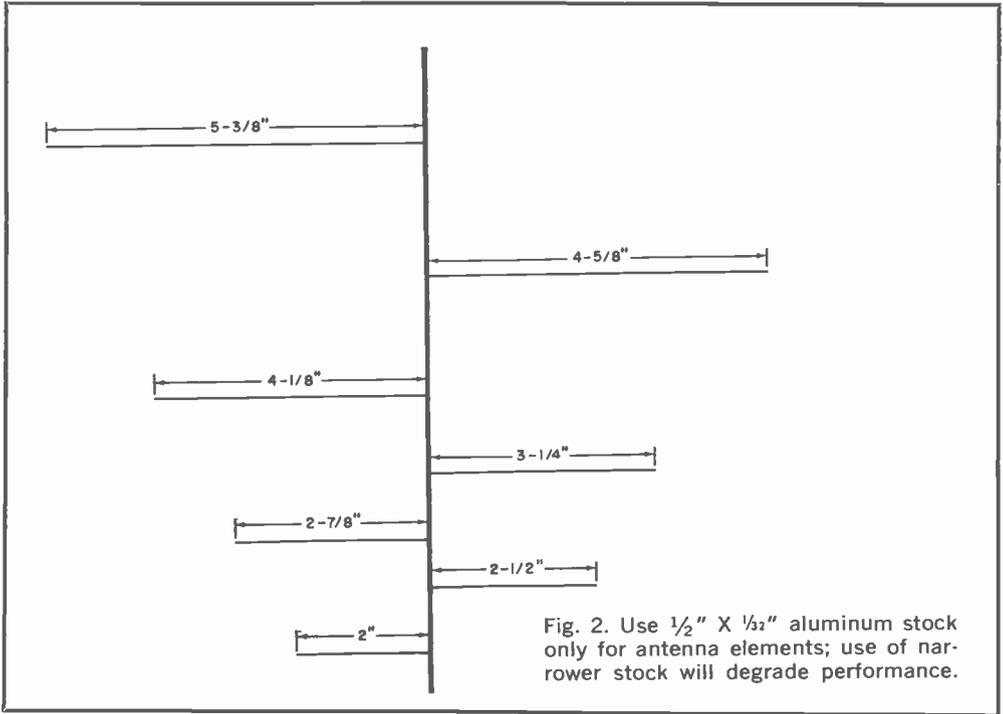
Fig. 2. Use 1/2" X 1/2" aluminum stock only for antenna elements; use of narrower stock will degrade performance.
