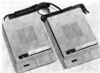
**AUDIOTEX WIRELESS INTERCOMS**—Designed for 117-volt ac operation GC Electronics' new Audiotex wireless intercom No. 30-6024 requires no special cables or wires. The ac line not only supplies the operating power for the intercoms, but it also acts as the transmitting and receiving cable. The intercom operates on a carrier current frequency of 140 kHz. Each intercom features a lock button for continuous operation when used for baby-sitting, surveillance, etc. Price is \$49.95 per pair.
