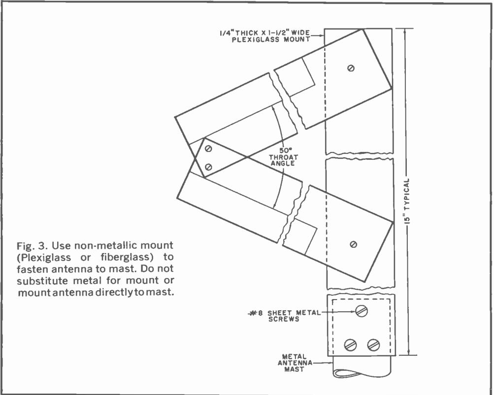
Fig. 3. Use non-metallic mount (Plexiglass or fiberglass) to fasten antenna to mast. Do not substitute metal for mount or mount antenna directly to mast.
