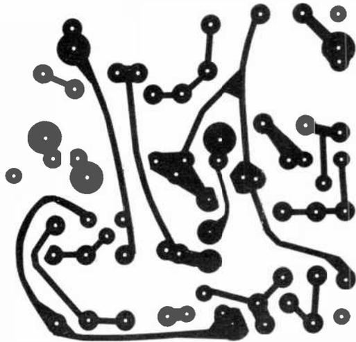
R1 and R12 are mounted vertically with their top terminals serving as terminals 1 and 3 respectively. Terminals 2 and 4 through 7 on the board are made from L-shaped pieces of stiff copper wire inserted in the appropriate holes and soldered to the foil on the bottom.
