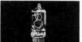
Designed as direct line, side-view readout devices for basic counter and computer circuits. Gas filled cold-cathode numerical indicator tubes use common anode, 10 cathodes in shapes of numerals 0-9. Also give visual digital display of volts, cycles, etc. High reliability, long life; wide-angle viewing with brightness and stability.
