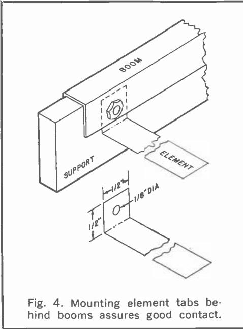
Fig. 4. Mounting element tabs behind booms assures good contact.
