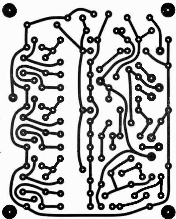
Fig. 3. Actual size foil pattern and component layout. Take care when installing semiconductors, diodes, etc. See text before installing Q7 and Q8.
