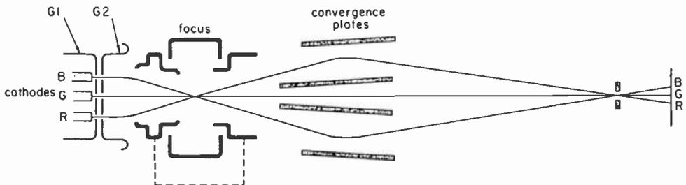
the same ones that let two green beam-segments through—pass only enough red beam to illuminate two red stripes of phosphor. The angle of the red beam just suits the positioning of the red stripes with respect to the grille openings, and the red beam does not touch green or blue stripes.
