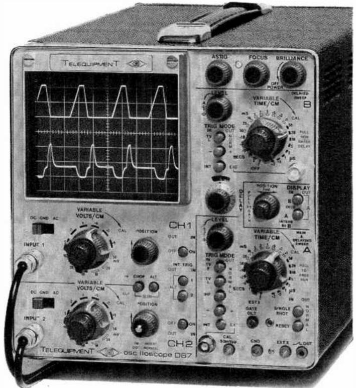
resolution analysis of pulse sequences. And if some of the pulses are jittery, that won't be a problem because the delayed sweep can be triggered. Those who have a need to view television signals will be pleased with the D67's ability to trigger at TV field and line rates.
