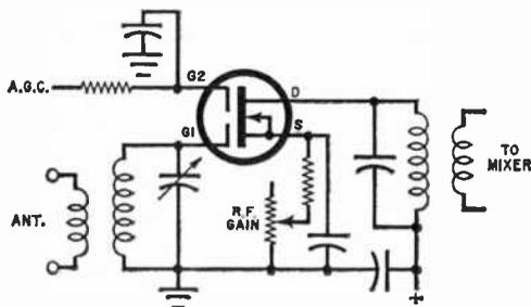
Fig. 3. Here, the dual-gate MOSFET r-f stage has its gain controlled by a negative voltage which shown is applied to gate 2.
