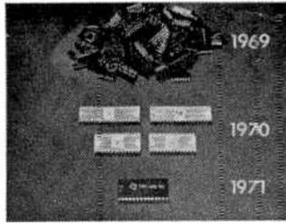
This succession of devices portrays the evolution of active components necessary for implementation of an 8-digit calculator. In 1969 the effort required dozens of bipolar devices. By 1970 the same calculator could be produced using only four MOS/LSI devices, and now it has been implemented on a single MOS/LSI chip.
