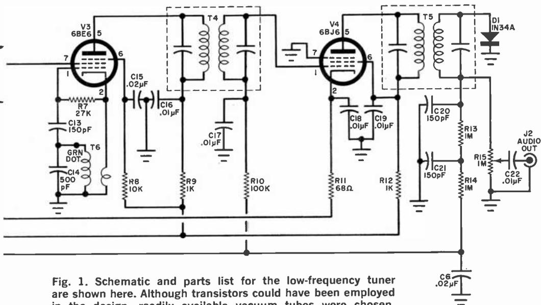
Fig. 1. Schematic and parts list for the low-frequency tuner are shown here. Although transistors could have been employed in the design, readily available vacuum tubes were chosen. Note that two r-f stages (V1 and V2) were used in design because the low power of the transmitter requires a very sensitive tuner. The converter stage is V3, and V4 is the amplifier.
