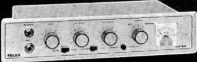
Matching electronics for above. RP 84, professional solid state, monaural record and playback preamplifier for tape transports with two or three heads. Selectable equalization from 1-7/8 to 15 ips. A-B monitor switch. Mixing of line and mike inputs. Bias synch provision for multi-channel applications. Phone jack, VU meter, record light. 30-18,000 Hz  $\pm$  3dB at 7.5 ips. Also model PB-10 playback preamplifier and model PA94F, 8 watt playback amplifier.
