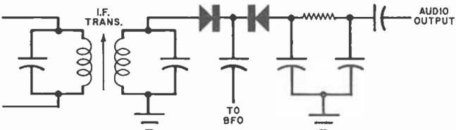
Fig. 11. This simple product detector for CW and SSB applications uses a back-to-back dual diode arrangement.
