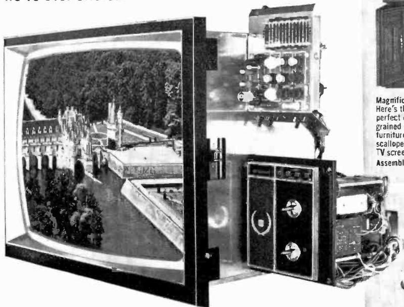
The new Heathkit GR-900 25V Color TV has UHF/VHF detent tuning & varactor UHF tuner, angular tint control — more features than any other color TV kit! Better performance than any other set.
