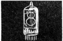
Designed as direct line, side-view read-out devices for basic control and computer circuits. Gas filled cold-cathode numerical readout tubes use common anode, 10 cathodes in shapes of numerals 0-9. Also give visual digital display of volts, cycles, etc. High reliability, long life, wide-angle viewing with brightness and stability.
