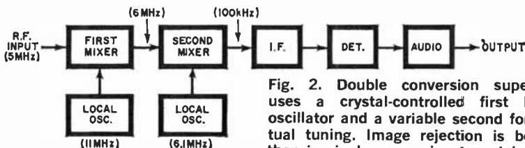
Fig. 2. Double conversion superhet uses a crystal-controlled first local oscillator and a variable second for actual tuning. Image rejection is better than in single-conversion type (above).
