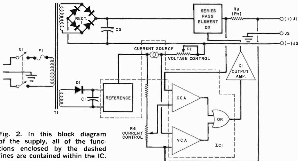
Fig. 2. In this block diagram of the supply, all of the functions enclosed by the dashed lines are contained within the IC.
