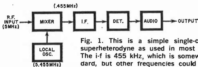
Fig. 1. This is a simple single-conversion superheterodyne as used in most receivers. The i-f is 455 kHz, which is somewhat standard, but other frequencies could be used.
