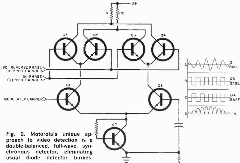
Fig. 2. Motorola's unique approach to video detection is a double-balanced, full-wave, synchronous detector, eliminating usual diode detector birdies.
