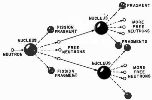
**Nuclear fission occurs when a high-speed neutron splits nucleus of uranium or plutonium. Tremendous energy is released and other neutrons are knocked loose. If released energy is sufficient, chain reaction can occur.**
