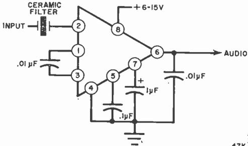
Fig. 9. This IC i-f stage provides 0.8 volt output from an input as low as 50 microvolts. The circuit also has agc range of 60 decibels.
