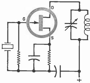
Fig. 7. Typical crystal-controlled oscillator using a junction FET. The tuned circuit in the drain is set to the crystal frequency. For a different frequency, both crystal and the tuned circuit components must be changed.
