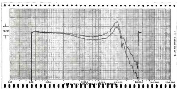
You have chosen a highly-rated, very popular cartridge. But to get flat response at home, you'll have to add a capacitor to each input, or measured lengths of cable of specific capacity. This will "kill" the peak you see here, but the Hi-Q mechanical resonance that caused it will remain. It won't sound bad, but it could be better!
