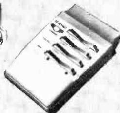
**Wireless Remote for your GR-900.** The ultimate in armchair viewing. Gives you eight function across-the-room control of on/off, three preset volume levels, power tuning (up or down), color, tint, UHF/VHF channel selection. Also activates Custom Wall Mount doors. Kit GRA-900-6, 6 lbs. .... 79.95\*
