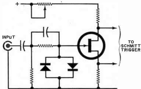
Input sensitivity is controlled automatically by this circuit in Weston counter.
