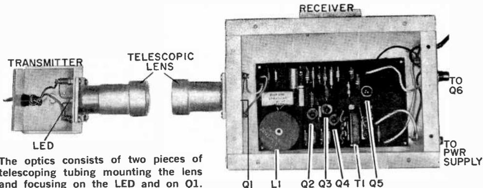
The optics consists of two pieces of telescoping tubing mounting the lens and focusing on the LED and on Q1.
