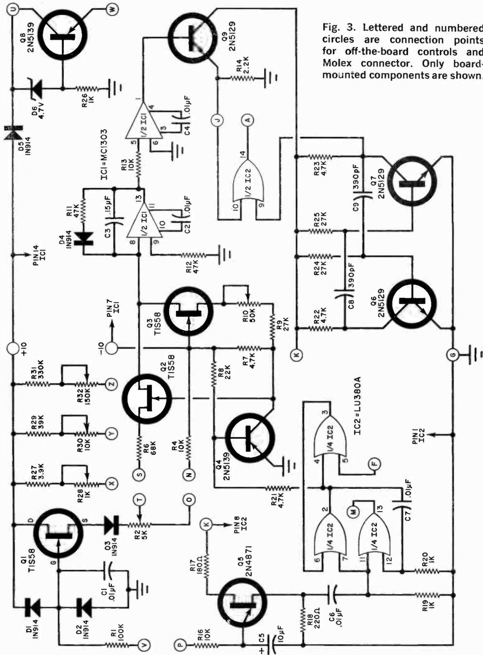
Fig. 3. Lettered and numbered circles are connection points for off-the-board controls and Molex connector. Only board-mounted components are shown.
