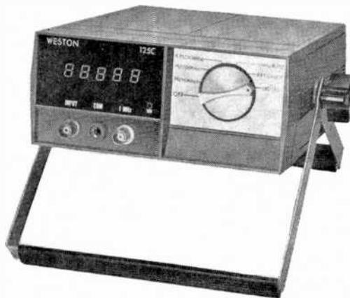
(which is very good). There is automatic blanking of the zeroes to the left of the actual displayed value to simplify reading. The input impedance of the frequency counter is 1 megohm, shunted by 30 pF. Sensitivity is 250 mV, while the maximum input level should not exceed 50 volts ac or dc. The input circuit has an automatic trigger level configuration that eliminates the need for a manually operated sensitivity control. Operating power can be taken from any 117-230-volt, 50-400-Hz ac line.
