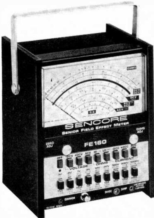
cause the transistors and diodes in a circuit to conduct and produce false indications. The high-power function allows the ohmmeter to be used in the same manner any other ohmmeter is used.
