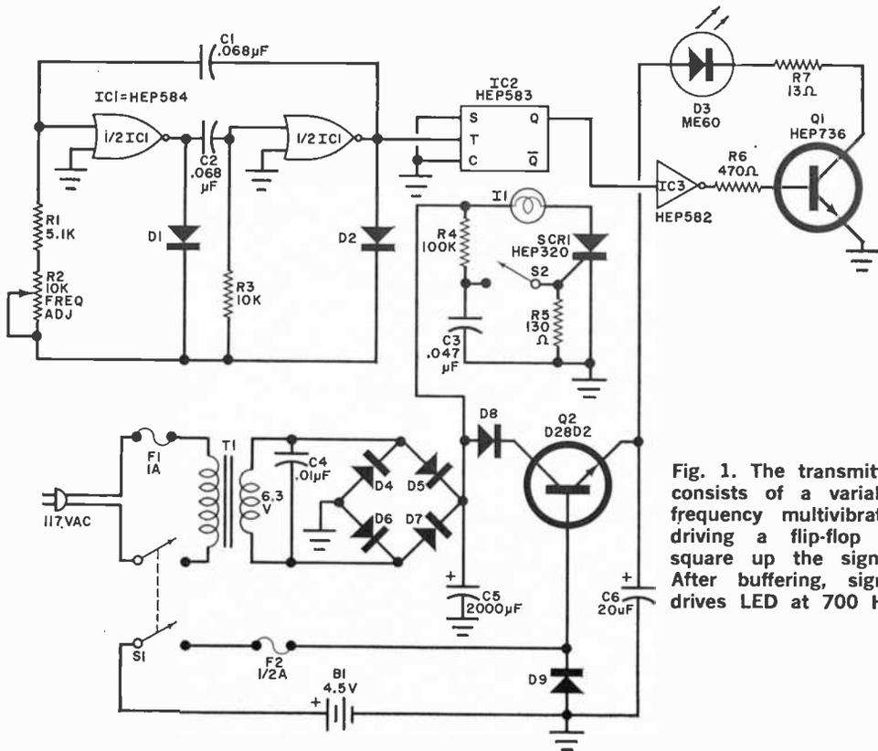
Fig. 1. The transmitter consists of a variable frequency multivibrator driving a flip-flop to square up the signal. After buffering, signal drives LED at 700 Hz.
