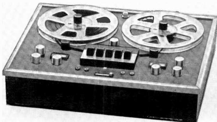
frequency response to beyond 12,000 Hz, which is adequate for taping almost all disc records and FM broadcasts. These two speeds are offered on virtually all home tape recorders, frequently in conjunction with a 1½-ips speed. Vocal material and background music can be recorded with adequate fidelity at 1½ ips, but the upper frequency limit is usually between 6000 Hz and 10,000 Hz.
