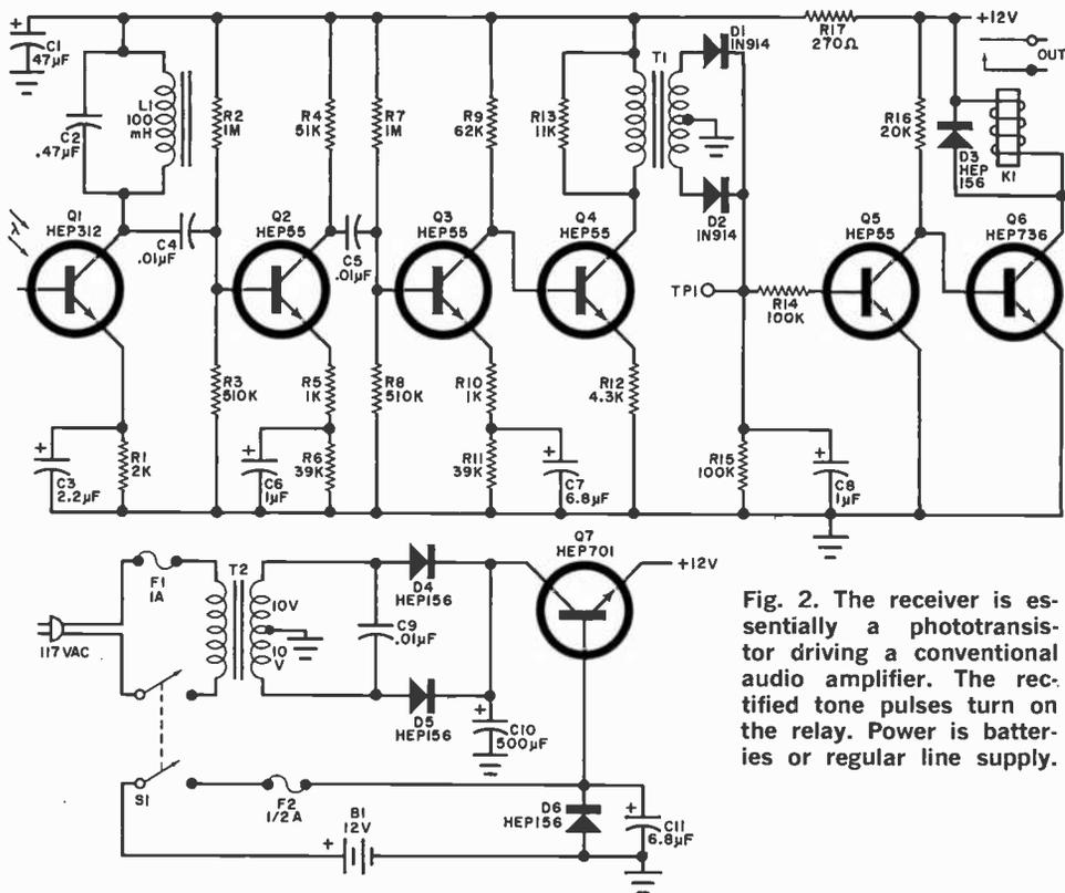
Fig. 2. The receiver is essentially a phototransistor driving a conventional audio amplifier. The rectified tone pulses turn on the relay. Power is batteries or regular line supply.
