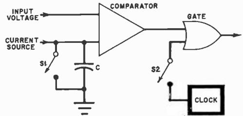
Fig. 1. Elementary capacitor-discharge analog-to-digital converter is typical of those used in digital instruments.
