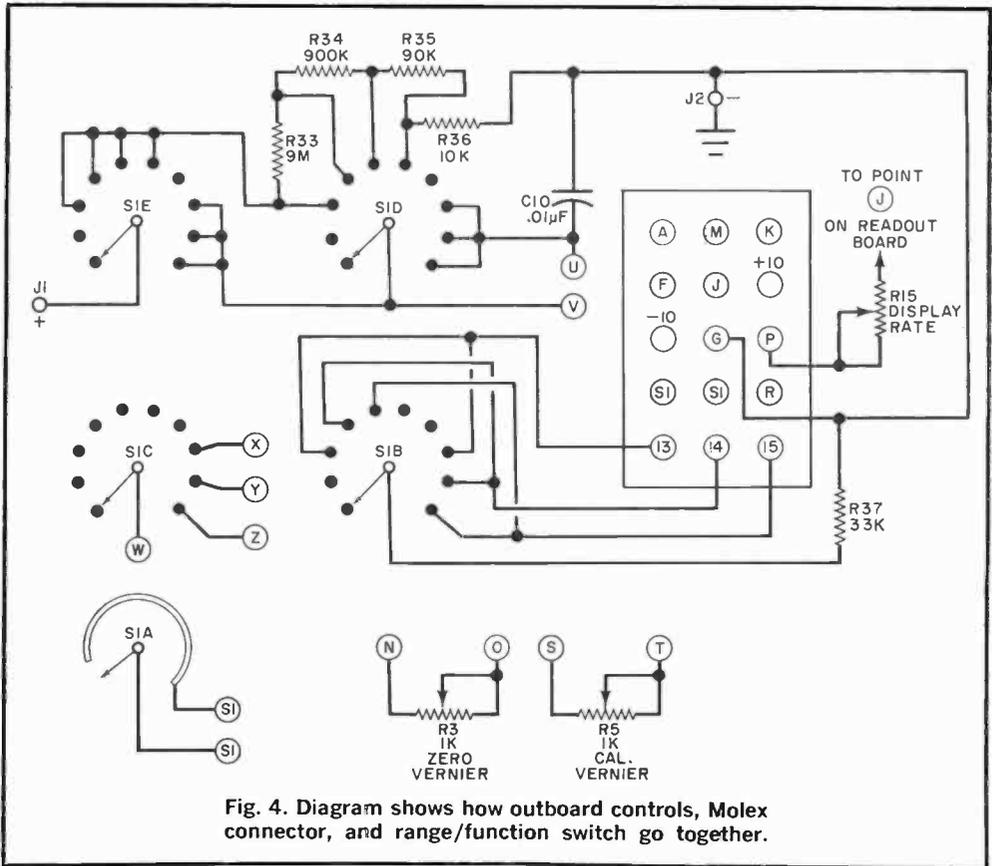
Fig. 4. Diagram shows how outboard controls, Molex connector, and range/function switch go together.
