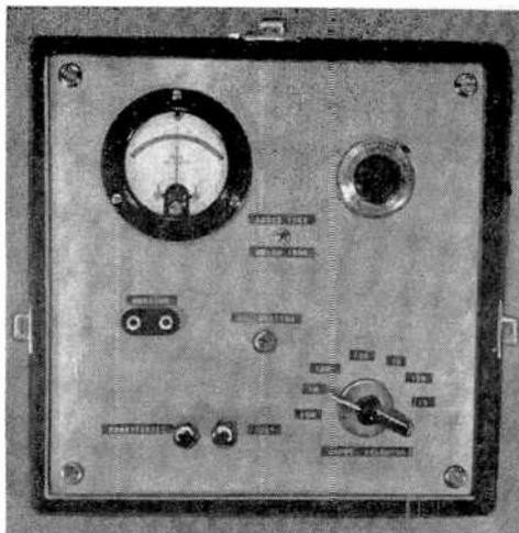
**Although the prototype was built in a wood case, any type of construction may be used. Note the 10-turn dial.**
