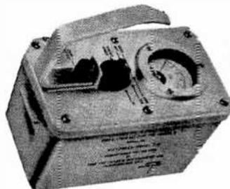
You can buy a complete radiation meter, complete with original instruction books, at less than the price of the meter movement alone. Range is 0.02 to 50 Roentgens/hour. This is not sensitive enough for prospecting, but useful for other radiation measuring and monitoring purposes. If not used for its original function, then the case,
