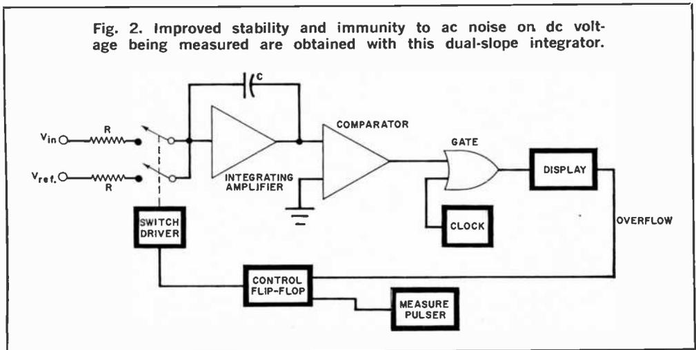
Fig. 2. Improved stability and immunity to ac noise on dc voltage being measured are obtained with this dual-slope integrator.
