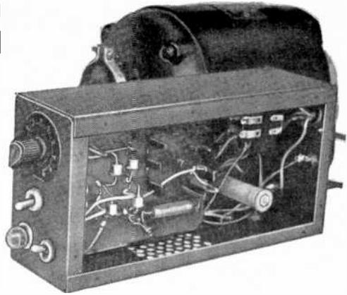
**E**LECTRONIC speed controls for ac motors usually use an SCR or Triac in conjunction with a phase-shifting network. However, for a dc motor, another approach must be used. The circuit schematic in Fig. 1 is for a speed control that has been successfully used for some time with a ½-hp dc shunt motor on a metalworking lathe that requires frequent starts and stops and imposes a wide range of loads, including over-
