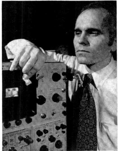
**That tiny sensor has only a  $\frac{1}{4}$ -square inch sensitive surface and is capable of producing the photograph as shown here on the scope screen. The sensor has 1408 sensitive elements.**
