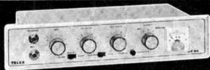
Matching electronics for above. RP 84, professional solid state, monaural record and playback preamplifier for tape transports with two or three heads. Selectable equalization from 1-7/8 to 15 ips. A-B monitor switch. Mixing of line and mike inputs. Bias synch provision for multi-channel applications. Phone jack, VU meter, record light. 30-18,000 Hz  $\pm$  3dB at 7.5 ips. Also model PB-10 playback preamplifier and model PA94F, 8 watt playback amplifier.
