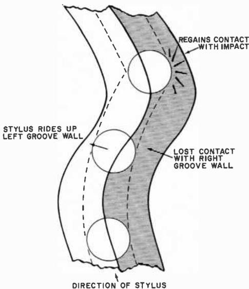
When stylus loses contact with one wall and rides up other, it returns to the first with a noisy impact sound.
