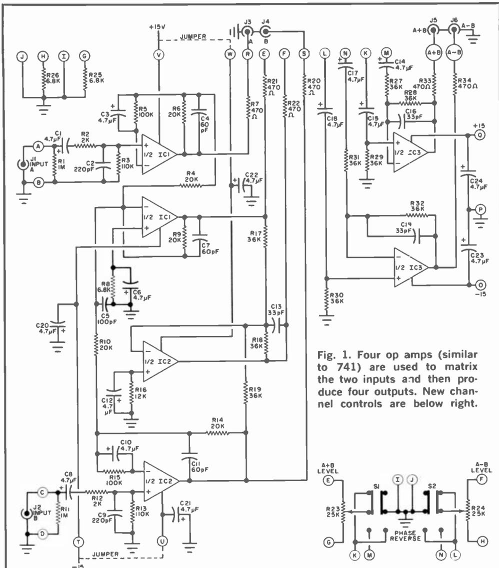
Fig. 1. Four op amps (similar to 741) are used to matrix the two inputs and then produce four outputs. New channel controls are below right.
