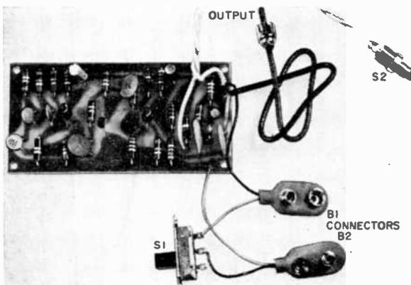
R9 and applied to the common emitter gain stage, Q3. When pushbutton S2 is open, Q3 cannot pass audio because its emitter is held at a slightly higher voltage than its base by the voltage divider R14 and R13. When S2 is closed, the voltage at Q3's emitter begins to drop as C9 discharges through R16.
