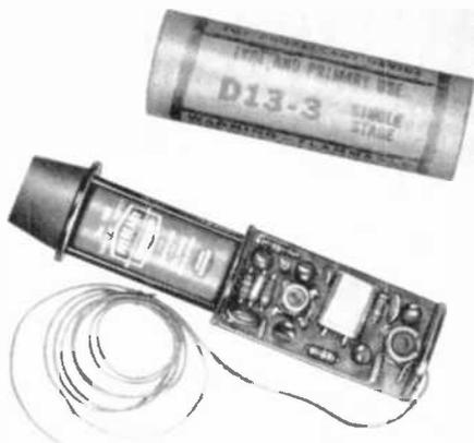
**R**ECENTLY, we had the opportunity to build and test the "Transroc" model aircraft and rocket transmitter put out by Estes Industries. Since it was designed to be used in conjunction with a conventional Citizens Band receiver, we were surprised at the compact size of the six-transistor, crystal-controlled transmitter.
