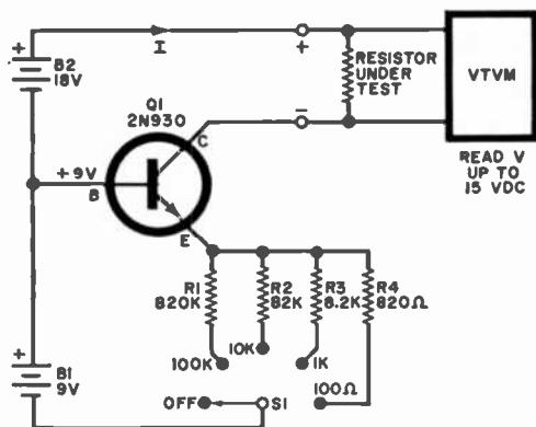
Test resistance value is equal to voltage drop across resistor times range multiplier of current source.
