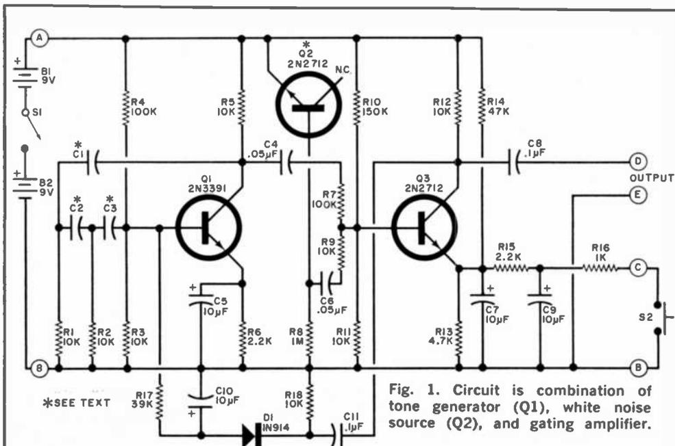
Fig. 1. Circuit is combination of tone generator (Q1), white noise source (Q2), and gating amplifier.
