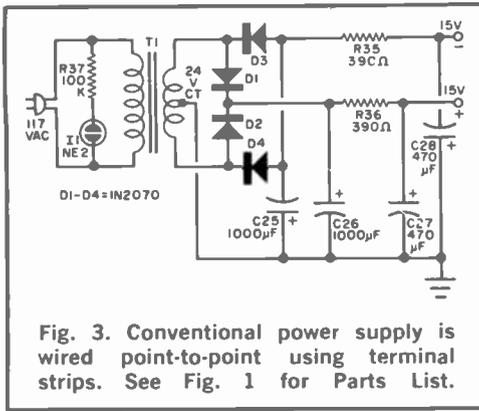
Fig. 3. Conventional power supply is wired point-to-point using terminal strips. See Fig. 1 for Parts List.
