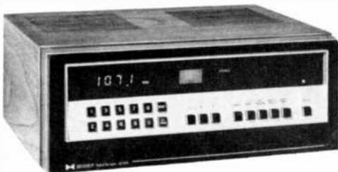
a master board. Tuning frequency, derived from a digital frequency synthesizer employing phase-locked loop techniques to achieve tuning accuracies of better than 0.005%, is displayed
