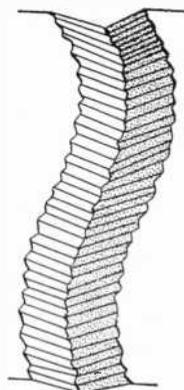
**Fig. 1. Audio signal (large undulation) and ultrasonic carrier (small undulations) in a single disc groove.**
