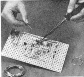
You learn how to construct circuits and connect them with a soldering iron, which is part of your CIE laboratory equipment. This "hands on" experience is extremely valuable in applying what you learn.
