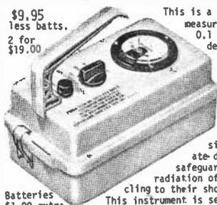
This is a monitoring instrument for measuring gamma radiation (from 0.1 to 50 roentgens/hr. Also designed to detect radioactive contamination levels caused by nuclear accidents, its sensitivity to ultra-minute electrical currents should make this a valuable tool in the experimental sciences. The Atomic Energy Commission requires far more elaborate detection instruments to safeguard workers from plutonium radiation of these gamma rays—particles
