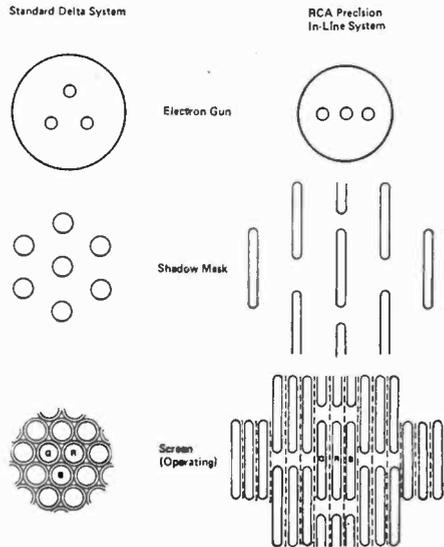
**New tube and in-line gun (left) has all deflection and convergence elements bonded to neck. It is smaller, lighter, and easier to set up than conventional tube (right).**
