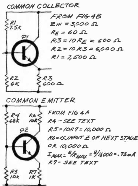
this time,  $R_6$  would be considered in regard to the desired voltage gain. A quick check shows that the 10,000-ohm value provides a gain of over 20.
