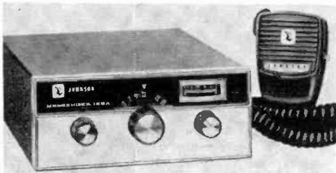
is an "acoustically isolated" speaker and special audio circuitry which has a frequency-tailored response for clearer voice reproduction and suppression of noise. An accessory external speaker is also available for use under exceptionally noisy conditions. Other accessories available include a power pack with rechargeable batteries for portable operation and a power supply base for desk-top use on 117-volt ac power.
