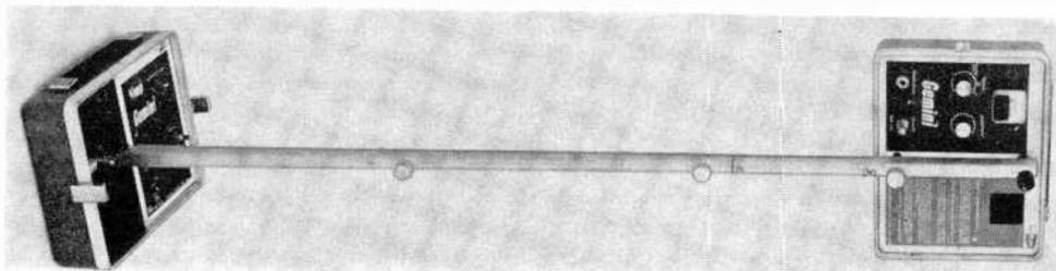
conditions. The output frequency is 82 kHz  $\pm$  5 kHz. Power to both the transmitter and receiver is furnished by conventional 9-volt batteries.
