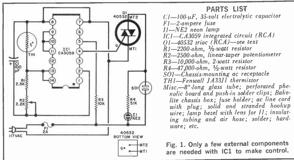
ing Q1 into conduction and shut off the heater. As long as the water temperature remains constant at the preset level, the system will remain passive. However, if the water temperature should fall below the preset level, TH1 will sense the event and initiate the process for resuming triggering Q1 and turning on the heater.
