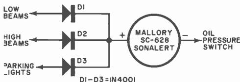
will be alerted to turn off parking and headlights whenever you turn off the engine without first switching off the lights.
