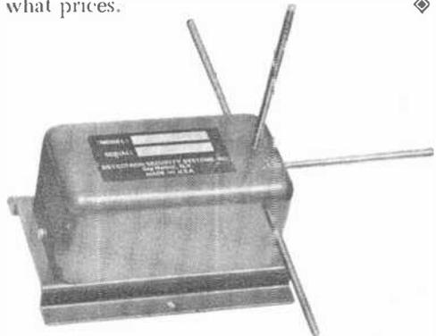
**Detecron unit has antenna on case.**
