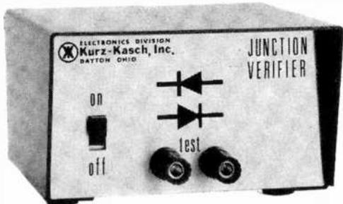
we were dealing with an npn type transistor that requires a positive voltage on the collector. If both displays had flashed simultaneously, I would know the junction was shorted. Had neither arrow flashed, I could be sure the junction was open. In either case, the transistor would be bad. So you see the verifier serves as a transistor tester and a transistor-type identifier."
