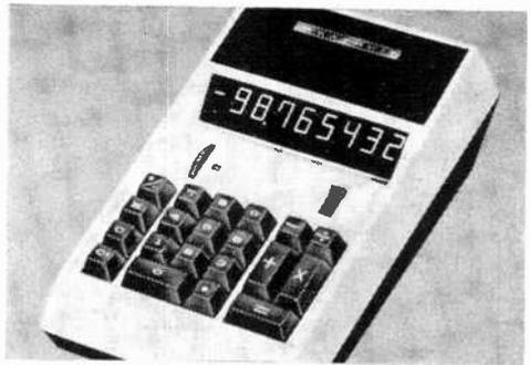
The overall range of the calculator is from 0.0000001 to 99999999. If the instrument's capability is exceeded—either during entry or during totalling—the keyboard automatically locks out, and the extreme left readout displays an E.
