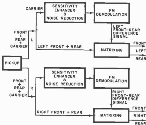
Fig. 2. Diagram of CD4 playback system.
