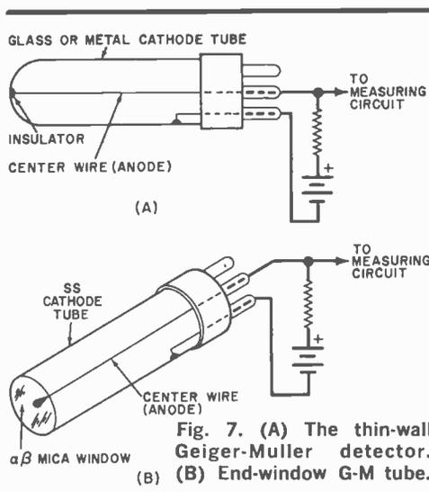
one point in the detector, while in the latter, the electron avalanche spreads along the entire length of the wire anode. The pulse size in the proportional detector varies with the number of secondary electrons produced. In the G-M tube, electron amplification is much larger so that the pulse size is practically independent of the number of electrons produced per nuclear radiation incident. The G-M tube, therefore, cannot discriminate between types of radiation.
