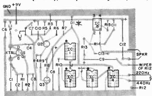
point, trimmer capacitor *C1* can be set to adjust the frequency as close as possible.
