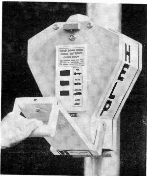
Using solid-state circuitry, the boxes derive their power from a patented electromechanical power module, which is activated when the door lever is opened. The electrical charge thus produced is retained temporarily to power the compact, integral FM transmitter. This means no batteries to run down and no dependence on regular electric power, which can fail just when motorists may particularly need help.
