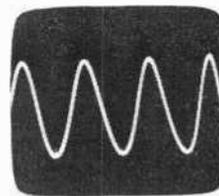
3.58 MHz sine-wave as shown on new RCA WO-535A in Recurrent Sweep Mode.
