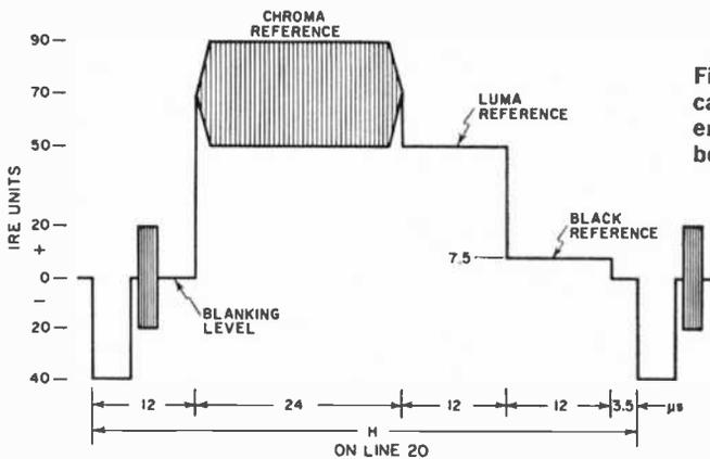
Fig. 5. Latest EIA test signal is called VIR (vertical interval reference) and is usually on line 20, both fields. It is being tested.
