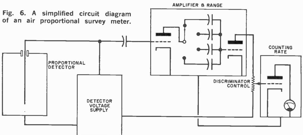
Fig. 6. A simplified circuit diagram of an air proportional survey meter.
