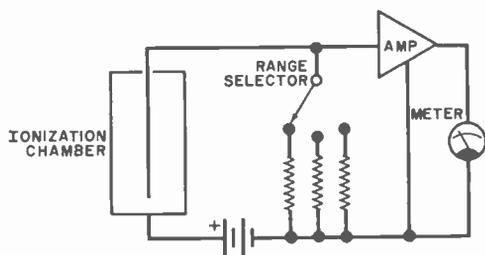
Fig. 3. Schematic of ionization survey meter.
