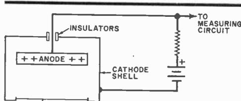
Fig. 1. Ionization chamber.
