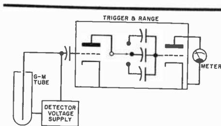
Fig. 8. Basic diagram of G-M survey meter.
