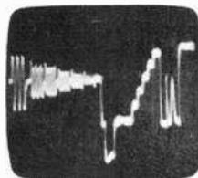
Typical TV VITS pattern on the new RCA WO-535A in Triggered Sweep Mode.
