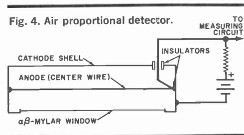
Fig. 4. Air proportional detector.
