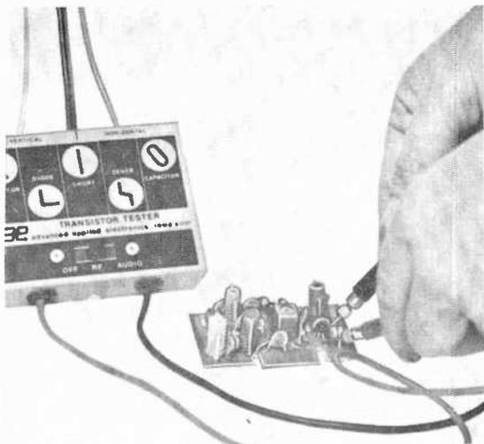
and the circuit under test. The two test leads are terminated in probes with needle tips to break through any PC board coating compound and make good electrical contact with the transistor leads.
