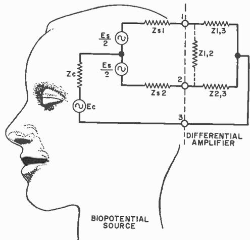
$Z_{1,2}$ =COMMON MODE INPUT IMPEDANCE
