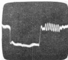
Expanded video signal on the new RCA WO-535A in Recurrent Sweep Mode shows the horizontal sync pulse and 3.58 MHz color-burst signal.
