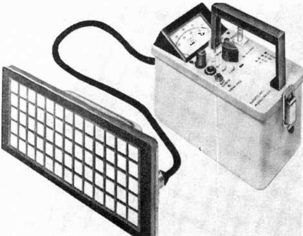
Fig. 5. An air proportional survey meter.
