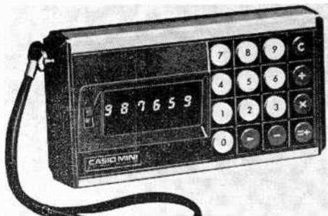
when performing division, the numbers displayed in the answer are the nearest whole-digit figures, while decimal figures are displayed by depressing the shift key. For all other arithmetic operations, the decimal point is located by interpolation. The readout indicators are 7-segment miniatures.
