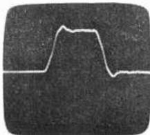
250-nanosecond ( $\frac{1}{4}$ -microsecond) pulse demonstrates trace expansion and rise time capability of the new RCA WO-535A in Triggered Sweep Mode.
