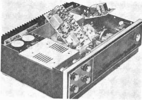
The audio amplifiers are probably the most impressive feature of the AR-1500. They are rated, with extreme conservatism, at 60 watts per channel into 8 ohms, 100 watts per channel into 4 ohms, and 40 watts per channel into 16 ohms, with both channels driven simultaneously. Harmonic distortion is rated at less than 0.25% from 20 to 20,000 Hz at 60 watts; and IM distortion is less than 0.1% at 60 watts.
