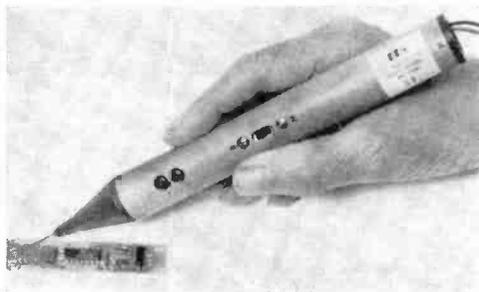
tronic logic quickly and simply and to diagnose digital malfunctions. The probe contains color-coded lamps which indicate logic levels. A memory feature which detects pulses as low as 3 ns in duration permits the tester to be used unattended. A gating feature allows the probe tip to be activated only when an auxiliary lead is in the selected logic state.
