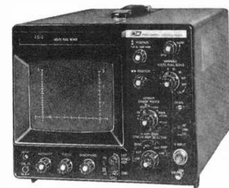
justment control). A built-in sync separator in the TV positions produces stable sync from a composite video input signal. The horizontal amplifier can also be driven from the power line or from an external source. Its gain control can be used to permit up to 2X trace expansion for close examination of any waveform. A pair of positioning controls completes the lineup.
