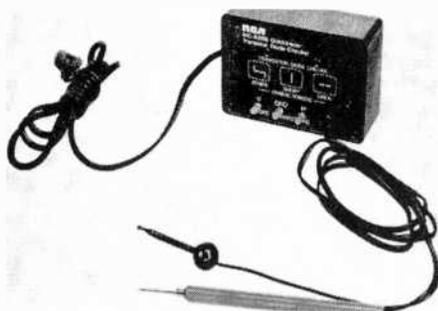
oscilloscope. When the two are paired together, the user has a handy means for checking all types of semiconductors except FET's. Too, it will even check many values of resistance and capacitance. The only difference between the A and B models is in the way they are mounted. The A model is plugged directly into the ac outlet (no cord), while the B version is attached to the side of the scope by a Velcro fasten-
