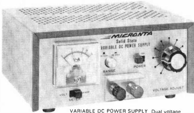
**VARIABLE DC POWER SUPPLY** Dual voltage range selector for 0-12 and 12-24 volts. Input 120 VAC at 60 Hz. Output current: 1.0 amp constant over entire range with 1.5 amp surge. Control adjusts output from 0-24 volts. Equipped with circuit breaker and housed in metal case 7-1/4 x 5-3/8 x 3". **29<sup>95</sup>**
