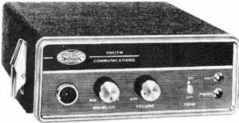
sions are Model 2103 (single-channel) and Model 2104 (four-channel). Operating power is from a 13.8-volt dc, negative ground only, source. In the Models 2102 and 2104, channel selection is via a bank of pushbutton switches.
