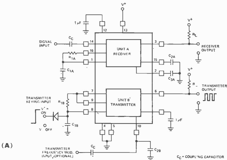
Fig. 2. Two applications for the XR-2567 dual tone decoder. In the duplex tone transceiver circuit shown at (A), unit A serves as a tone receiver and unit B as a tone transmitter. In (B), at right, only half of the IC is utilized to form a precision oscillator for use in circuits such as a musical instrument tone generator.
