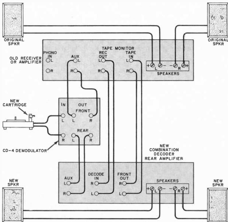
Fig. 3. A combination decoder/amplifier reduced the number of electronic components required—unless you want to add CD-4 disc playing capability.
