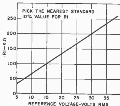
Fig. 3. Use this chart to determine value of *R1* (Fig. 2) when 60-Hz reference voltage level in rms is known.
