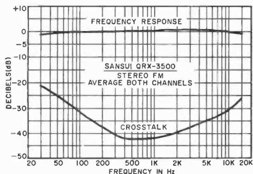
kHz pilot-carrier leakage was 69.5 dB down. Channel separation was better than 21 dB from 30 Hz to 15,000 Hz and exceeded 40
