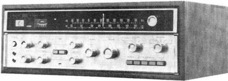
**T**HE Model QRX-3500 4-channel stereo receiver is one of the new line of products made by Sansui which uses their Vario-Matrix (a logic controller that enhances the stereo separation inherent in the QS system). The Vario-Matrix compares the phases of the two input channels and controls the matrix coefficients to accentuate separation without "pumping" or other audible side effects encountered with other decoding systems.
