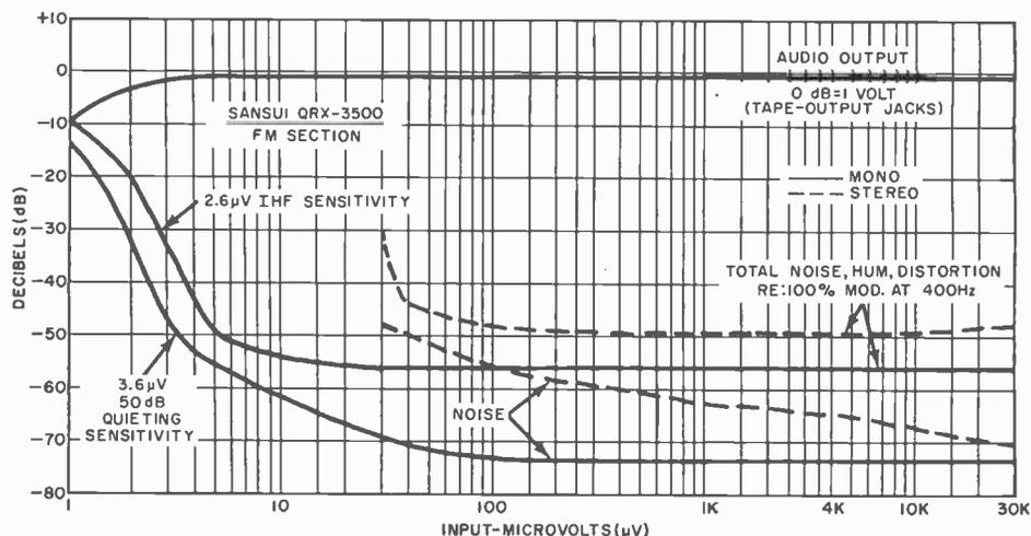
The FM capture ratio was 1.75 dB, and AM rejection was 49 dB. Image rejection was better than rated, measuring 77 dB. The receiver proved to be slightly better than its rated 50-dB alternate-channel selectivity figure, measuring 51.5 dB on one side of the signal and 65 dB on the other side.
