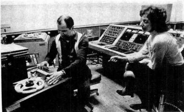
Many tracks are equalized, enhanced and mixed electronically to make master tape.
