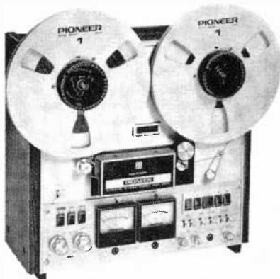
modate professional 10½-in. tape reels. It offers unique two-step equalizer and three-step bias selection that permits its use with all available tape formulations. The deck will record and play back in the standard 2-channel/4-track stereo format. Additionally, the playback head permits playback of discrete 4-channel stereo tapes.
