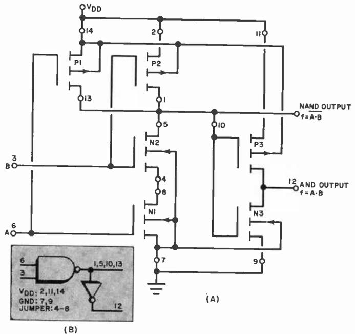
put will be low. If both inputs are low, the output is high. The NOR logic is performed by *P1*, *P2*, *N1*, *N2*. If either the A or B input is high, *N1* or *N2* is held low by the low on resistance of *N1* (or *N2*). Also, during a high input, either *P1* or *P2* is off, so there is no series path to  $V_{DD}$ . But suppose both inputs are low. Then, both *P1*
