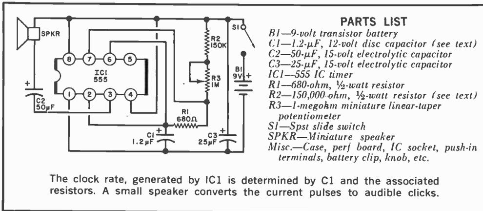
through coupling capacitor C2. Using small resistance values for R1 and large values for R2 and R3 produces brief pulses at moderate time intervals, with potentiometer R3 determining the repetition rate.
