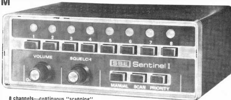
**8 channels**—continuous "scanning". Receiver locks on first channel on which signal appears.
