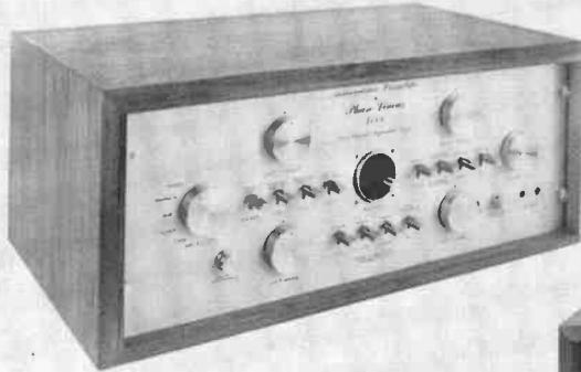
**Phase Linear's 4-channel Autocorrelation Preamp boasts special hiss- and noise-reduction circuits, dynamics restorer and active equalizer (left).**
