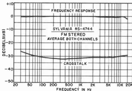
(We were pleased to note that the equalization was not affected significantly by cartridge inductance, unlike the case with most amplifiers, which exhibit loss of several decibels at 10,000 Hz or higher from this interaction.)
