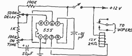
shield-wiper control. I originally planned on using transistor switching, but too much power was wasted in base current. So, I opted for relay switching.
