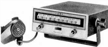
dc input. Ten pushbutton switches are mounted on the front panel for channel selection. Eight-pole second i-f filters are incorporated for selectivity, and r-f output devices are VSWR-protected. The GTX-2 comes with quick-disconnect power cable, SO239 antenna connector, a mobile mounting bracket and a ceramic plug-in microphone. Optional accessories include the TE-1 tone pad for autopatching, a variety of power supplies, antennas, receiver preamp, and auxiliary speaker.
