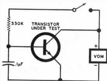
ployed to make a low-cost transistor tester that can be used to check leakage and give a rough idea of the beta of an unknown transistor. The circuit is shown in the test setup for npn transistors, but all you have to do is reverse the leads of the VOM when checking pnp devices.
