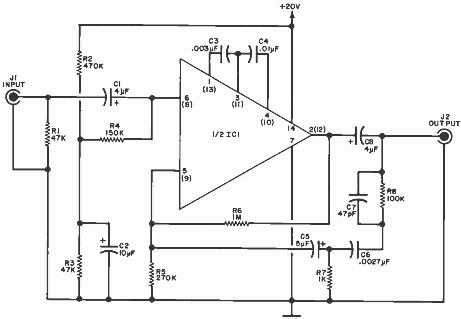
*Fig. 5. In this reader's circuit, an op amp IC is used as the basis for a preamplifier. Both halves of the IC can be used for a stereo system. Distortion is low and channel separation good.*
