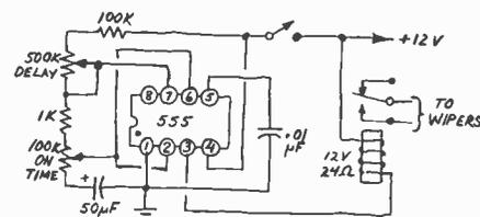
shield-wiper control. I originally planned on using transistor switching, but too much power was wasted in base current. So, I opted for relay switching.
