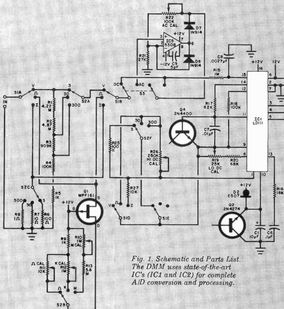
Fig. 1. Schematic and Parts List. The DMM uses state-of-the-art IC's (IC1 and IC2) for complete A/D conversion and processing.
