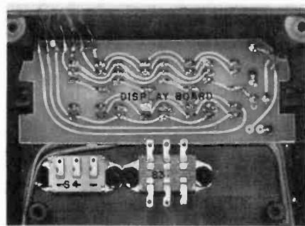
*Fig. 3. Photo shows installation of S3 and S4.*
