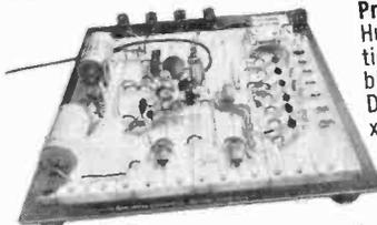
Proto Board 104. Huge. 3,060 solderless tie points. (4) 5-way binding posts. 32-14 pin DIP capacity. 9 $\frac{1}{2}$ " long x 8" wide. **79<sup>95</sup>**
