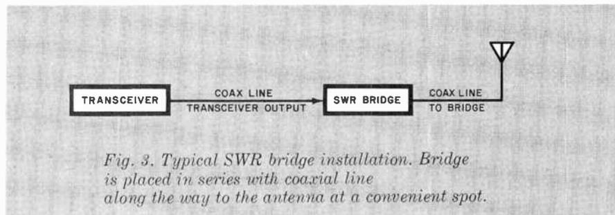
*Fig. 3. Typical SWR bridge installation. Bridge is placed in series with coaxial line along the way to the antenna at a convenient spot.*
