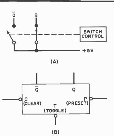
Fig. 1. Switch analogy (A) and logic (B) of a flip-flop.
