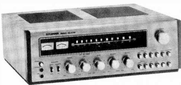
**T**HE MODEL RS-4744 is Sylvania's finest AM/stereo FM receiver. Its FM tuner section features a phase-locked loop (PLL) multiplex decoder and direct-coupled 60-watt/channel power amplifier. Switching is provided for two pairs of speaker systems and for driving rear speaker systems with a modified difference signal for a simulated 4-channel effect from stereo programs.
