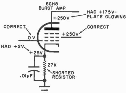
*Fig. 2. Voltage readings showed a shorted resistor.*
