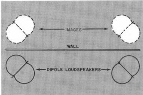
*Fig. 1. When two dipole radiators are placed at angles near a wall, the listener at L is at the null points of the reflected signals and the stereo image is not affected.*
