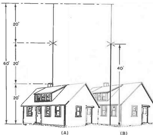
Fig. 3. The 20-foot rule is still applicable for beam antennas.
