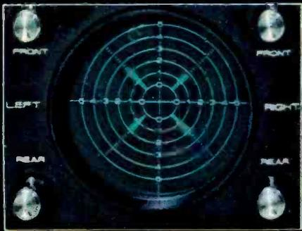
**Four-Channel Level Indicator — See what you hear. Make instant adjustments with left/right, front/rear level controls.**
