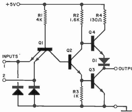
about 1.8 volts. The values of R2 and R3 are selected so that, when Q2 is conducting, the voltage drop across R3 is high enough to turn on Q3. But the voltage at the collector of Q2 is not high enough to cause Q4 to conduct. The "0" output is then only a junction away from ground (through Q3). Note that in this state, the output (via Q3 to ground) can sink a reasonable amount of current—approximately 16 mA. This is why TTL is sometimes referred to as "current-sinking logic."
