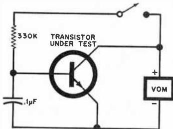
ployed to make a low-cost transistor tester that can be used to check leakage and give a rough idea of the beta of an unknown transistor. The circuit is shown in the test setup for npn transistors, but all you have to do is reverse the leads of the VOM when checking pnp devices.
