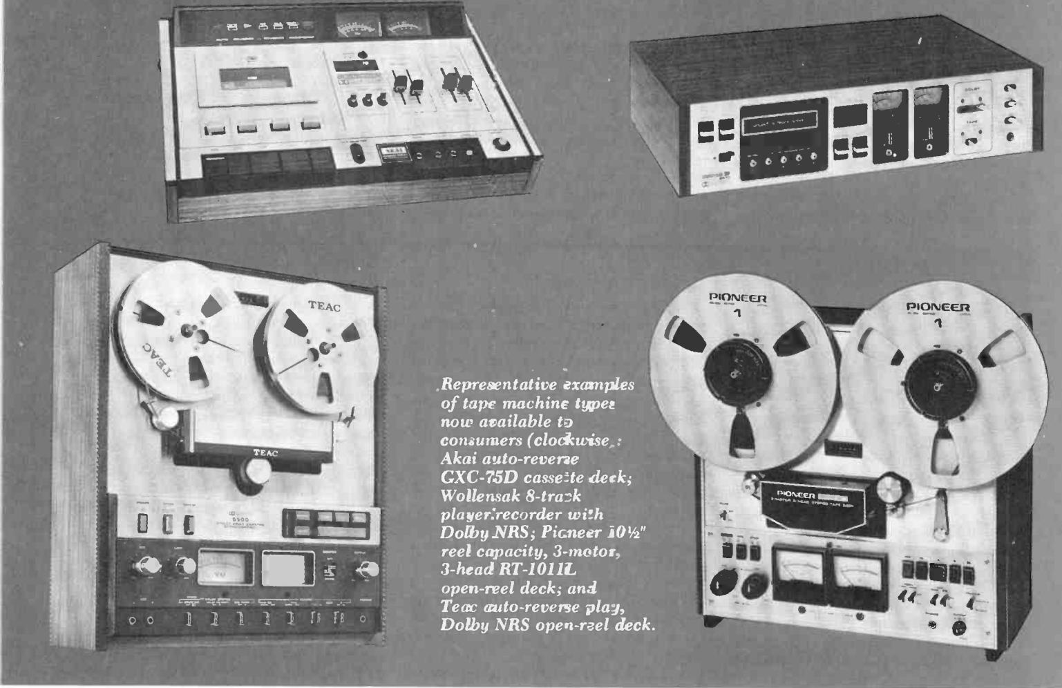
*Representative examples of tape machine types now available to consumers (clockwise): Akai auto-reverse GXC-75D cassette deck; Wollensak 8-track player/recorder with Dolby NRS; Pioneer 10½" reel capacity, 3-motor, 3-head RT-101L open-reel deck; and Teac auto-reverse play, Dolby NRS open-reel deck.*
