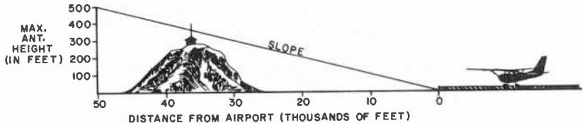
Fig. 4. This antenna near an airport would be against the rules.
