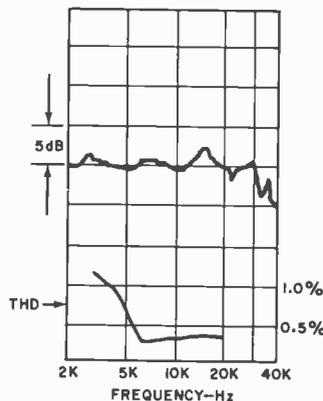
**Fig. 2. Frequency response and distortion for piezo speaker.**
