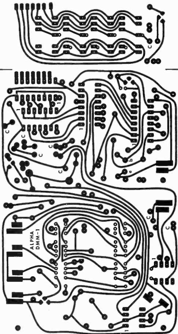
*Fig. 2. Actual-size foil patterns for display (top) and main (below) boards.*
