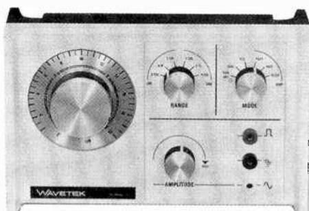
NOT TOO long ago, the only economical way of plotting the response of an audio amplifier, filters, and the like was by point-by-point entry on graph paper at various frequencies obtained from a signal generator. The process was time-consuming and tedious. No matter how you approached the problem, you had to look forward to many hours of dial "twiddling," reading and recording an output meter indication, and laboriously plotting the resulting curve.
