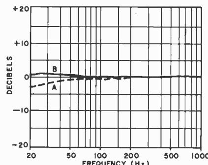
*Fig. 1. Curve A shows frequency response with amplifier adjusted for 10-kilohm input impedance; while B is response with 50-kilohm impedance.*
