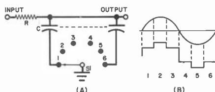
Fig. 2. Circuit of an experimental digital filter for the audio range (right).
