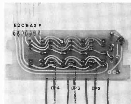
Fig. 4. Component layout for the display board.
