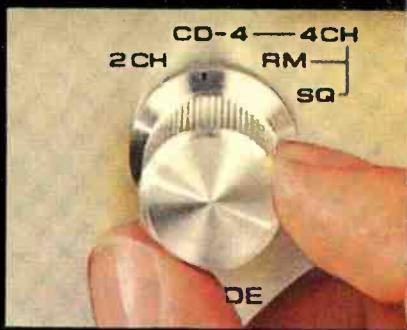
**Total Capability Mode Switch — Fingertip switching to CD-4, SQ, RM quadraphonic sources, as well as two-channel stereo.**
