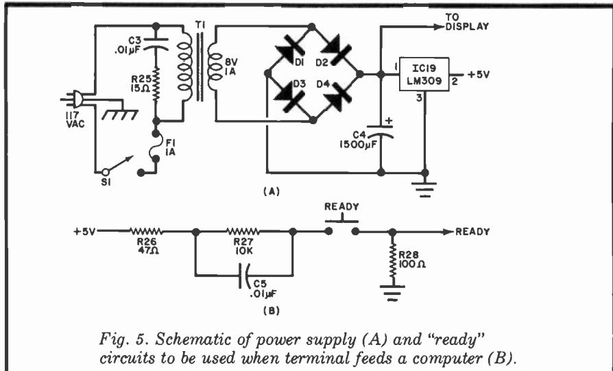
Fig. 5. Schematic of power supply (A) and "ready" circuits to be used when terminal feeds a computer (B).
