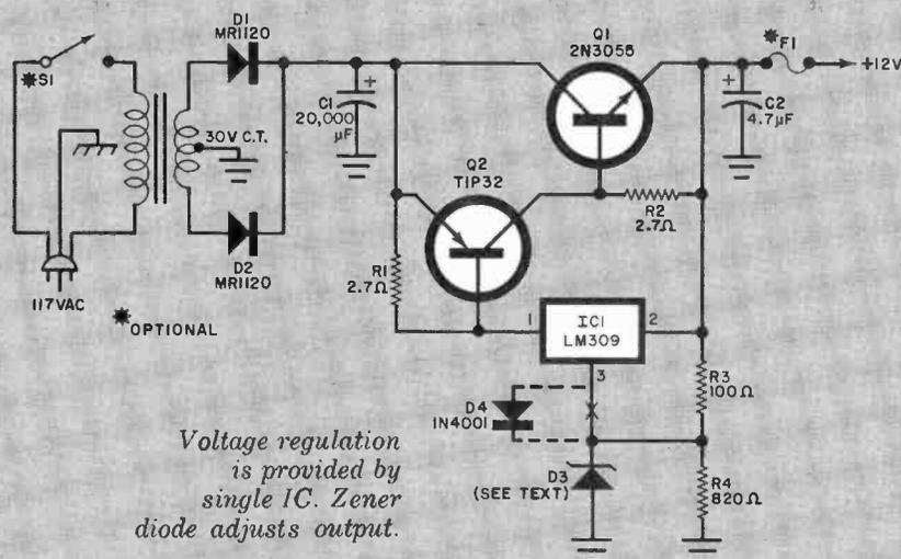
*Voltage regulation is provided by single IC. Zener diode adjusts output.*
