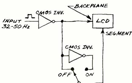
Fig. 3. Practical circuit for driving an LC display.
