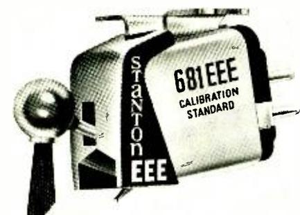
The Model 681-EEE is the successor to and supersedes Stanton's Model 681EE stereo phono cartridge. In fact, the two models have identical external appearance, except for the difference in nomenclature marked on the removable stylus assemblies. The principal design difference between the two is that the EEE's stylus mass has been reduced by about one third.
