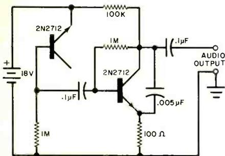
reverse-biased pn junction of a 2N2712 transistor is used as a noise generator. The second 2N2712 is an audio amplifier. The 0.005- $\mu$ F capacitor across the amplifier output removes some high-frequency components to simulate pink noise more closely. The audio output may be connected to high-impedance earphones or to a driver amplifier for speaker listening.
