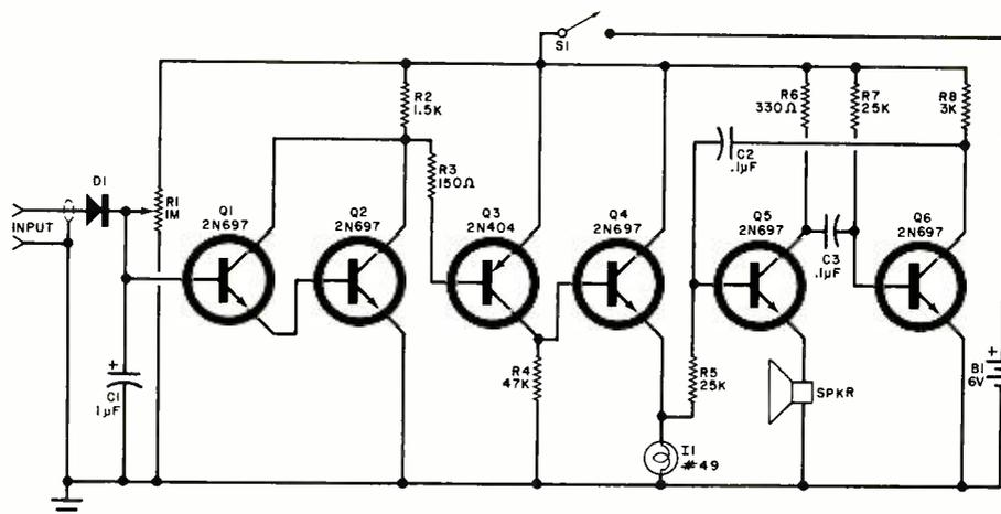
Neither layout nor lead dress should be overly critical although, because of the multiple stages involved, good wiring practices should be followed when duplicating the design. Signal-carrying leads should be kept short and direct and care should be taken not to overheat the semiconductor devices when soldering them in place. A pc board might be advisable.
