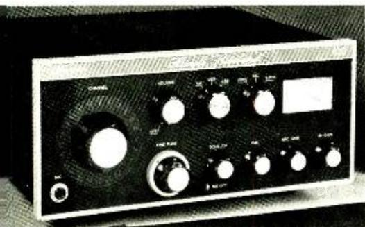
**H**Y-GAIN'S Model 623A base station Citizens Band transceiver is designed for both AM and SSB operation. In some respects, it differs from other AM/SSB rigs. For example, the circuitry is all solid-state in design, except for the transmitter's power amplifier stage, which is a vacuum tube. This design departure greatly reduces the chance of damage to the power amplifier due to mismatched loads.
