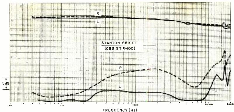
sponse, we temporarily increased the load to 480 pF, which is as high as will ever be encountered in practice. This increased the drop rate in the output curve at frequencies beyond 10,000 Hz, amounting at 20,000 Hz to an additional 5 dB. The Model 681EEE obviously does not require excessive circuit capacitance to equalize its frequency response as do some other cartridges. It should deliver optimum performance with almost any load.
