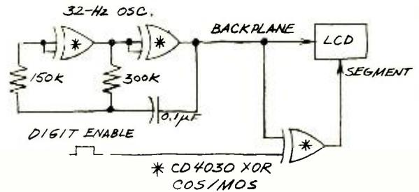
The drive voltage's amplitude in an LCD circuit is important. At least its rated voltage must be supplied to the display, which is the normal battery voltage in most CMOS systems. It is usually safe to exceed this voltage without harm, but the display segments might start to come on without being addressed as a result of internal display leakage if the voltage applied is too high.
