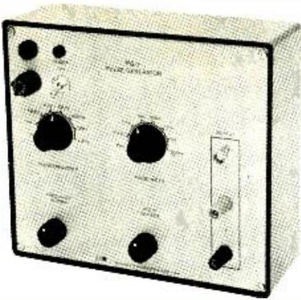
**Some Details.** Assembling the kit took us only an evening of unhurried work. No special tools were required, and we encountered no difficulties in putting the kit together. Everything mounts on the front panel, and even the line cord exits through a hole in the panel, held in place by a plastic strain relief. When we plugged the line cord into an ac outlet and turned on the power, the instrument worked properly the first time out.
