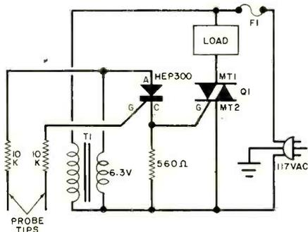
Q1, is not given a specific part number since various loads demand different currents. Check how much current your load demands and obtain a triac that can handle this amount. The triac should be well heat-sinked. Use the same current rating for F1 as Q1, and make it a quick-acting type fuse. The resistors may be mounted on a board, with leads in the clear used as probe tips.
