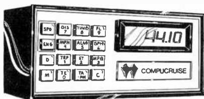
in the car, it monitors battery voltage, speed, fuel flow, distance, time and air temperatures both inside and outside the
