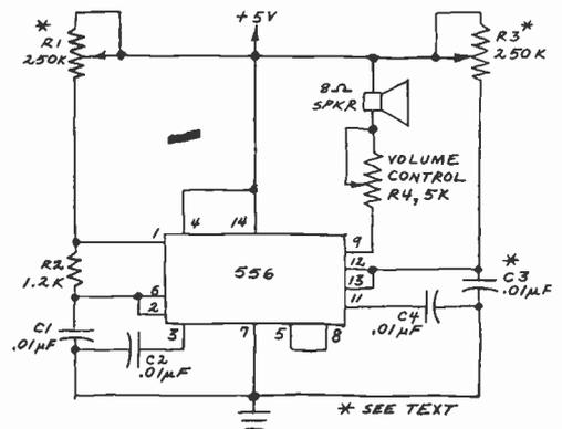
Fig. 4. A stable-monostable divider.
