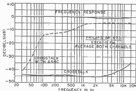
Frequency response and crosstalk averaged for both FM sections, with dashed line showing effect of Automatic Stereo Noise Canceling. Active signal level is less than 32 dBf.
