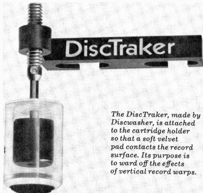
*The DiscTraker, made by Discwasher, is attached to the cartridge holder so that a soft velvet pad contacts the record surface. Its purpose is to ward off the effects of vertical record warps.*
