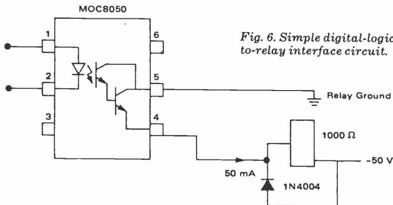
Fig. 6. Simple digital-logic-to-relay interface circuit.
