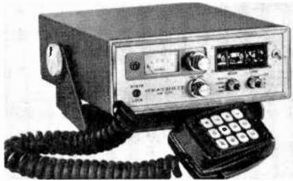
**T**HE Model HW-2036 is the Heath Company's latest and most sophisticated vhf FM amateur transceiver. Among its features are synthesized coverage of any 2-MHz segment from 143.5 to 148.5 MHz in 5-kHz increments, true FM transmitter circuitry, dual-conversion receiver with MOSFET front end, and a 10-watt minimum-output power amplifier designed to operate into an infinite VSWR without failure.
