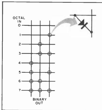
Fig. 4. A ROM programmed as an octal-to-binary encoder, a circuit usually designed with OR gates.
