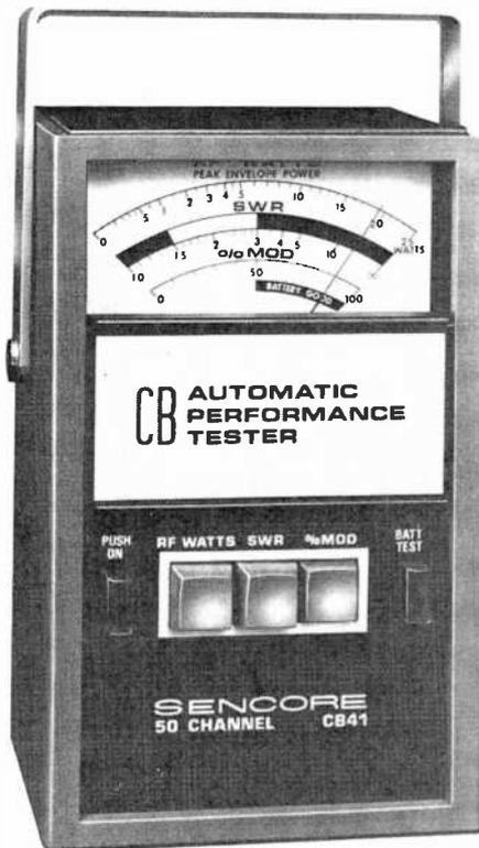
**T**HE Sencore Model CB41 automatic CB performance tester conveniently checks the operation of CB transmitters. It provides measurements of r-f output power directly in watts, peak-envelope power (PEP) on SSB and AM, percent modulation for AM, and the standing-wave ratio (SWR) presented by the transmitter load or antenna system.
