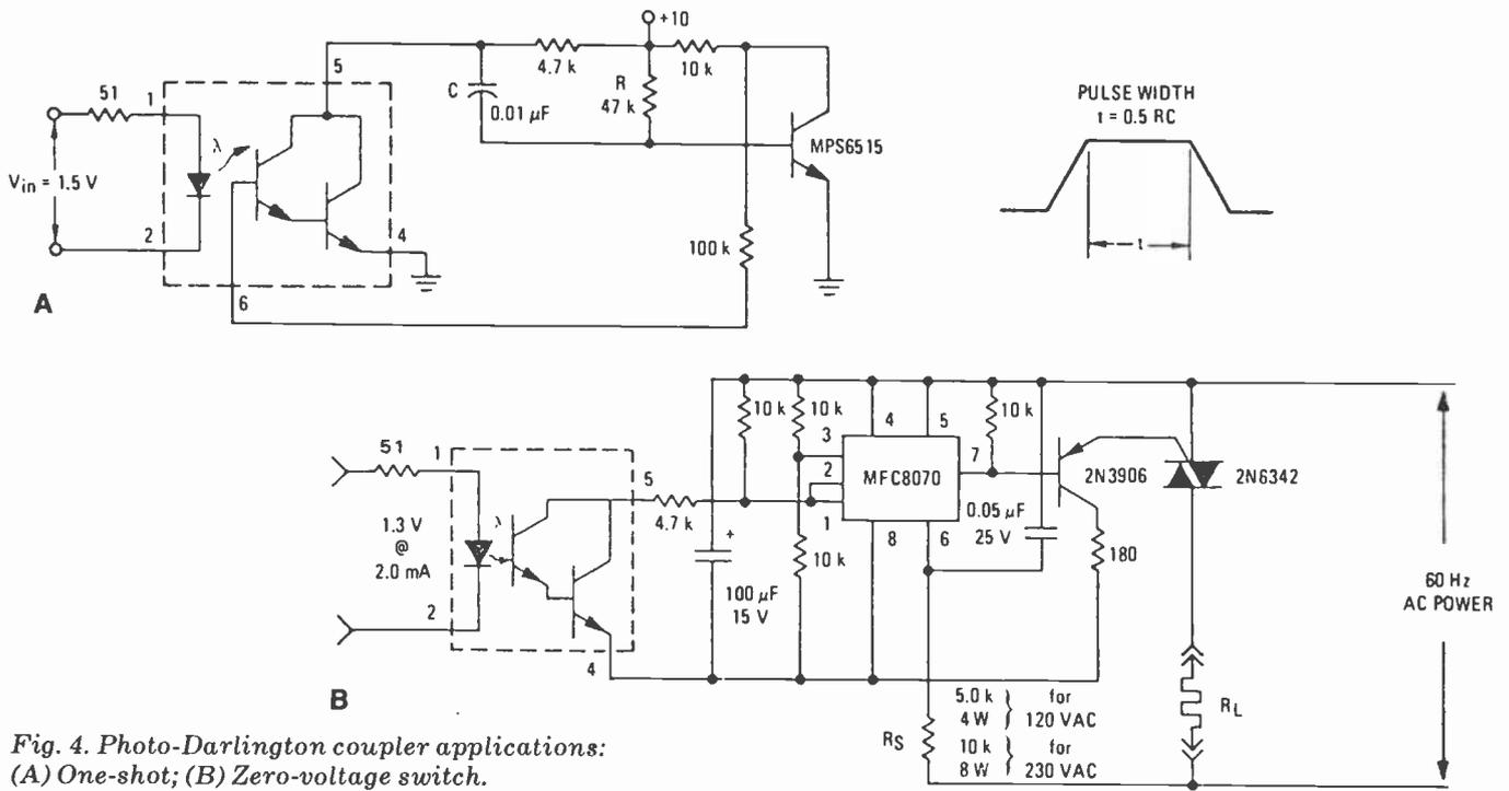
Fig. 4. Photo-Darlington coupler applications: (A) One-shot; (B) Zero-voltage switch.
