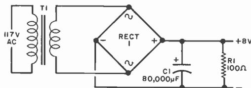
Fig. 1. Basic 8-volt, 15-ampere dc source. Note heavy wiring between elements.
