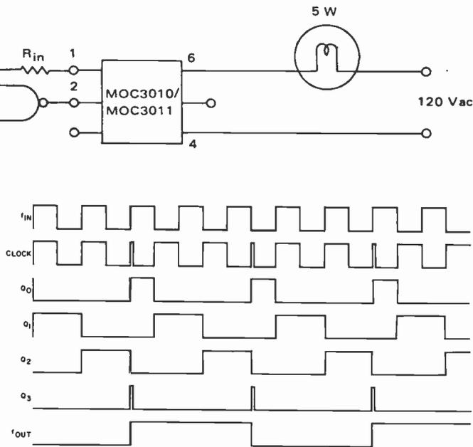
Fig. 9. Timing diagram for the frequency divider circuit in Fig. 8.
