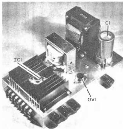
This TO-3 size protection circuit will fire the crowbar at 6.6 volts. Note that pin 1 of this circuit is left floating for proper operation in this application.
