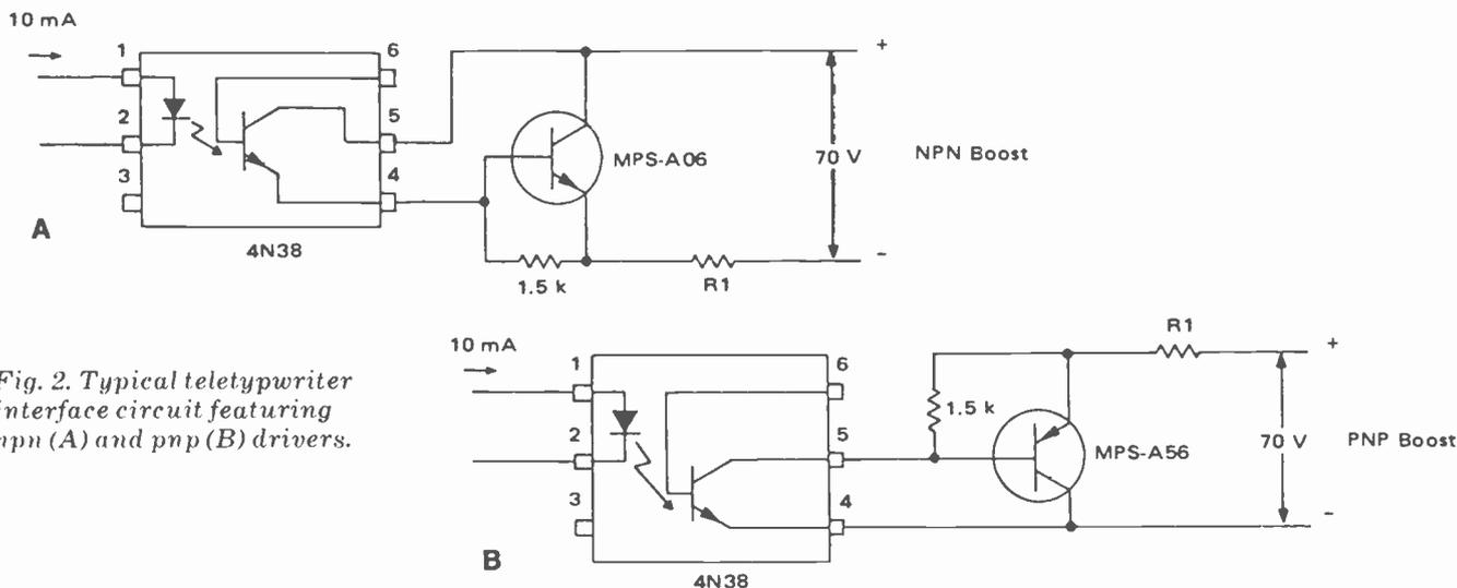
Fig. 2. Typical teletypewriter interface circuit featuring npn (A) and pnp (B) drivers.
