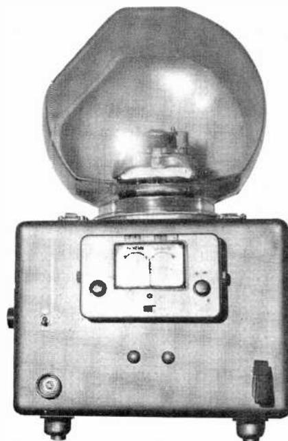
At right is author's prototype of eddy-disk magnetometer.
