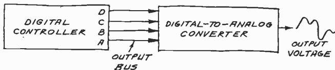
Fig. 1. Connecting digital controller to D/A converter.
