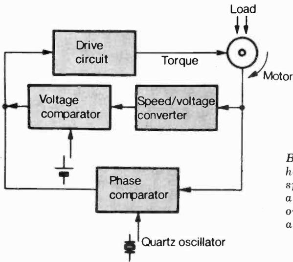
Block diagram shows how motor rotational speed is "locked" to a reference frequency originating in a quartz oscillator.
