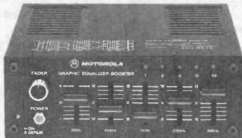
Motorola equalizer/booster has 30-W rms power output, LED power indicators.
