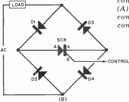
Fig. 4. Using a bridge rectifier as an automatic polarity switch.
