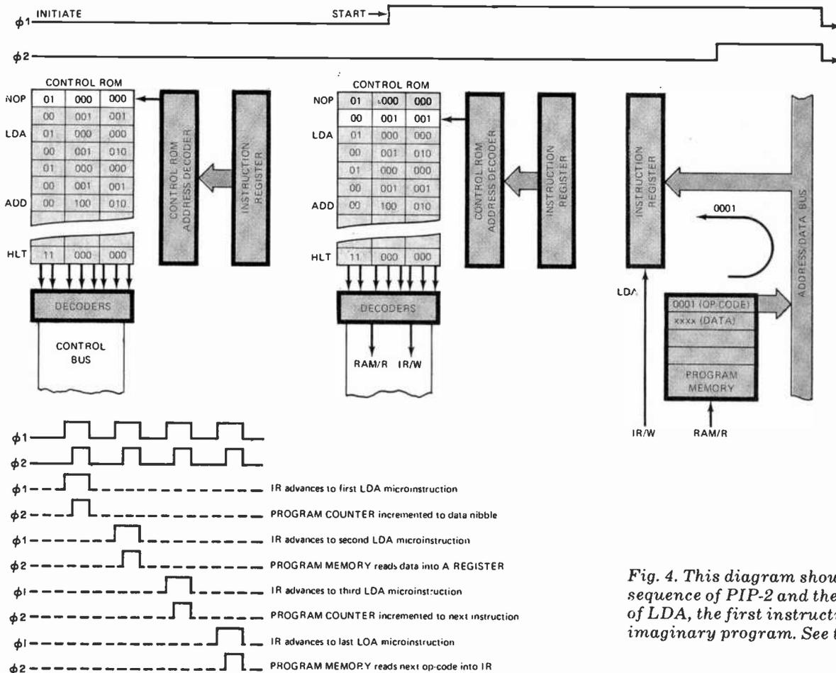
Fig. 4. This diagram shows the start sequence of PIP-2 and the execution of LDA, the first instruction in an imaginary program. See text for details.
