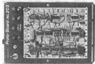
provide additional power and signal connections. The power supply is rated at 1 A,  $5 \pm 0.25$  V, with 10 mV combined ripple and noise at  $\frac{1}{2}$  A out, and is protected against short circuits. Dimensions are  $6\frac{1}{4} \times 3\frac{1}{4}$  in. (16.5 x 24.8 x 8.3 cm). \$80.
