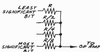
Fig. 2. Simple 4-bit D/A converter using resistor ladder.
