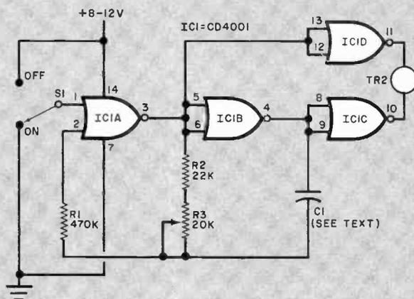
Fig. 2. This ultrasonic transmitter employs four NOR gates.
