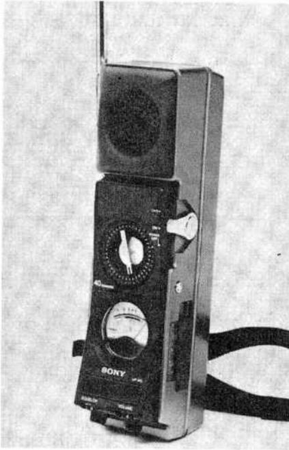
The hand-held Model ICB-1020 AM transceiver from Sony uses the latest in phase-locked-loop (PLL) synthesizers to provide coverage on all 40 CB channels. It is powered by eight AA cells that fit within its housing and has provisions for obtaining power from a 12-volt mobile electrical system and, with an adapter, standard 117-volt ac line power. Whichever power source is used, the rated r-f output power from the transmitter is 1 watt.
