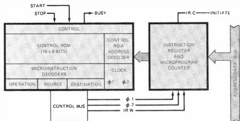
Fig. 1. Organization of the PIP-2 control section.
