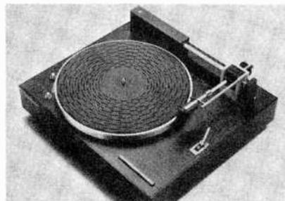
lus overhang. A "Hall-effect" servo-controlled dc motor drives the 2.4-lb (1.1-kg) turntable via a belt. The platter is brought to selected speed from a dead stop in only one revolution, according to the manufacturer. Wow and flutter is said to be 0.05%;
