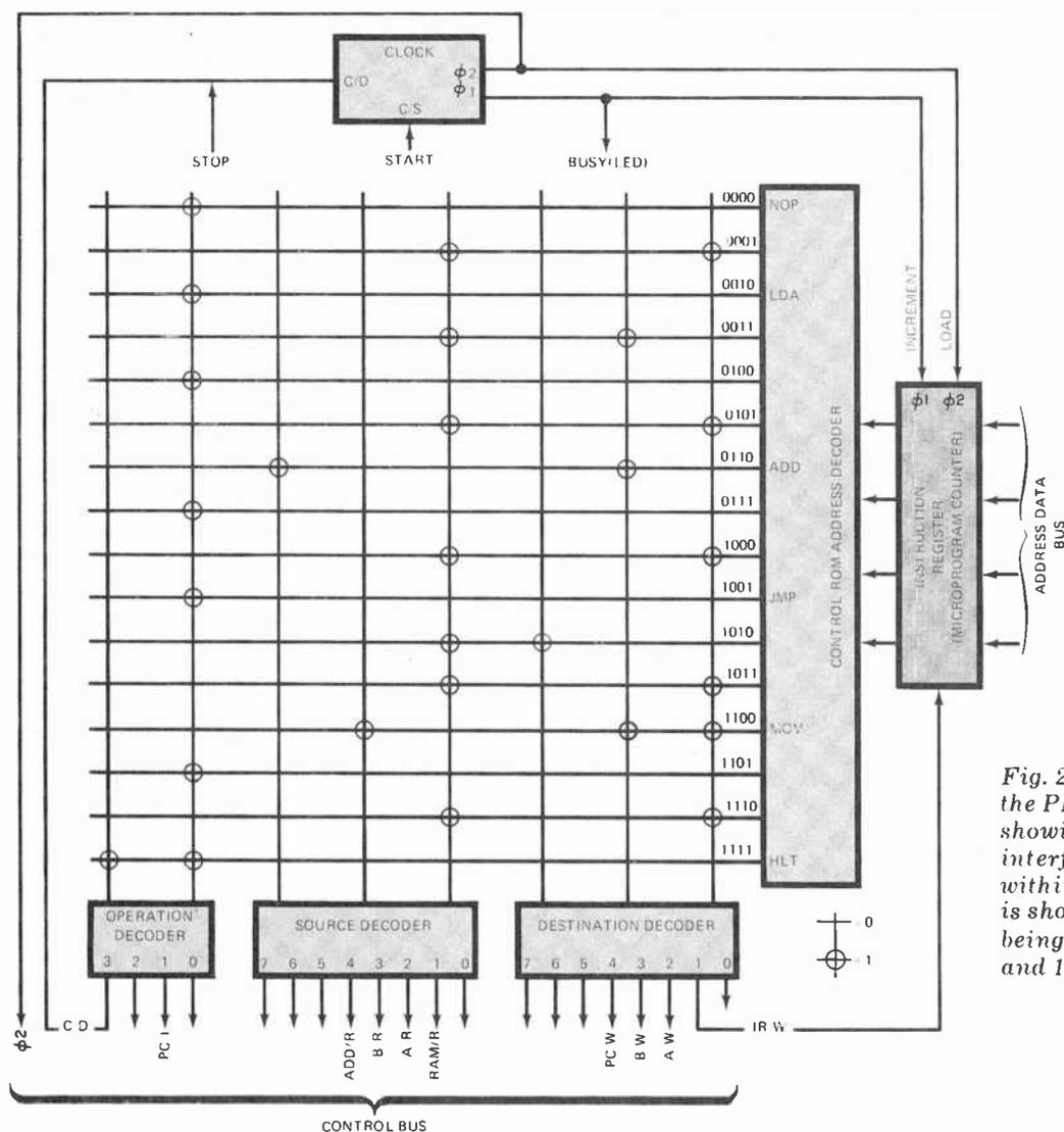
Fig. 2. Internal details of the PIP-2 control section showing how the three decoders interface with the microprogram within the ROM. Here, the ROM is shown as a matrix with 0's being unconnected junctions and 1's having a connection.
