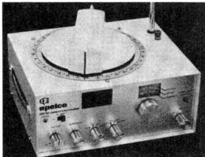
and standard AM broadcasts. The DF-10 features a switchable noise limiter and a bfo. Another tuning aid provided is a sensitivity meter, which doubles as a power cell strength indicator. The solid-state radio direction finder is powered by eight "D" cells. Dimensions are 7.5"H x 11"W x 9"D (19.1 x 27.9 x 22.9 cm). Weight is 8.5 lb (3.9 kg). \$249.
