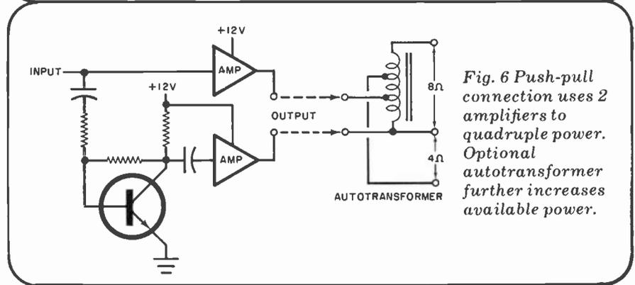
Fig. 6. Push-pull connection uses 2 amplifiers to quadruple power. Optional autotransformer further increases available power.
