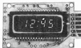
Just add switches and install! 12-hour readout, 0.3" digits, ±0.5 sec./day accuracy. 12VDC. 277-1003. Reg. 24.95 ..... Sale 19.95
