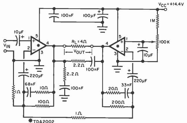
Fig. 6. Power amplifier bridge configuration.
