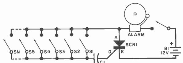
Fig. 7. Burglar alarm uses sensors in parallel.
