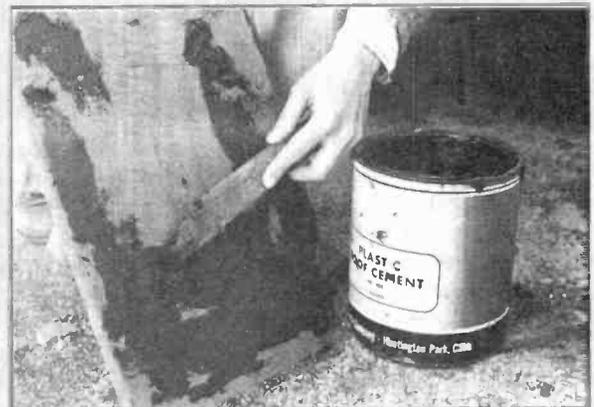
Sound-deadening board, secured with roofing cement, suppresses rattles and resonances which may occur with sheet-metal door panels.
