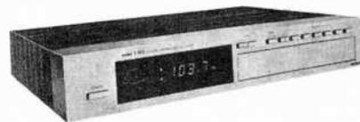
plished in 200-kHz steps, and the T-909 displays the frequency to which it is tuned on front-panel, seven-segment LED's. Among the features of the T-909 is its seven-channel, user-programmable memory. This allows station selection at the push of a button. Other features include Dolby NR adaptor plug-in provisions and a deemphasis switch, front-end dual-gate MOSFET's, multipath detector terminals, and a "birdie"
