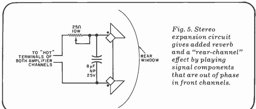
Fig. 5. Stereo expansion circuit gives added reverb and a "rear-channel" effect by playing signal components that are out of phase in front channels.
