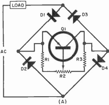
Fig. 3. Using a bridge rectifier to control an ac load: (A) Transistor control; (B) SCR control.
