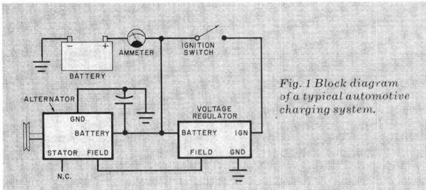
*Fig. 1 Block diagram of a typical automotive charging system.*
