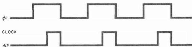
Fig. 3. Timing diagram of the PIP-2 two-phase clock.
