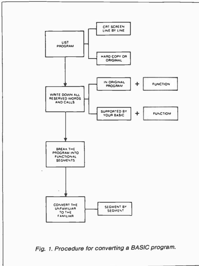
Fig. 1. Procedure for converting a BASIC program.
