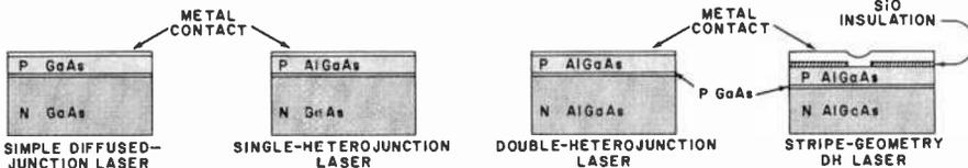
Fig. 3. Simplified cross sections of the four most important kinds of injection lasers.
