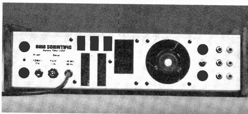
Rear panel of C4P with I/O ports.
