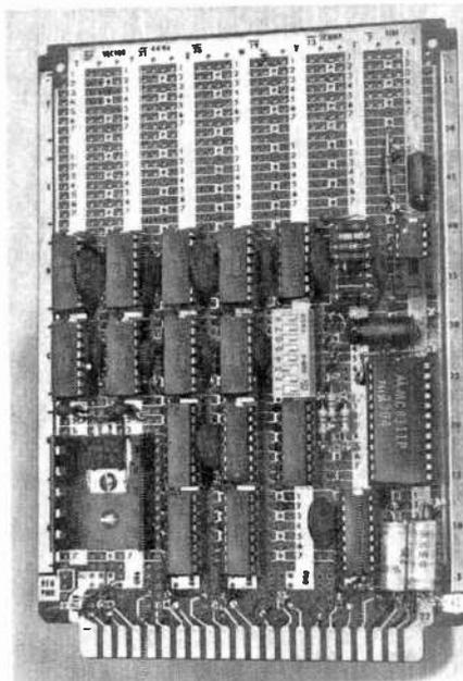
The memory expansion system mounted on a 4494 plug board. There is room for eight additional RAMs if desired.
