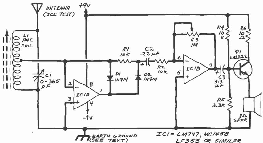
Fig. 2. An AM radio using an operational amplifier.
