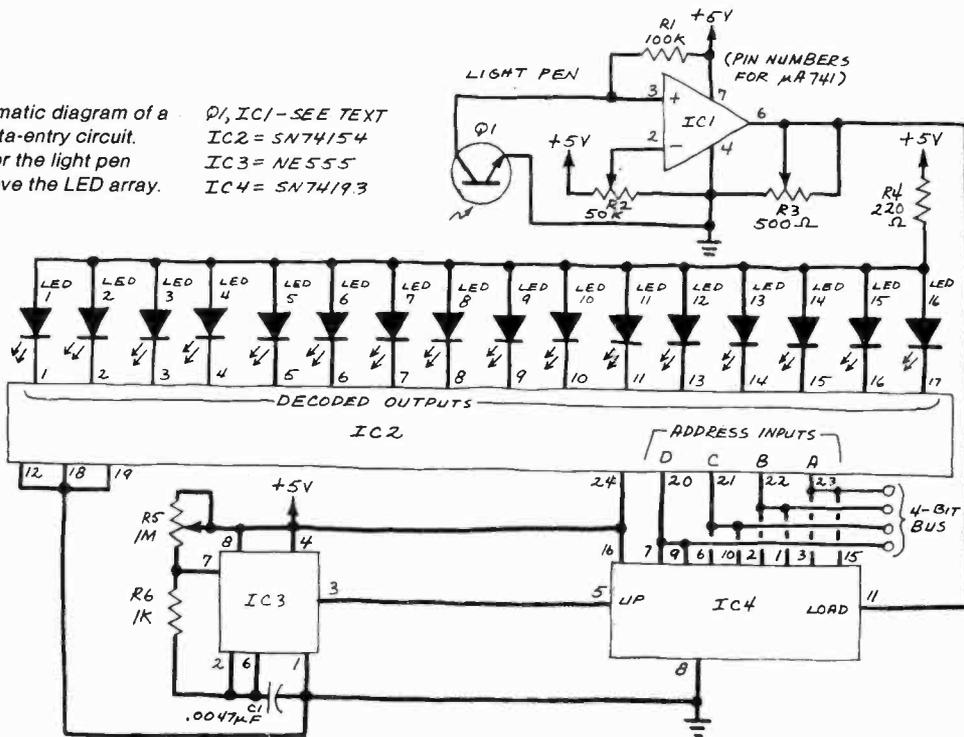
address of the selected LED will then appear on the 4-bit bus between IC2 and IC4.
