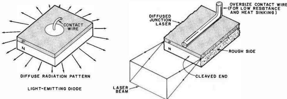
Fig. 1. Comparison of the physical structures of a light-emitting diode (left) and a simple diffused-junction laser.
