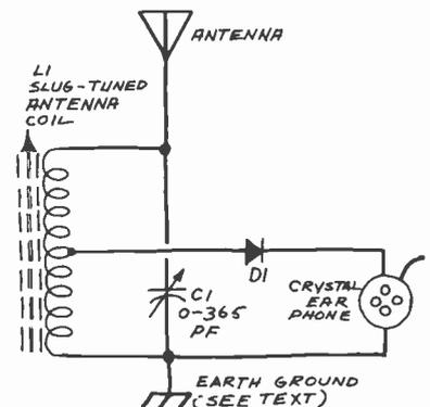
Fig. 1. Super-simple diode AM radio.
