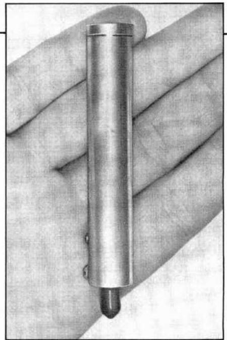
Fig. 6. A battery-driven miniaturized single-heterojunction laser transmitter.
