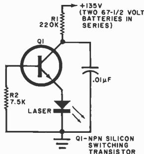
Fig. 5. Simple pulse driving circuit for injection laser.
