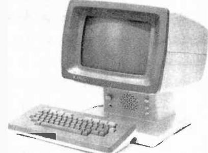
processors, a CRT screen and speech synthesizer. Phonetic characters plus rules for enunciation are fed into the synthesizer and the product is clear synthetic speech for a blind computer
