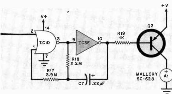
Fig. 2. The circuit in the project uses a CMOS phase-locked loop to detect the presence of the alert signal. The CMOS components cause little battery drain so that the monitor can be in use constantly.
