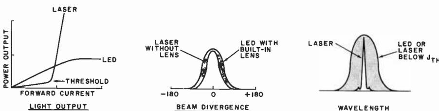
Fig. 2. Comparing the chief operating characteristics of light-emitting diodes and junction lasers.
