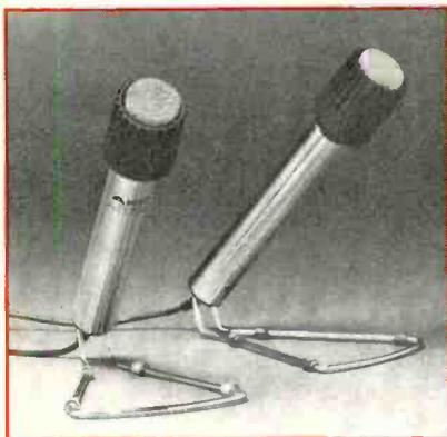
The D-40 from AKG is a moving-coil microphone sold in matched stereo pairs. Frequency range is 80-15,000 Hz, rated impedance is 600 ohms, and sensitivity at 1,000 Hz is -55 dBV. A pair of D-40s, whose pickup patterns are cardioid, comes packaged in a kit with two stands and eight-foot shielded cables. \$99 a pair.
