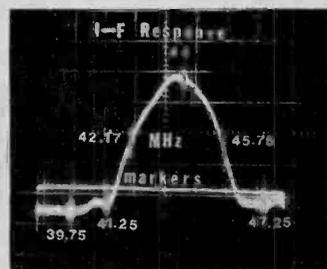
Fig. 4. Factory alignment is good except for placement of lower audio adjacent channel marker, which could be closer to response curve.
