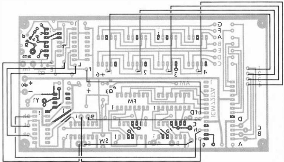
Fig. 5. Foil pattern and component layout for the prescaler board.
