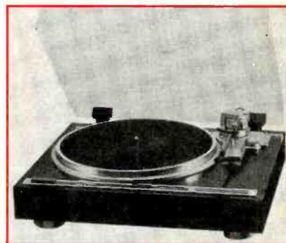
The HT-500 from Hitachi features the Unitorque motor, which is said to provide constant torque as the platter rotates. The motor is brushless, slotless, and coreless; and is regulated by reference pulses from a crystal oscillator. Sensing tonearm position optically, the unit is fully automatic. The tonearm itself is a straight low-mass design. The platter is of aluminum alloy. S/N is 78 dB; wow and flutter, 0.025% wrms. \$330.
