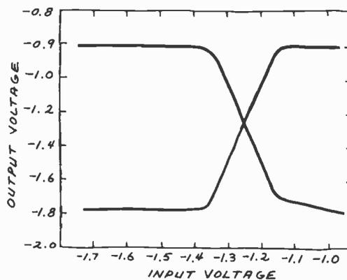
Fig. 2. Transfer curves of a typical ECL gate. The difference between a high and a low is only about 0.85 volt.
