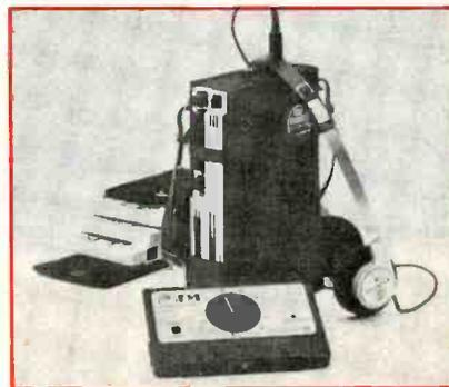
DNR (Dynamic Noise Reduction) is the major feature of Technidyne's model 140 Hip Pocket Stereo. DNR, a low-pass filter system whose cutoff frequency varies with program content, is said by the manufacturer to rid the program source of noise, as well as to prevent noise from being added by the playback equipment. In the model
