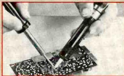
The new DP-1 desolder pump from OK Machine and Tool Corp. features all-metal construction and compact size for one-hand operation. Suction is said to be precisely regulated to minimize damage to delicate circuitry. Self-cleaning on each stroke, the DP-1 can be disassembled without tools for maintenance or repair. The tip is made of Teflon. \$10.95.
