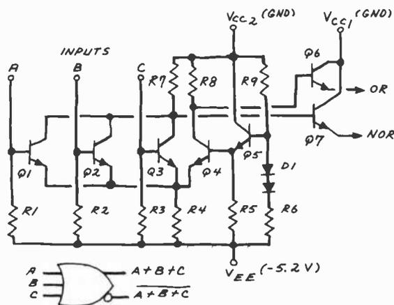
Fig. 1. An emitter-coupled logic (ECL) 3-input OR-NOR gate.
