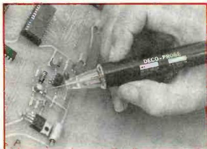
The Deco-Probe from Deco Sales is intended for use on TTL, CMOS, and microprocessors with voltages from 5 to 18 V. The circuitry is said to automatically adjust thresholds and to detect logic levels. Pulse detection is claimed for intervals down to 50 ns. The red and green LED display illuminates the point of circuit contact through a light-pipe nose piece. \$19.95, kit form; \$29.95, assembled.
