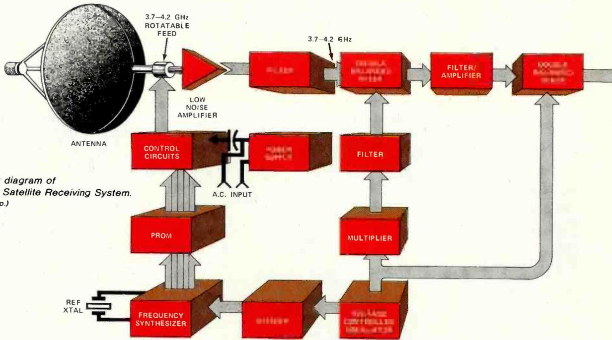
Fig. 1. Basic block diagram of Megastar/TVRO-1 Satellite Receiving System. (Courtesy Microdyne Corp.)
