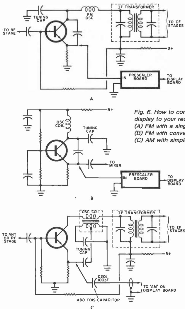
Fig. 6. How to connect the digital display to your receiver: (A) FM with a single-stage converter; (B) FM with conventional local oscillator; (C) AM with simple converter.
