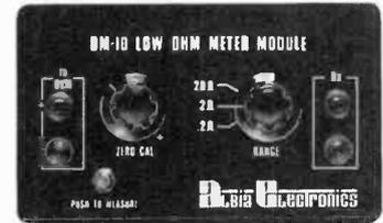
Measures resistance from 10 milliOhms to 20 Ohms. Now you can measure resistance down to 10 milliOhms with this low cost, easy to use DVM module. Check coil resistance, transformers, relays, Special zero balance control nulls out input cable resistance to insure accurate readings. Your DVM has to be set to 2V range during operation.
