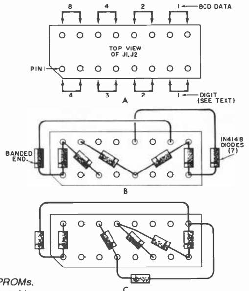
Fig. 9. How to program the diode-encoded PROMs. Use the truth table in the text as a guide. Diagram (B) is for FM; (C) is for AM receivers.
