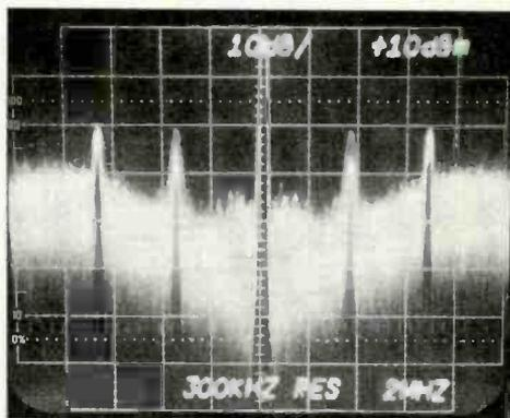
Fig. 3. Unfiltered carriers appear on either side of video reference.
