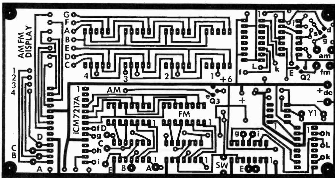
The FM prescaler board (Fig. 2) is installed inside the receiver and connected to the FM local oscillator. Otherwise, the long cables required to bring out the FM local-oscillator signal would detune the oscillator, making the FM section inoperative.
