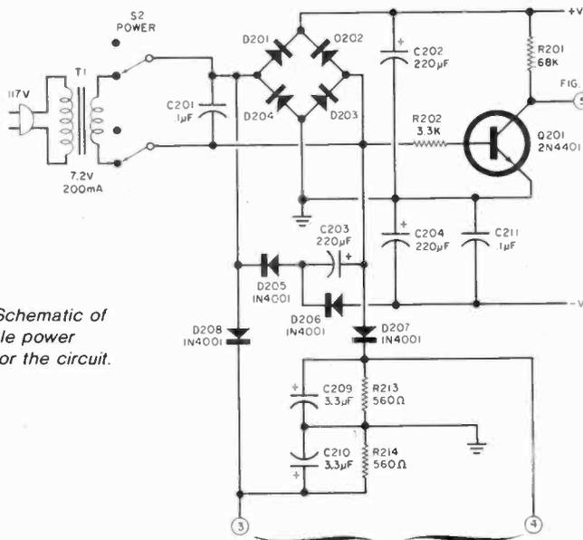
Fig. 3. Schematic of a suitable power supply for the circuit.
