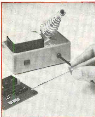
Wahl's new Model 7230 is designed for fine, heat-sensitive work. The 6-watt iron weighs 1/4 oz, and has 14 interchangeable tips from 0.04 to 0.16 inches. The tips are said to cool down quickly from 360°C and to resist seizure. Other features include a double-insulated transformer, a tip-cleaning sponge and sponge well, an indicator lamp, and an internal safety fuse. \$39.95.
