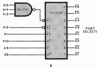
Fig. 9. Three ways to generate the port select signal: (A) with a NAND gate; (B) with a 1-of-8 decoder; and (C) with a comparator.
