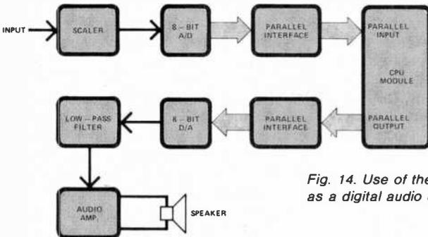
Fig. 14. Use of the CPU module as a digital audio delay line.
