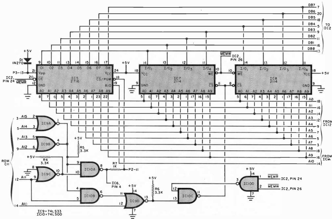
Fig. 6. Memory circuits contain the EPROM (IC5) and RAM composed of IC7 and IC8. Control logic is in IC9 and IC10.
