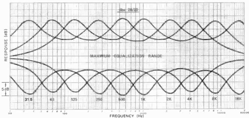
Fig. 1. Equalization filter curves for the dbx 20/20.
