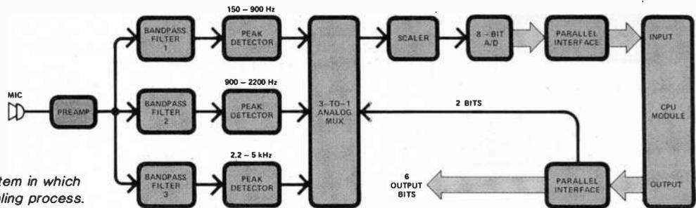
Fig. 15. A speech recognition system in which A/D conversion is used in a sampling process.
