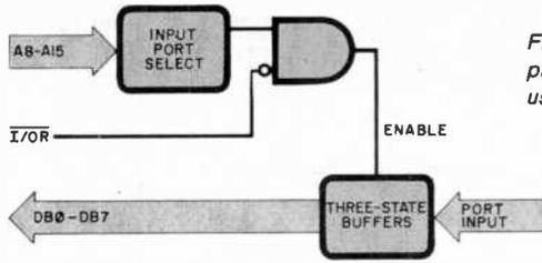
Fig. 10. Block diagram of parallel input interface using three-state buffers.
