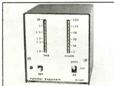
The new M-827 from Palomar Engineers is designed to compute standing wave ratios automatically and display them on a light bar. SWR reading is claimed to be accurate regardless of input power level (which is also displayed on a light bar adjacent to the SWR display). The M-827 has a frequency range rated at 1 to 30 MHz and power range of 20, 200, and 2000 W. The SWR scale is 1 to 10, with logarithmic response. \$98.
