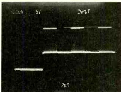
Fig. 5. Color-bar signal at the video input.
