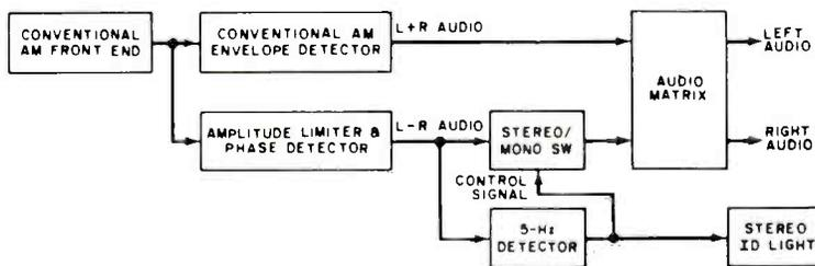
Fig. 4. Basic receiver configuration for Magnavox system.
