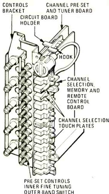
Fig. 1. A cut-away view of the tuning control.
