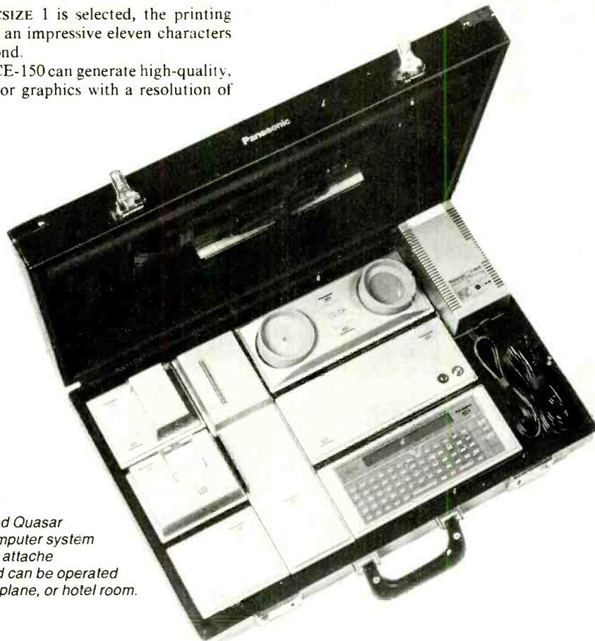
The fully expanded Quasar HHC computer system fits in an attache case and can be operated in a car, plane, or hotel room.
