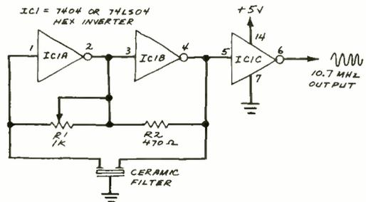
Fig. 6. Schematic diagram of a 10.7-MHz ceramic oscillator.
