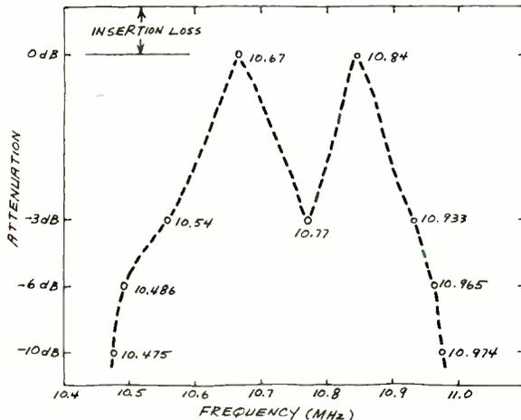
Fig. 5. Measured bandpass of a 10.7-MHz ceramic filter.
