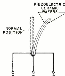
Fig. 2. Piezoelectric bimorph.
