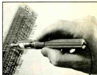
disturbing pins adjacent to the ones being tested. The Model 120-113 is rated for powered connections up to 600 V. It uses its own batteries to test unpowered connections. \$23. Address: Desco Industries, Inc., 761 Penarth Ave., Walnut, CA 91789.
