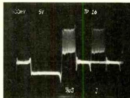
Fig. 6. Color-bar signal at first video amp.
