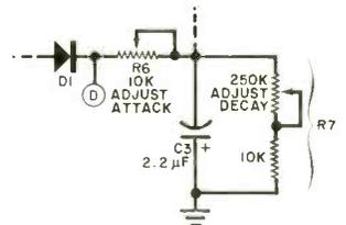
Fig. 5. Using pots for  $R6$  and  $R7$ .
