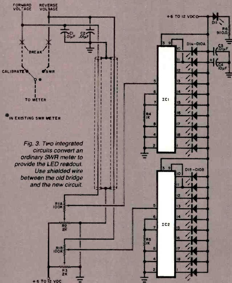
Fig. 3. Two integrated circuits convert an ordinary SWR meter to provide the LED readout. Use shielded wire between the old bridge and the new circuit.
