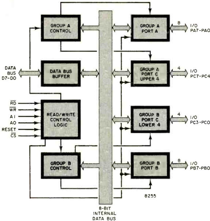
Fig. 4. Internal logic arrangement of the Intel 8255A.
