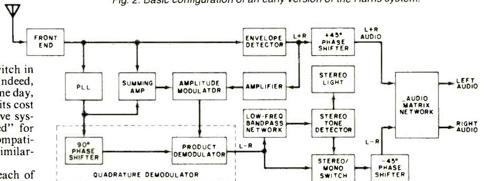
Fig. 3. Single-receiver diagram for Kahn/Hazeltine ISB system.
