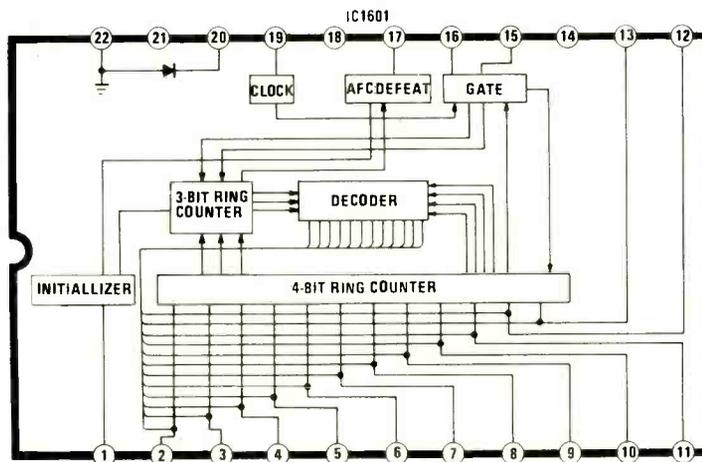
Fig. 2. The Mitsubishi IC1601 controls channel selection.
