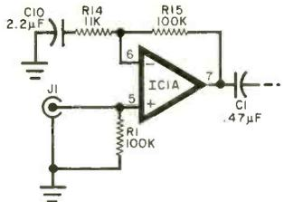
Fig. 4. First stage with gain of 10.
