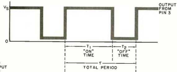
Fig. 2. Output of the circuit in Fig. 1, with characteristics defined.
