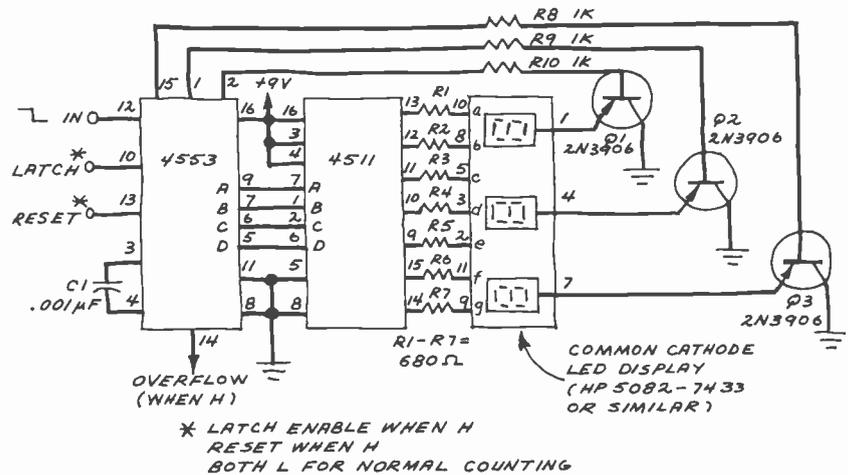
Fig. 1. Simplified block diagram of a 000-to-999 event counter.
