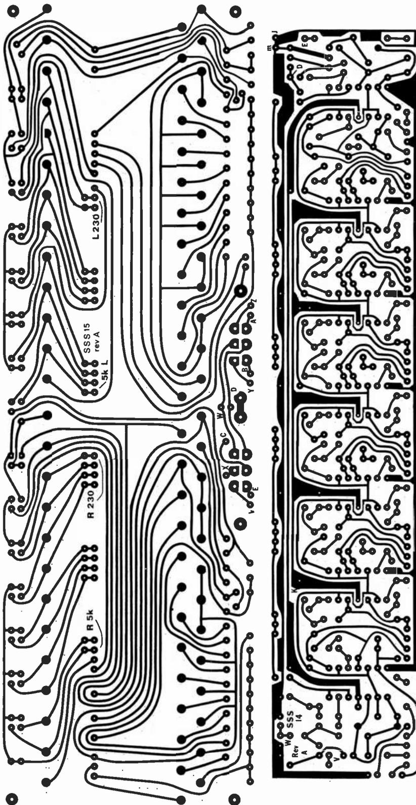
Fig. 3. Foil patterns for the Equalizer pc boards
