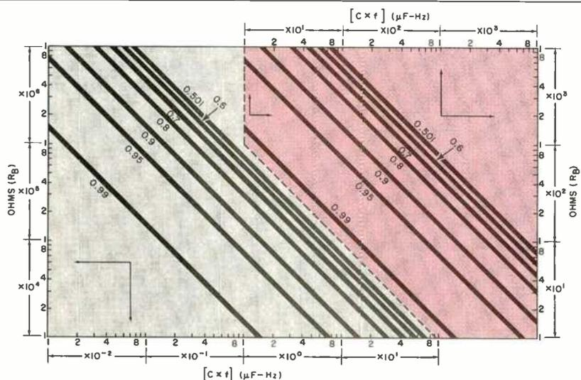
Fig. 3. Plot of  $C \times f$  vs.  $R_B$  which can be used with Fig. 4 to determine circuit values.
