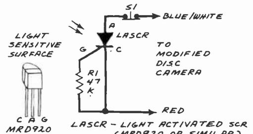
Fig. 3. Light-activated SCR trigger.
