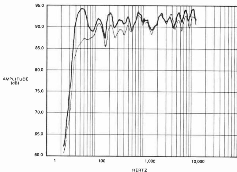
Fig. 6. Response of a standard car with (heavy line) and without a tuned enclosure.
