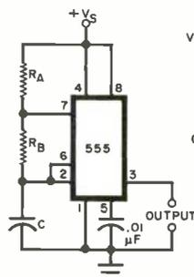
Fig. 1. Standard 555 square-wave generator.
