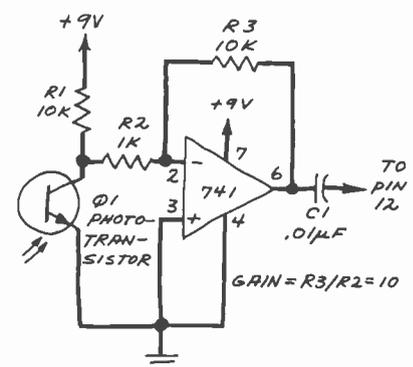
Fig. 3. Phototransistor gain stage for 3-digit event counter.
