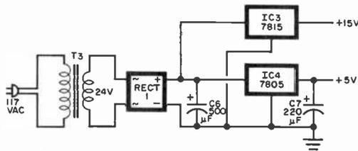
Fig. 3. Schematic of a suitable power supply.
