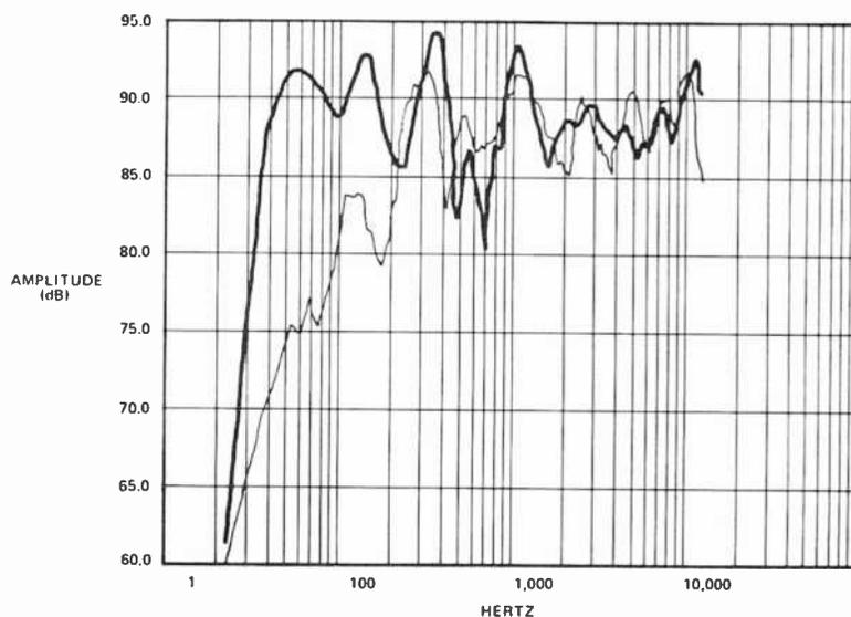
Fig. 7. Effect of a tuned enclosure (heavy line) in a compact car.
