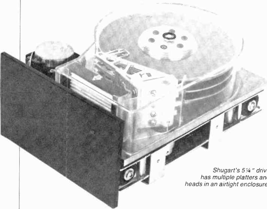
Shugart's 5 1/4" drive has multiple platters and heads in an airtight enclosure.
