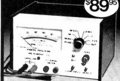
**Usefulness** — Measure capacitors 10pF — 500 $\mu$ F; leakage 1 nA or .005 C.V., whichever is greater. **Accuracy** — To 2% depending on range. **Dependability** — Ruggedized construction; 1 yr. warranty. **Versatility** — In circuit measurement of capacitance and leakage. Output signal proportionate to measurement. **Portability** — 350 Hr. Battery Life.
