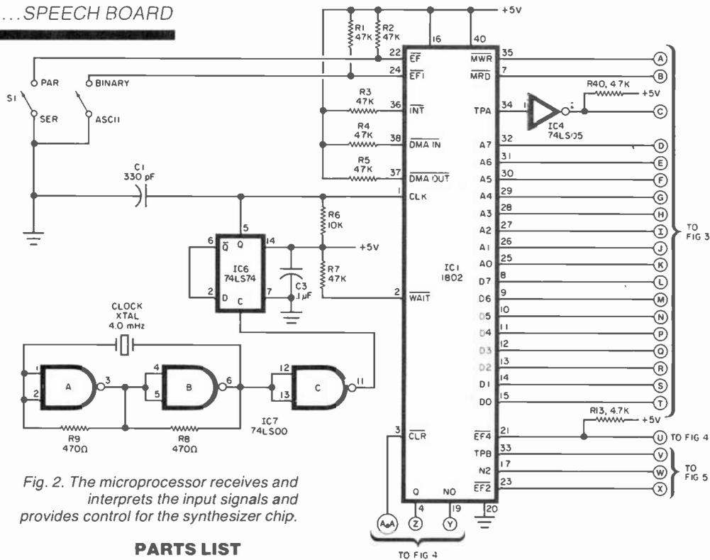
Fig. 2. The microprocessor receives and interprets the input signals and provides control for the synthesizer chip.
