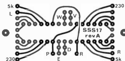
Fig. 5. Foil pattern for the connector board to the analyzer.
