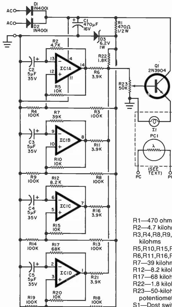
Fig. 2. Four square waves of different frequencies are generated in the four op amps and combined to produce the pseudo-random flicker voltage.
