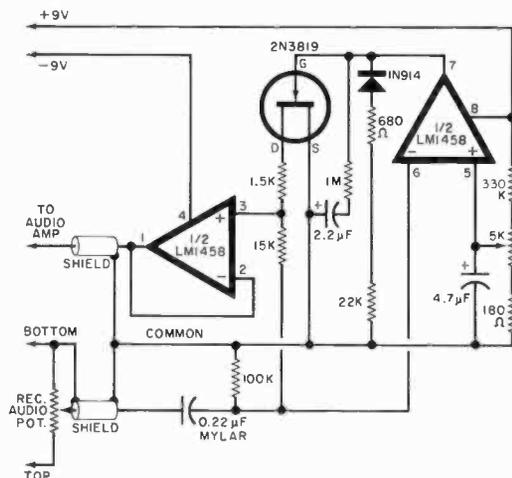
Changes were made to allow long-life battery operation. Since no input buffer, preamplifier, nor LED were required, a dual op amp was used instead of the quad op amp. The results are most promising—there is marked quieting for S/N ratios of 5 dB or more. In the presence of fading, however, the noise level pot has to be set to a value lower than the optimum.—*C. H. Harry, Bowie, MD.*
