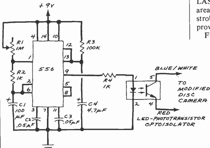
Fig. 2. Interval timer for disc camera
