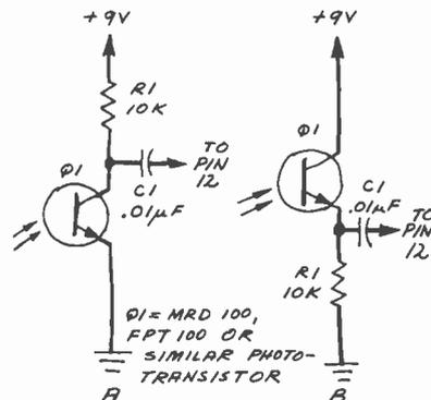
Fig. 2. Phototransistor inputs for 3-digit event counter.
