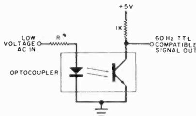
Some other nice features of the circuit are: 1) by connecting two of the above circuits to the same ac input with their diodes reversed, two signals 180° out of phase can be obtained; 2) if you use a neon-input optocoupler (Clairax makes many or a hobbyist could build one), the idea would work directly from the line and is isolated! It might be necessary to also insert a diode in series with the neon lamp or you'll get a 120-Hz output (desirable for some designs).
