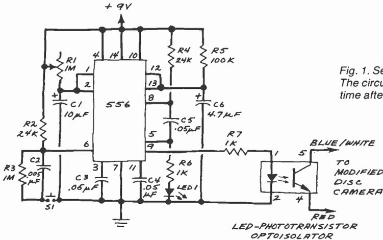
Fig. 1. Self timer for disc camera. The circuit triggers an adjustable time after *S1* is pressed and released.
