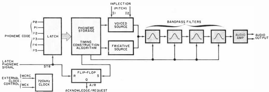
The Votrax SC-01 speech synthesizer chip used in this project is a phoneme type. It contains two voicing generators (voiced and fricative), four speech bandpass filters, a clock generator (710-kHz optimum), and a low-level audio amplifier. There are 64 stored phonemes in seven categories—the first six cover voiced, fricatives, and nasal sounds, while the seventh is silence.
