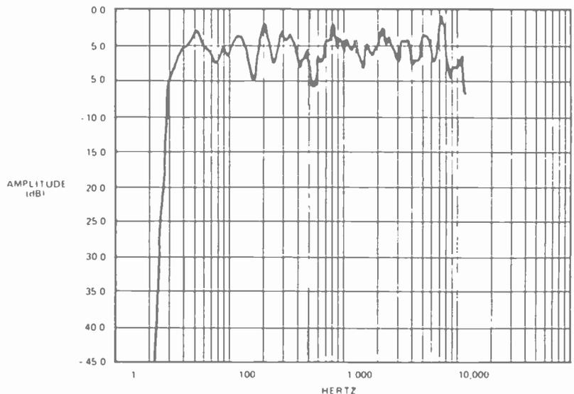
Fig. 5. Response of car with equalization applied.
