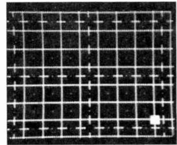
Electronically generated test pattern shows good linearity.
