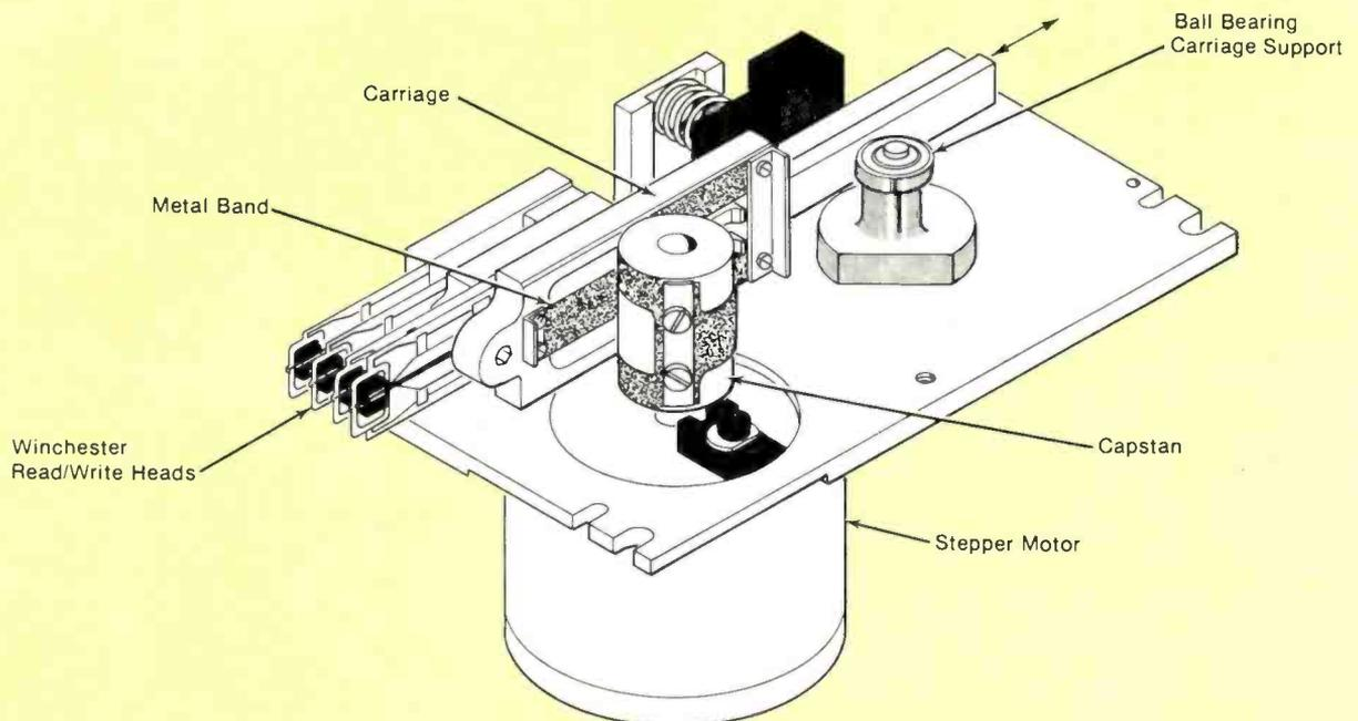
Fig. 2. Actuator assembly of the Shugart SA1000.
