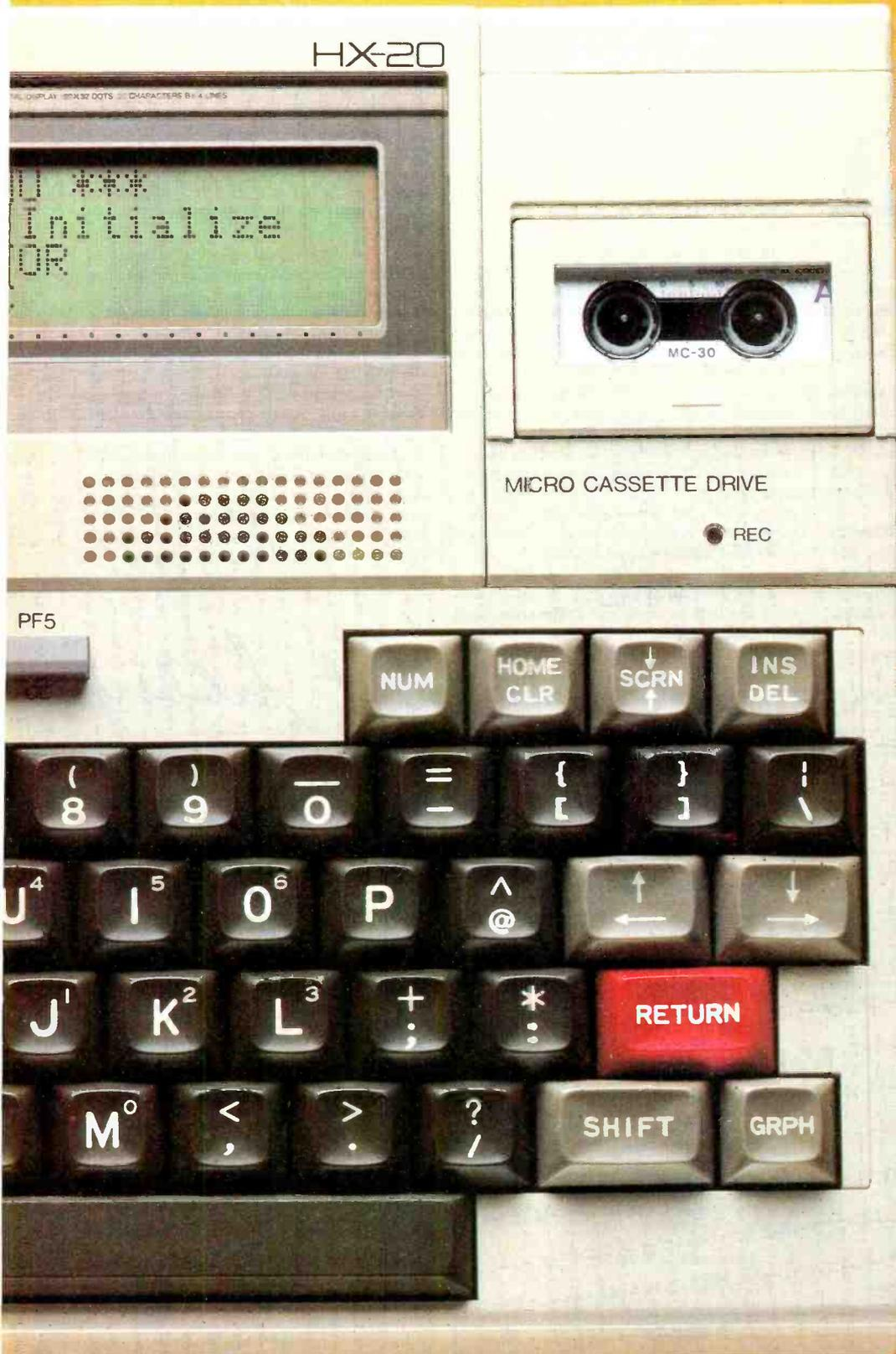
So with the HX-20, you can do programming, word processing and data entry just like you've got a big screen, up to 255 characters wide, with easy-to-read upper and lower case letters, numbers and punctuation and any 20 column by four line part of it visible by user command.
