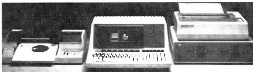
*Complete HP-87 system with plotter, disk drive and printer.*
