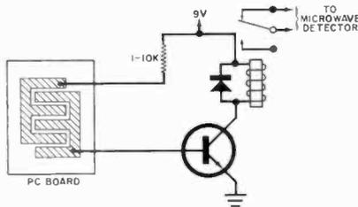
low. Connect the two wires to a pc board that has an interlaced pattern. Mount the board on an angle. When it rains, the wires will conduct, turn the transistor on, and energize the relay.
