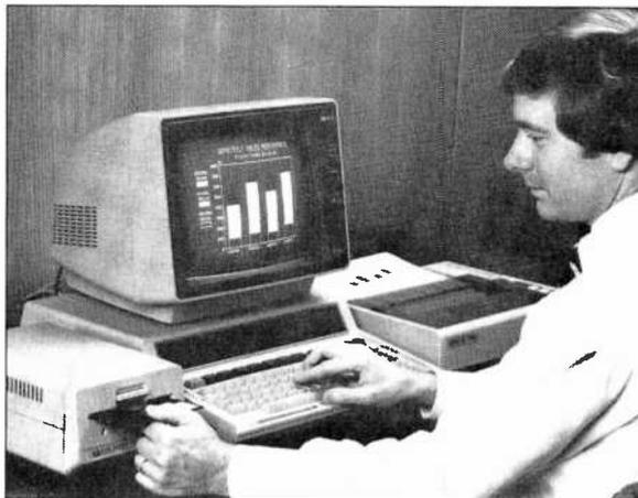
The HP-86 with a monitor, disk drive and printer.
