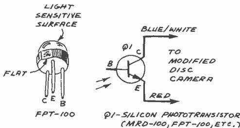
Fig. 4. Light-sensitive trigger for modified camera.
