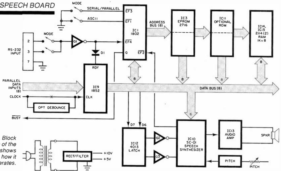
Fig. 1. Block diagram of the system shows how it operates.
