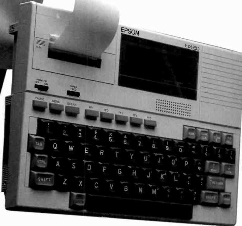
pared to the HP-75C's 10" × 5" × 1 1/4". But the HX-20 accounts for this most admirably by packing a microprinter and an optional micro-cassette drive or ROM program module easily into its rectangular face.
