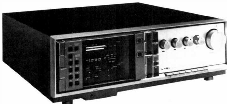
**T**HE Luxman RX-103 AM/FM stereo receiver has digitally synthesized AM and FM tuners and a rated audio output of 90 watts per channel into 8-ohm loads from 20 to 20,000 Hz with no more than 0.018% total harmonic distortion. It features a novel "Servo-Panel" that encloses the front-panel knobs when the set is off, and is retracted by a motor to expose them (together with some pushbutton controls) when it is turned on.
