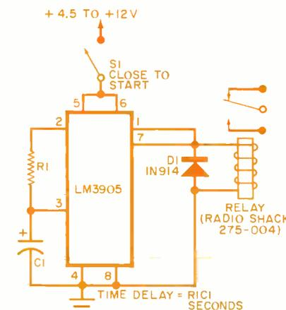
Fig. 12. Off-after-delay timer.
