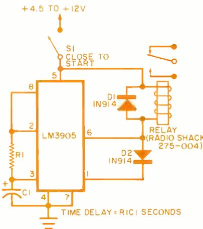
Fig. 11. On-after-delay timer.
