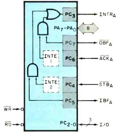
lines are used for a bidirectional bus and five lines for handshaking (borrowing one line from the other group).
