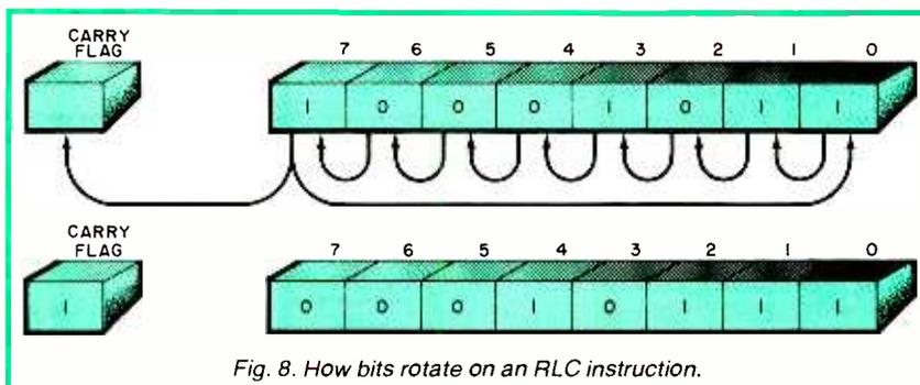
Fig. 8. How bits rotate on an RLC instruction.
