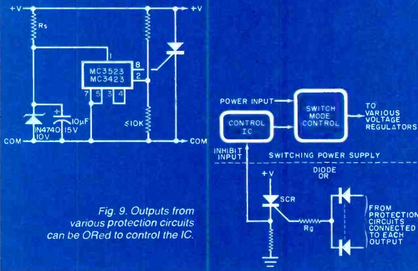
Fig. 9. Outputs from various protection circuits can be ORed to control the IC.
