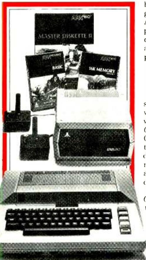
business accounting, play video games. Programmable in Basic or Assembly, the 800 can use all Atari peripherals and can control up to four disk drives and a 60 lpm printer. In all, the 800 and its accessories form a package worth a full \$1620 at retail!
