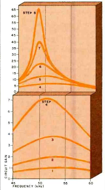
Fig. 4. First eight steps of receiver gain.
