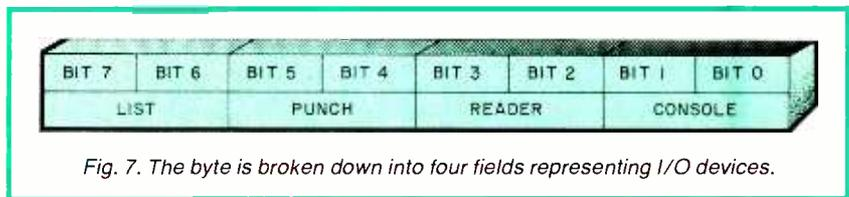
Fig. 7. The byte is broken down into four fields representing I/O devices.
