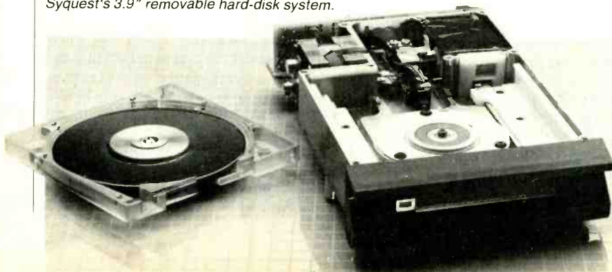
Syquest's 3.9" removable hard-disk system.
