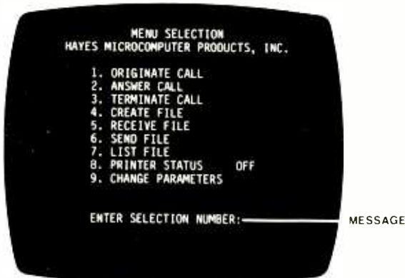
Fig. 2. When the system is ready and booted, the Hayes Terminal Program displays this menu.
