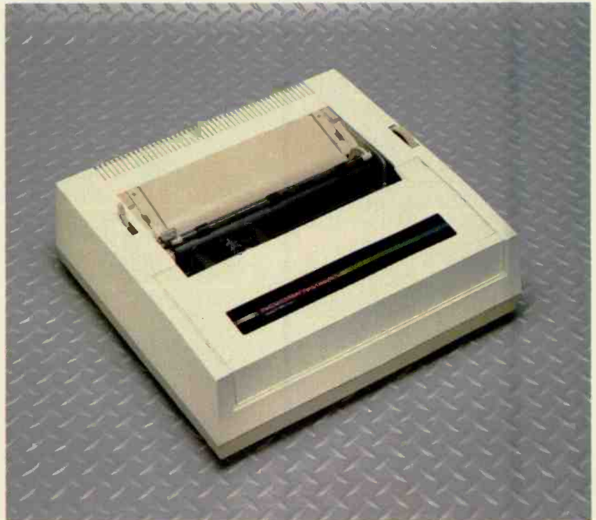
The daisy-wheel printer houses the system power supply.
