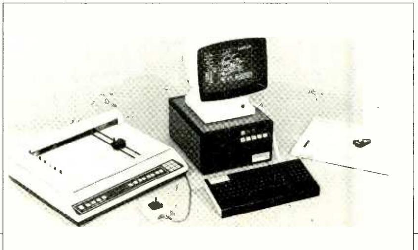
tion with an Apple II or IIe, the CAD-1 package sells for \$1095 and includes software, precision joystick controller and an interface module that plugs into the Apple's game port. CAD-1 will directly drive a Robographics plotter, and software drivers for other popular plotters can be obtained at prices ranging from \$250 to \$400.
