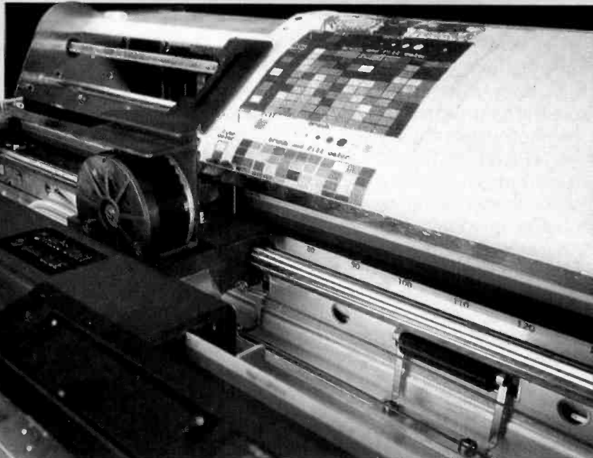
Shifting ribbon up or down on the Anadex 9725B brings different bands of colored ink into position before printhead.
