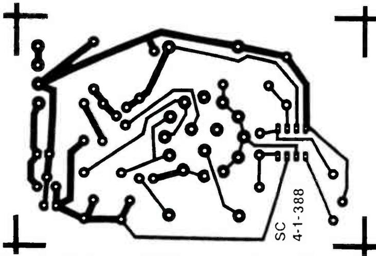
Fig. 2. If you are going to use a printed-circuit board for the Low-Ohms Adapter, as recommended, here is an appropriate full-size foil pattern.
