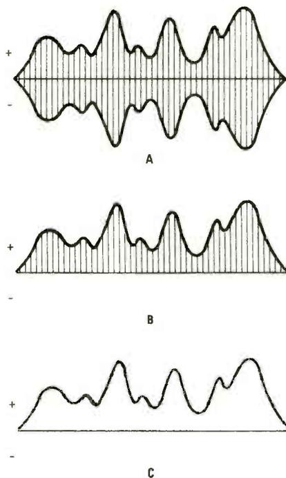
Fig. 1. The waveform in part "A" is a crude representation of an AM radio signal. Waveform B illustrates the rectification process, and C shows that the pulsations have been filtered out, resulting in a DC signal that varies in step with the original modulation.
