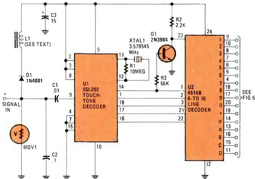
Fig. 4. The DTMF tone decoder (U1), which feeds a 4-bit signal to U2 (a 4- to 16-line decoder).
