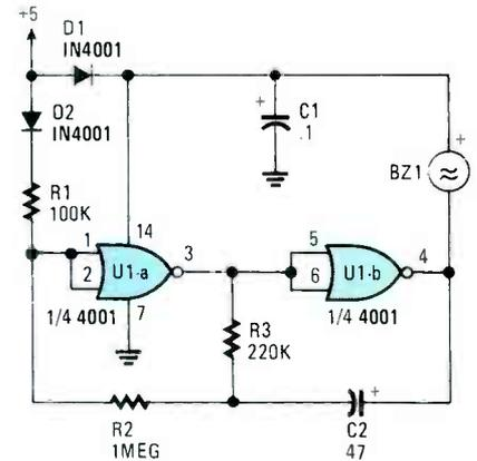
Fig. 4. The Thirty-Minute Electronic Virus does nothing as long as the equipment is in use. But when the power is turned off, the Virus sends out a beep every two seconds for about 30 minutes.
