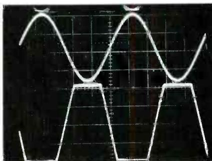
The vertical position controls can superimpose two signals for amplitude and phase comparison, (upper photo) or separate them for easy viewing.
