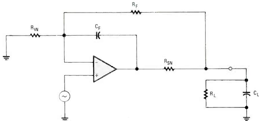
Fig. 7. Capacitor  $C_F$  rolls off the overall gain of the op-amp at high frequencies that are not within the desired frequency range. The snubber resistor ( $R_{SN}$ ) provides some isolation between the load and op-amp's internal driver amplifier.
