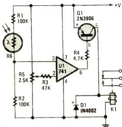
Fig. 6. The Dark Sensor is controlled by an LDR (light-dependant resistor).
