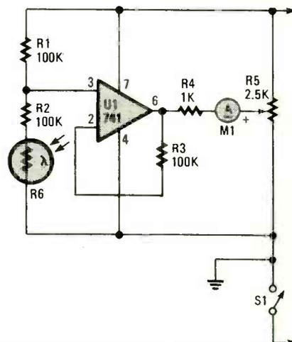
Fig. 5. The Enlarging Meter uses a light-dependent resistor mounted in a tube with a small hole at the end to allow light to enter.
