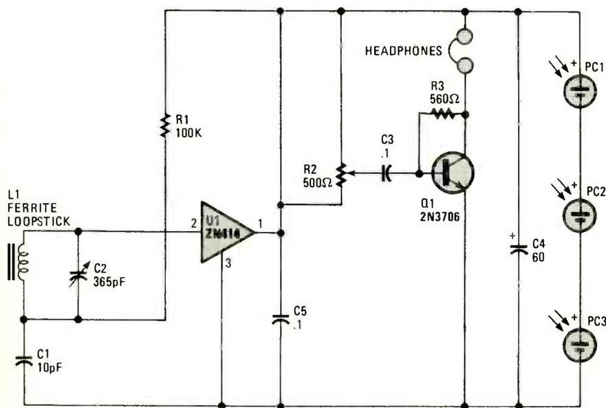
Fig. 4. Powered by sunlight or a bright lamp, the receiver is built around a ZN414.
