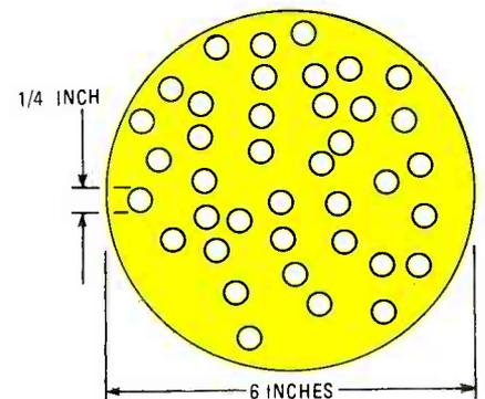
Fig. 5. A 6-inch diameter lid is fashioned from a piece of clear plexiglass. Quarter-inch holes are then drilled into the lid to help ventilate the lamp.
