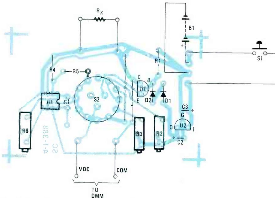
Fig. 3. Mount the components on the printed-circuit board using this parts-placement guide. Trim the shaft of switch S2 to a length of 3/8-in. before soldering it to the board, and don't forget the two wire jumpers on the board.
