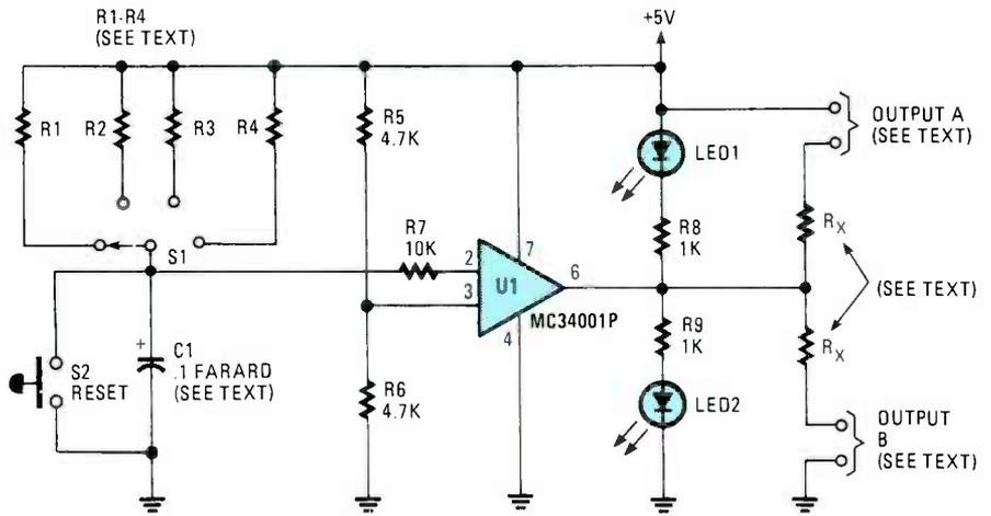
Fig. 3. This RC Timer, using a .1-farad capacitor, can provide time delays of up to one hour and 20 minutes.
