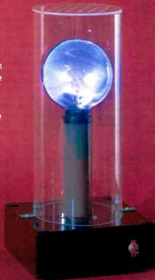
voltage power supply. The lamp is modified by taping a piece of aluminum foil to the back half of its glass envelope, forming a sort of make-shift capacitor. The electrode inside the lamp forms one plate of the capacitor, the glass envelope of the lamp serves as the dielectric, and the aluminum foil is used as the second plate.
