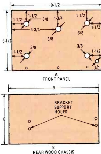
Fig. 3. Cut the front panel out of scrap Masonite and the back chassis from soft pinewood. Drill all holes in the front panel before spraying both sides with black enamel paint.
