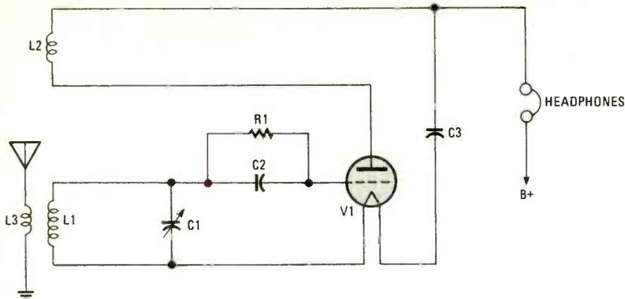
Fig. 2. This rather simplified generic schematic diagram, which is representative of one-tube regenerative sets, helps to illustrate the operation of grid-leak detectors.
