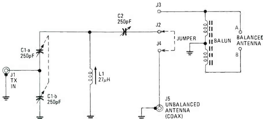
Fig. 1. The TM-1000 broadband antenna-tuning unit that works over the range 1.8 to 30 MHz, at power levels up to 1,000-watts, and suppresses harmonics of the operating frequency, while offering less than 0.5 dB insertion loss.
