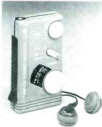
The blue and yellow receiver measures only 1.7 x 3.3 inches, and runs on one AAA battery. The AM/FM-stereo reception offers clear sound; built-in automatic frequency control reduces station drift. There are no external antennas to get in the way. The FM antenna is built into the headphone cord and the AM antenna is built into the receiver.
