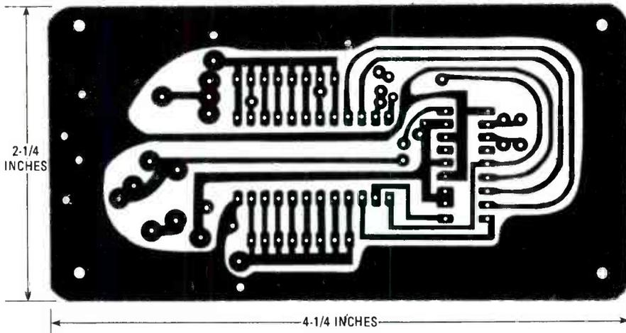
Fig. 6. Here is a full-scale template of the DTMF Field Phone's printed circuit board.
