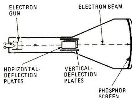
*Fig. 1. Once a beam of electrons is generated by the electron gun, the deflection plates deflect the beam in the vertical and horizontal directions to trace patterns on the screen.*
