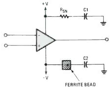
Fig. 6. To eliminate the unfortunate effect that ceramic-disc capacitors have at high frequencies, snubber resistors ( $R_{SN}$  in A) and ferrite beads (B) are used.
