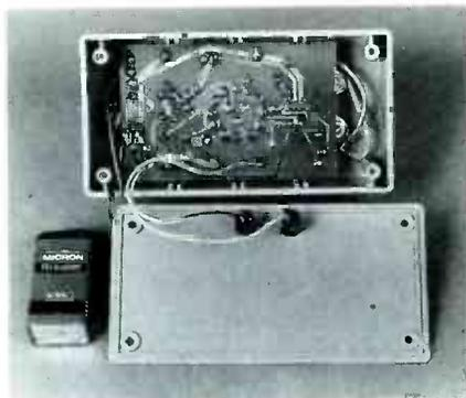
The completed Low-Ohms Adapter is shown here just prior to buttoning up. The battery will bounce around in the box if stuffing or two-sided tape is not used.
