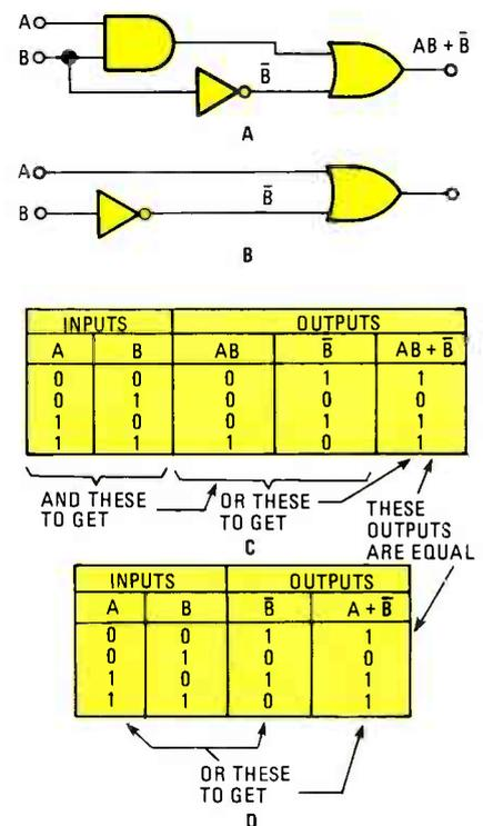
Fig. 9. Obviously, the circuit in B is easier than the one in A. To prove their equivalence you can compare the outputs of their truth tables given in C and D.
