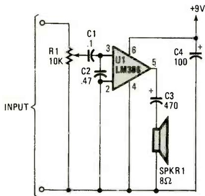
Fig. 3. The Speaker Amplifier is designed to plug into the earphone jack of Walkman-type receivers and provide enough power to drive external speakers.
