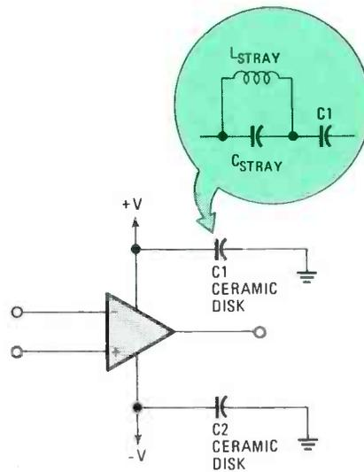
Fig. 5. Ceramic-disc capacitors can be your undoing when they are used to decouple the power supply from the circuit. The equivalent circuit for that capacitor is in the inset.
