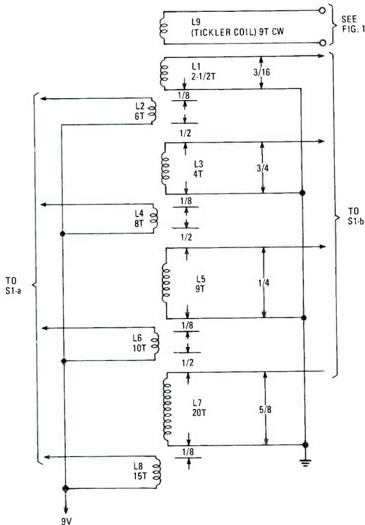
Fig. 2. Here are the coils- with turn, size, and spacing information. All coils are wound with number 24 enameled wire.
