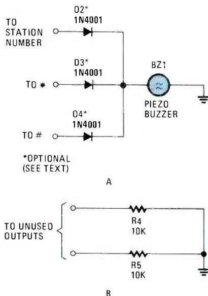
Fig. 5. If more than one output is to be used, diodes (as shown in A) should be connected between the chosen outputs and the buzzer. Unused outputs are routed to ground (as shown in B) through resistors R4 and R5.
