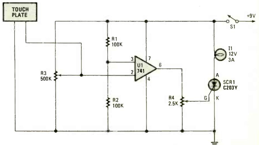
Fig. 1. The input from the touch-plate is fed to the inverting input of U1, which delivers a sufficient current to trigger SCR1.
