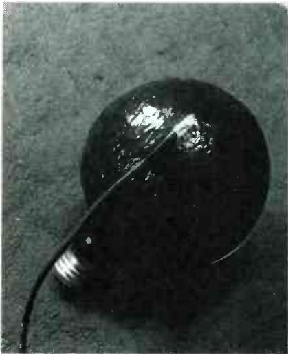
When applying the second layer of tape, leave a small area of aluminum exposed, and connect a wire to the foil.
