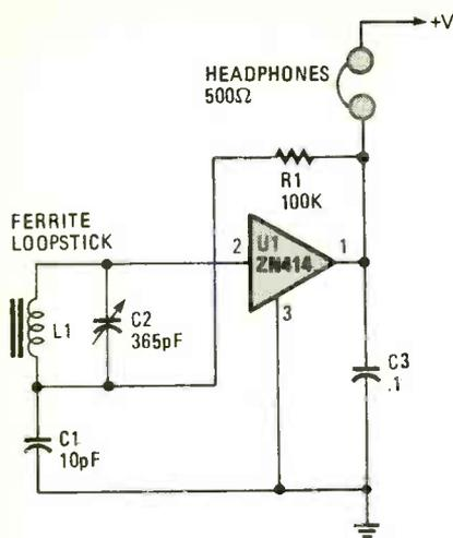
Fig. 2. In this circuit, L1 (a ferrite loopstick) serves as the antenna, which is tuned by variable capacitor C2.
