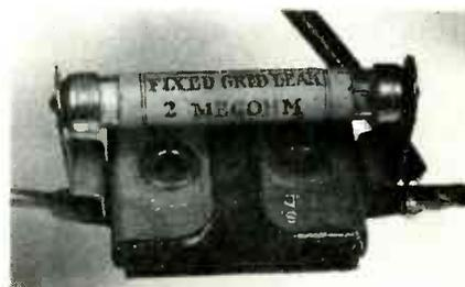
Here's a close-up of the Crosley's grid-leak detector assembly. The resistance unit looks a lot like a small fuse. It snaps into a couple of spring clips mounted directly on the grid capacitor.
