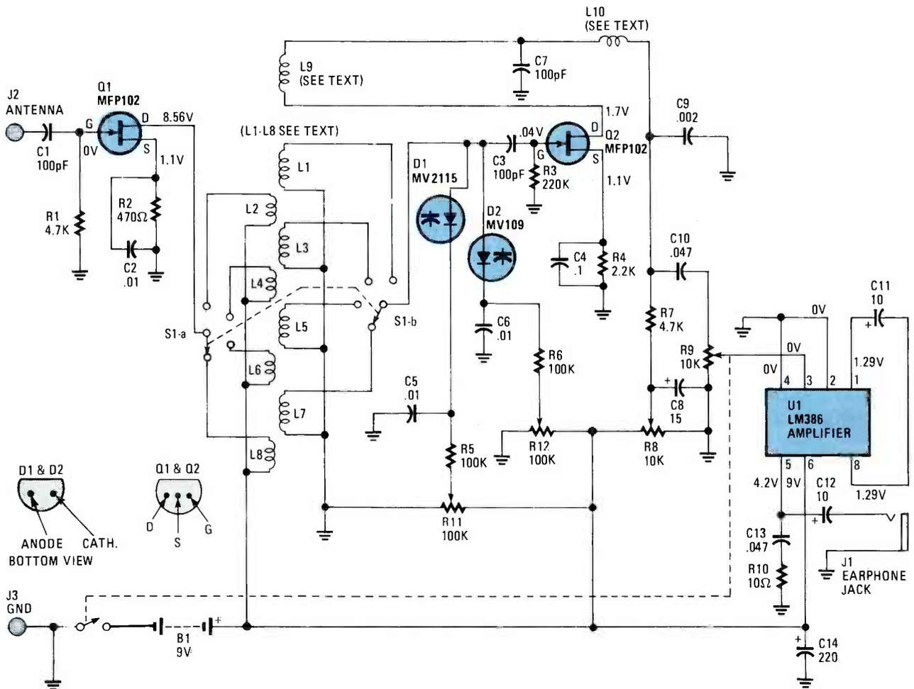
Fig. 1. Distant shortwave stations can be pulled in with two RF transistors (Q1 and Q2), and the often used audio IC (LM386). Here is the main schematic.
