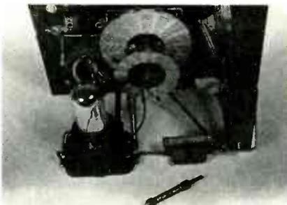
A look behind the Crosley 50 panel shows the grid-leak detector assembly just to the right of the tube socket. Below that is an Eagle adjustable grid-leak resistor of the same era. Its value could be changed by twisting a knurled thumbscrew on one end.
