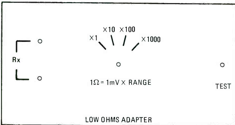
Fig. 4. This front-panel artwork can be used as a drilling template for the front panel provided the printed-circuit board and cabinet are of the sizes specified. If not, a little more layout designing will be required on your part.
