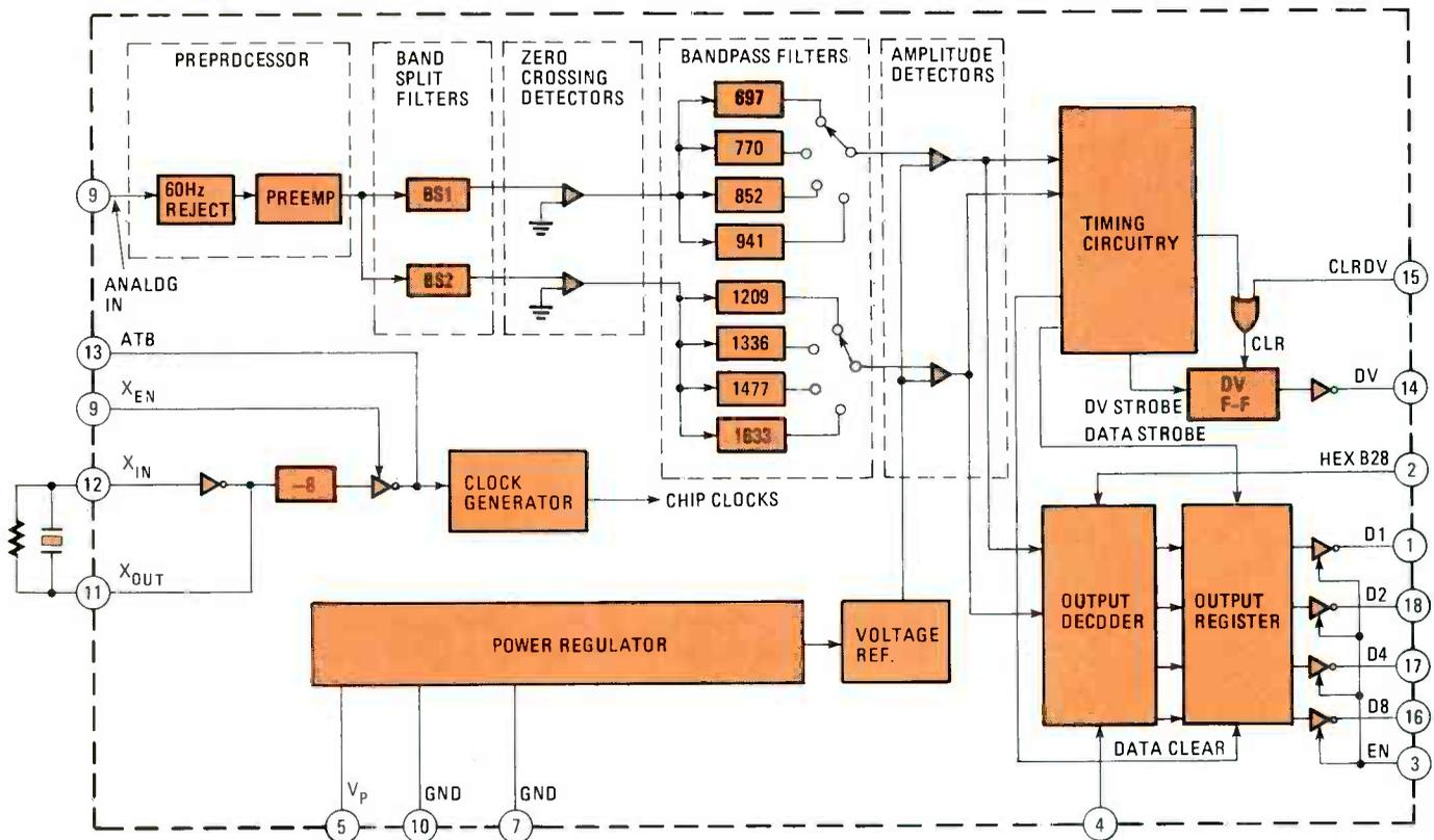
Fig. 3. This is a functional block diagram of the SSI-202 DTMF (dual-tone multi-frequency) decoder, which is the heart of the DTMF Field Phone circuit.
