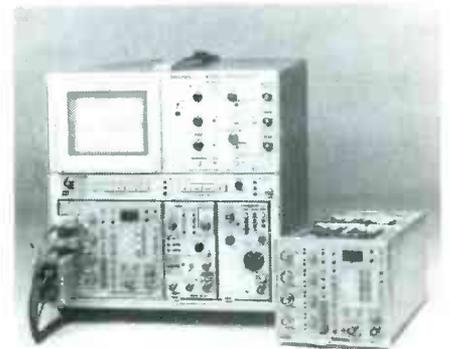
Super-colossal units, like this Tektronix, have plug-in modules (on the right) for specific applications.
