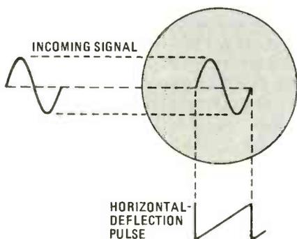
Fig. 2. If an input signal is applied across the vertical plates while a synchronized sawtooth controls the horizontal deflection, then the electron beam will trace the input signal on the CRT screen while it is swept by the sawtooth.
