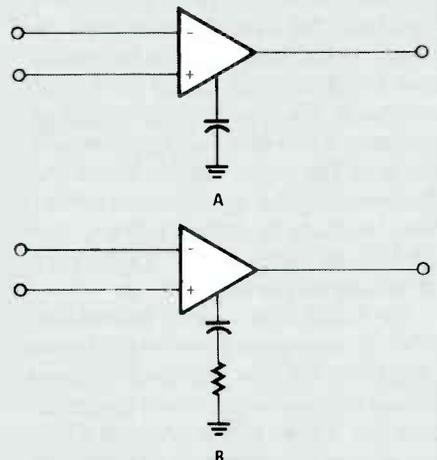
Fig. 3. Another method of reducing oscillation is called lag compensation. In that technique, one of the op-amp's compensation terminals is connected to ground using a capacitor (A) or an RC network (B).
