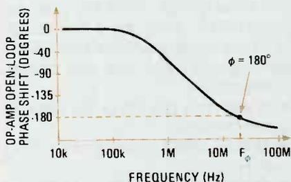
Fig. 1. This graph tells the story of how an innocent op-amp operating at low frequencies can produce parasitic oscillations beyond its frequency range.
