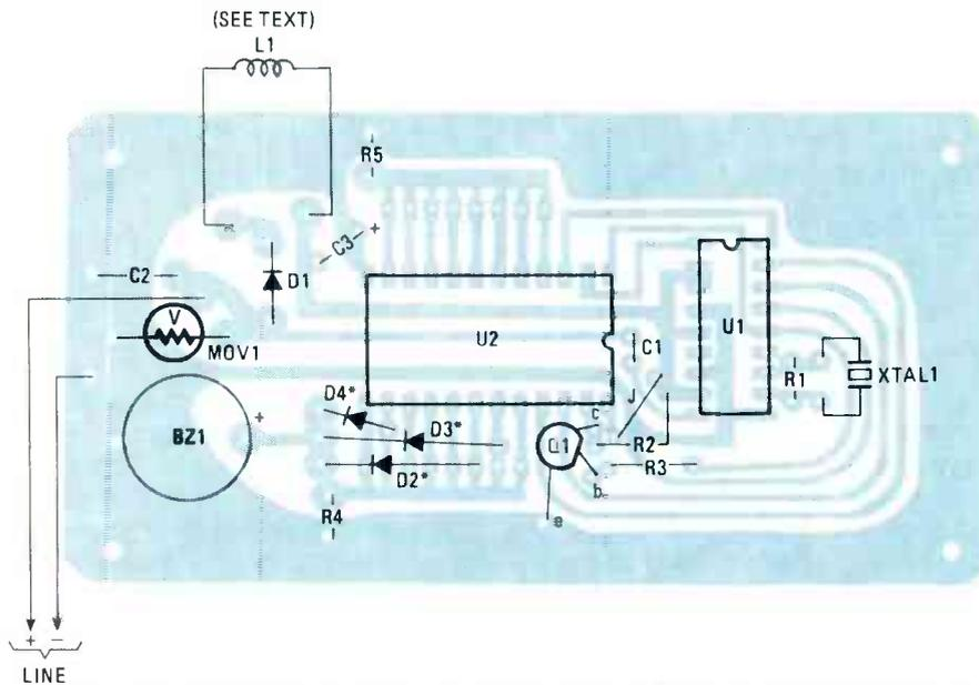
Fig. 7. Here is the parts-placement diagram for the DTMF Field Phone's decoder circuit. Cut the appropriate traces for the number to which the station is to respond. As for the unused outputs, the traces should be left as they are.
