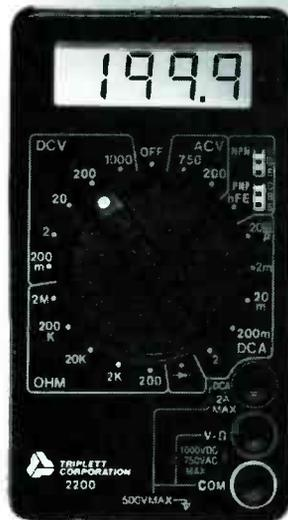
measures from 200-millivolts to 1000-volts DC in 5 ranges; from 200 volts to 750 volts AC in two ranges; 200-microamps to 2-amps DC in 5 ranges; 200 ohms to 2 megohms in two ranges; and diode-test and FE measurements.
