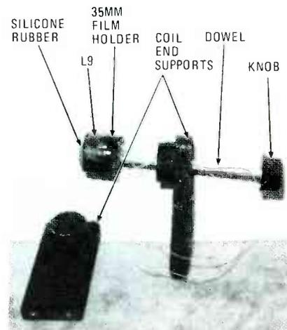
The tickler coil is wound with 9 turns of number 24 enameled wire over a 35-mm film container. Any 1-inch form will do. The container is cemented to a  $\frac{1}{4}$ -inch dowel rod for feedback operation.
