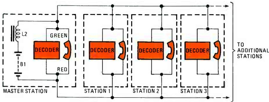
Fig. 1. Here is a block diagram of the field phone system, which is powered by a single battery that is located at the master station.
