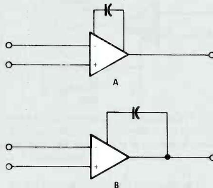
Fig. 2. In lead compensation, a small-value capacitor can be used to reduce the op-amp gain at frequencies where unwanted oscillations occur. Two different methods of lead compensation are shown here.
