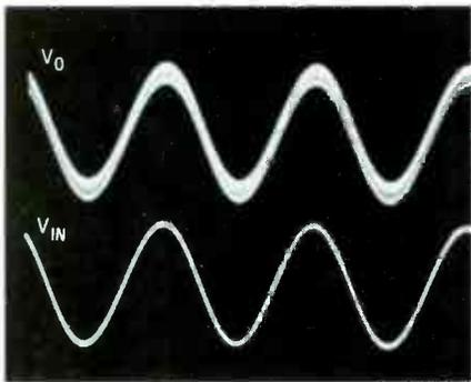
Fig. 4. Note the instability in the output signal of this op-amp circuit. The problem was remedied by adding decoupling capacitors to the circuit's DC power supply.
