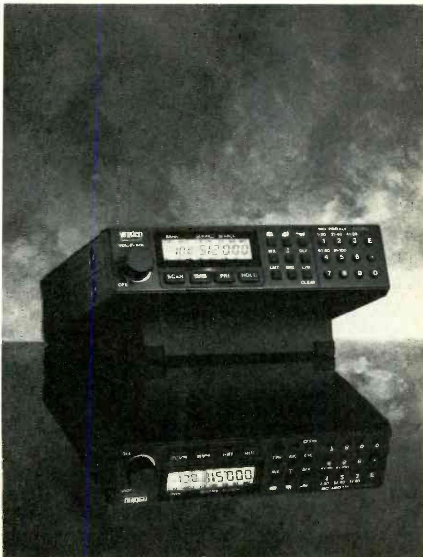
*The Uniden Bearcat 950XLT has 100-channels divided into five banks of twenty each and features an optional CTCSS PL (selective calling) decoder board and something called "Service Scan," in addition to all of the usual scanner features.*
