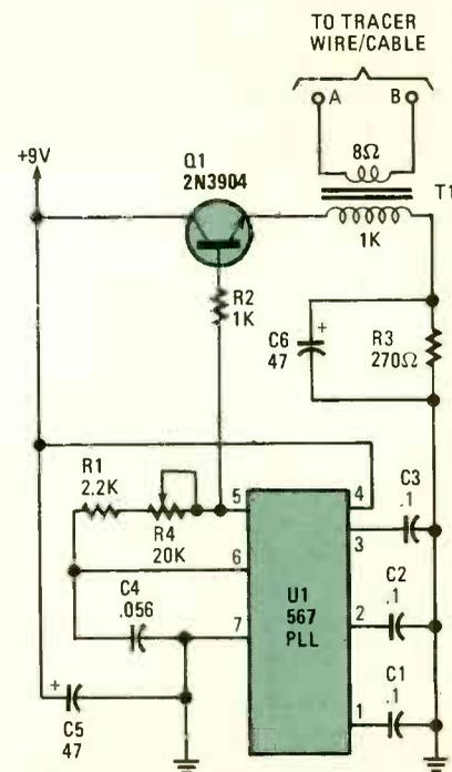
Fig. 2. The Closed-Loop Tracer is designed to follow an induced voltage path that's created by feeding a low current, audio-frequency signal through the cable.
