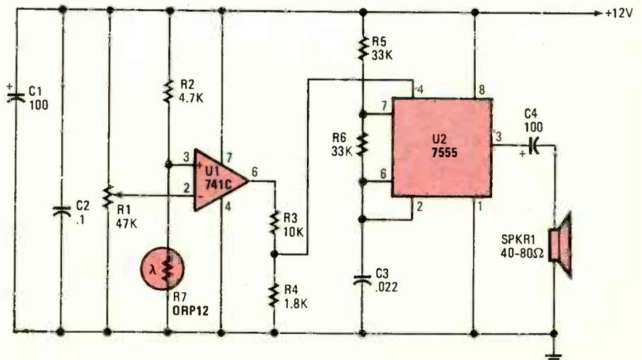
Fig. 1. The Lights-On Reminder sounds an audible alarm when the ambient light level falls below a certain point.
