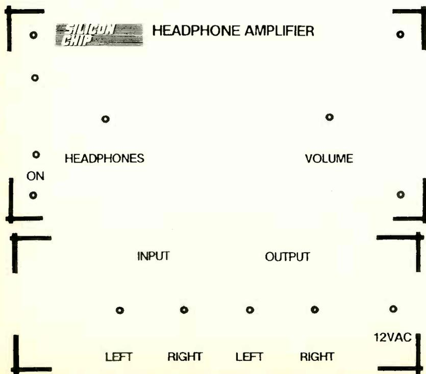
Fig. 4. This is a template of the author's front- and rear-panel layouts.
