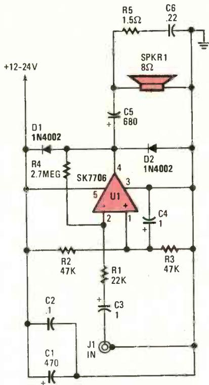
Fig. 2. The Practice Amp has a power output of under two watts.
