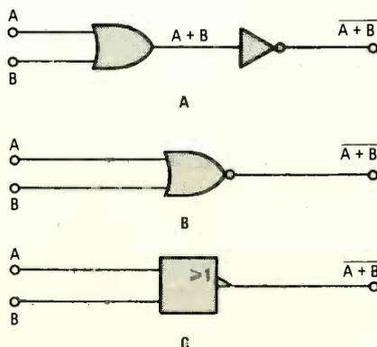
Fig. 4. An OR with a NOT gate output (A) forms a NOR gate (B), which has a special symbol as shown in C.
