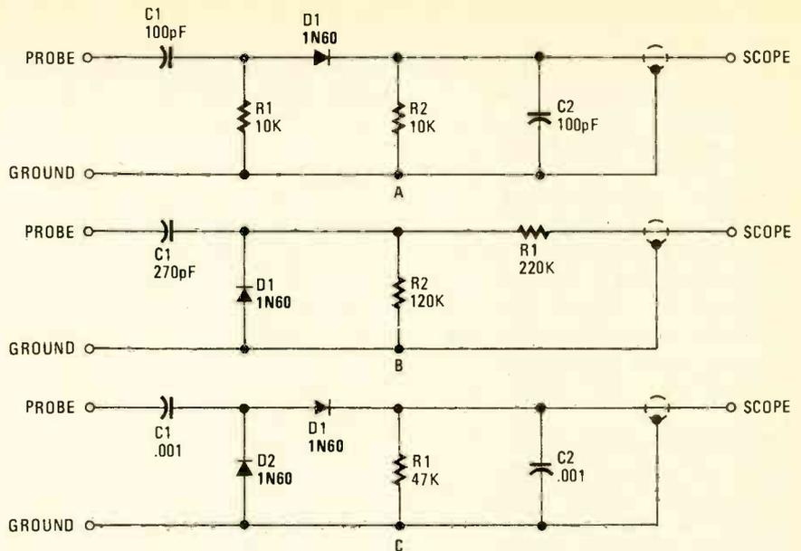
Fig. 7. The demodulator probe shown in A uses a series detector. The capacitor values shown are typical but not right for all applications. A shunt detector version of the probe is shown in A voltage-doubler version is shown in C.
