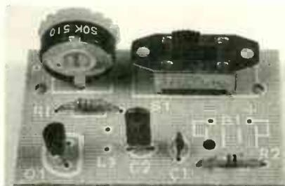
Mounting holes are drilled in the board before any components were installed. Be careful when drilling the holes, so as not to sever the copper traces.
