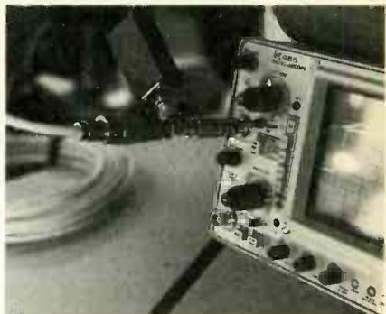
When making RF measurements, adapters should be mounted as close as possible to an oscilloscope. Note how that is accomplished with a "tee" connector.
