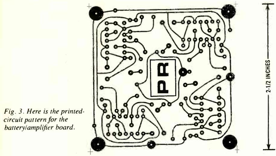
Fig. 3. Here is the printed-circuit pattern for the battery/amplifier board.
