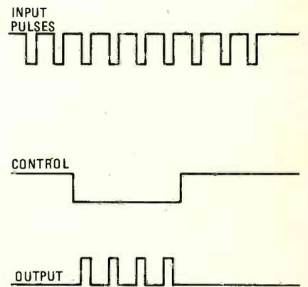
*Fig. 7. A negative NAND gate can be used to control the flow of pulses. One input receives the input pulses, and the other a control signal. When the control goes low, the inverted input signal appears at the output as shown.*
