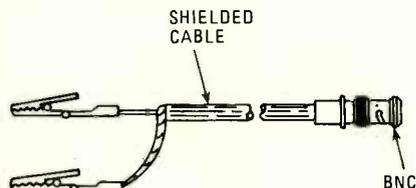
Fig. 4. This is the most basic form of oscilloscope probe. That probe works well for signals with frequencies below RF. In the RF region the cable capacitance starts to cause roll off.
