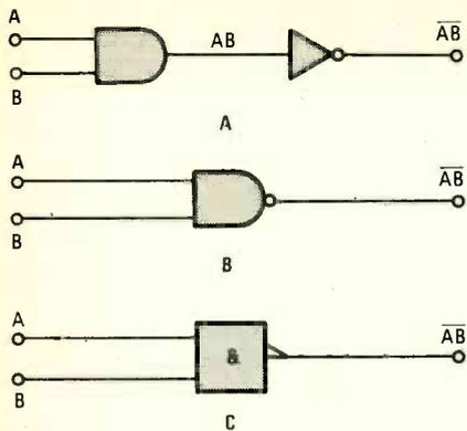
Fig. 2. An AND and NOT gate combined (A) is really a NAND gate (B), which has a special symbol shown in C.
