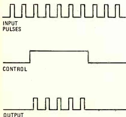
*Fig. 6. Any AND gate can be used to control the flow of input pulses. One input is used to accept input pulses, and the other a control signal. If the control goes high, the input signal appears at the output as shown.*
