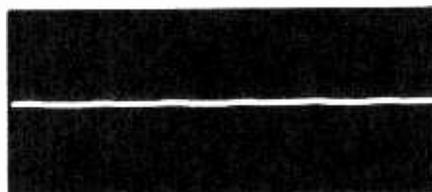
Fig. 11. Even at .1 V/division the ripple of a regulated power supply is hard to see. The nasty ripple tamed by the regulator can be seen in Fig. 10.
