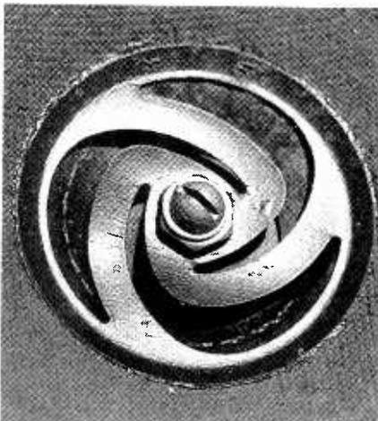
The "spider" at the center of old speaker cones acts as a damper on cone movement and holds the voice coil centered in the gap. If the voice coil is fouling the magnet, the cone can be repositioned by temporarily loosening the screw.
