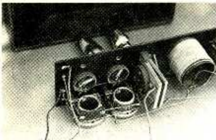
Interior shot of Model VI gives us a good look at the famous Crosley "book-style" tuning capacitor. Fixed RF coil (right) suggests set isn't regenerative.
