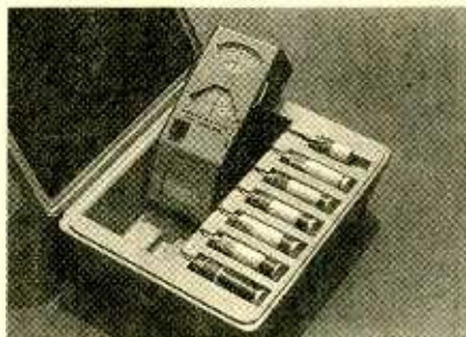
This Heath dip meter comes with a variety of coils so that it can cover a wide frequency range. Although you have to build it yourself, if done properly it is a quality instrument.
