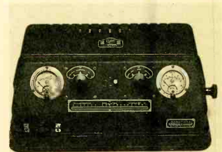
This antiquated medical generator was manufactured by the H.G. Fisher Company of Chicago, Illinois. The rotary switch on the left allows selection of alternating current, "galvanic" current, or a "combination" of the two. The device is made of cast iron.
