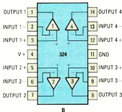
Fig. 6. In this circuit (A), the voltages that are to be compared are derived from typical voltage-divider networks: R1 and R3 for the inverting inputs; and the R2/R4 and R6/R5 combinations, for the non-inverting inputs. Shown in B is the pinout diagram for the 324 quad op-amp.
