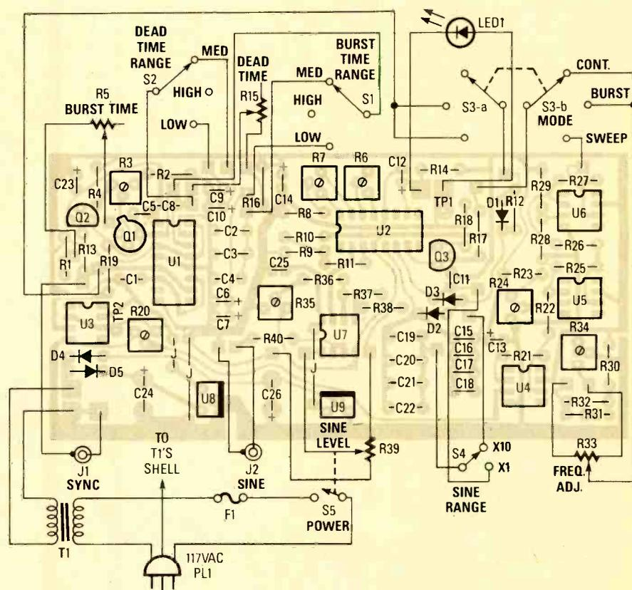
Fig. 3. Here is the parts-placement diagram for the foil pattern shown in Fig. 2. The wise way to begin assembly is to install IC sockets at the appropriate locations on the board, and then use the sockets as reference points to the proper positions for the other board-mounted components.
