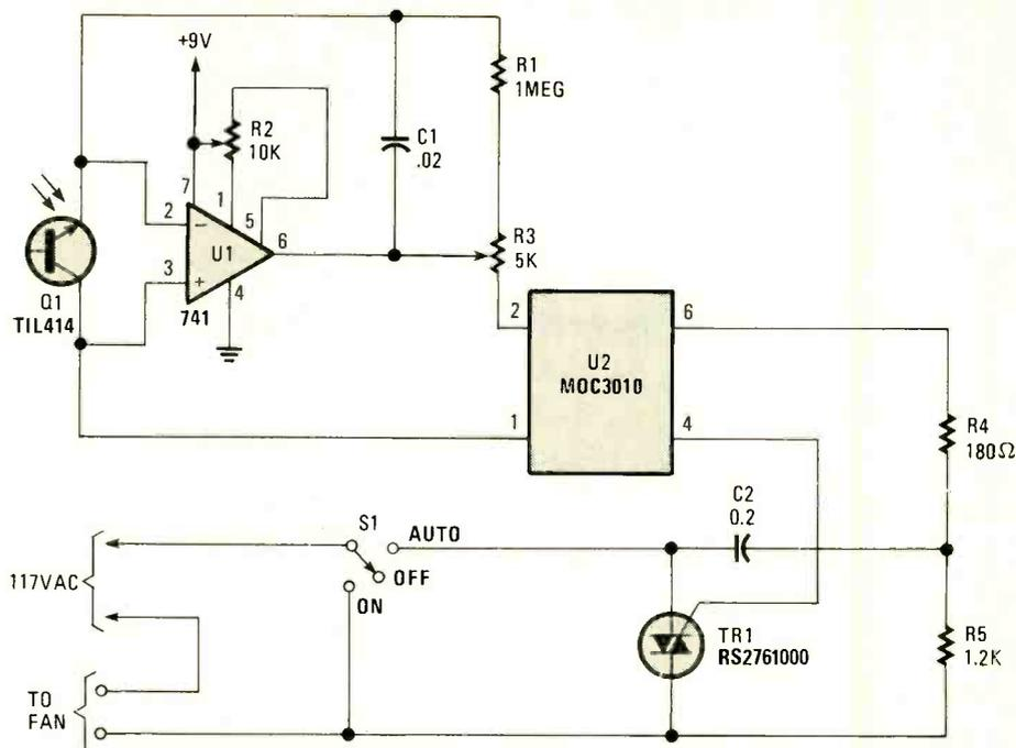
Fig. 2. This simple IR control circuit is designed to activate a kitchen exhaust fan under pre-defined conditions.
