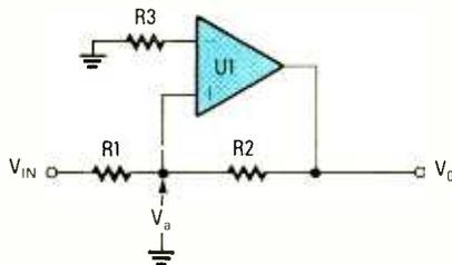
Fig. 4. Single-ended comparators with hysteresis are also possible.
