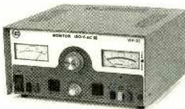
comes with two 3<sup>1</sup>/<sub>2</sub>-inch meters. One meter monitors line or output voltage and the other can be used to display output current or leakage. For safety, the units' metal cases are connected to the power-line ground through the three-conductor AC-power cord. The AC input is separately fused.
