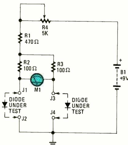
Fig. 2. If a more-dynamic testing approach is desired, try this modified version of the previous matching circuit. The main difference between the two circuits is the addition of a variable resistor, R4, which allows you to vary the current through the diodes.
