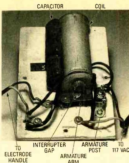
*Here's a restored generator circuit. Use as much fresh hardware as possible. The screws going into the compartment lid should be fairly short; long ones will go straight through and damage the outer surface.*
