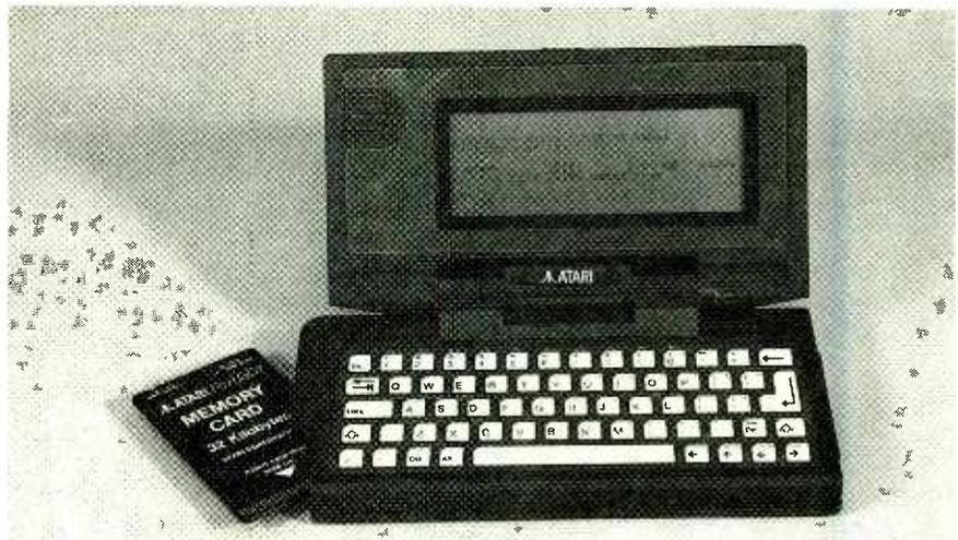
*Sophisticated micro-miniaturization technology was used to make the Atari a one-pound unit, which is slightly smaller than a video-tape cassette. The thin memory card snaps into a side port. Note the piano-key-like contacts at the bottom of the card.*
