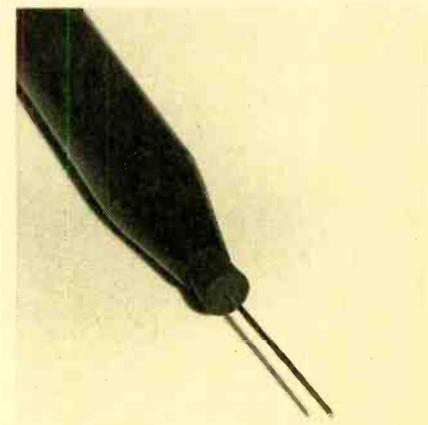
*Push the loop into the barrel, fit the stopper down over the wire, and your probe is done.*
