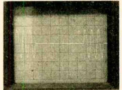
The Audio Sweep/Burst Generator can produce many signal patterns; shown here is a sine-wave burst followed by a dead-time period, which is followed by another burst.
