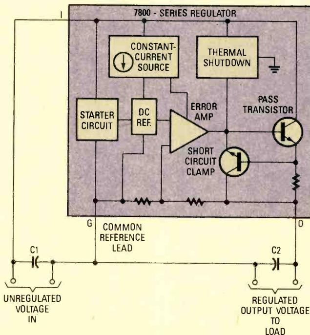
Fig. 5. This block diagram of a typical TTR doesn't really give one the feel for the level of complexity normally found in such devices.
