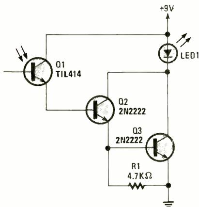
Fig. 7. The IR Remote Checker consist of little more than an infrared-sensitive phototransistor, and a pair of general-purpose transistors connected in a Darlington configuration, to provide sufficient drive to light LED1 (a visible light unit).
