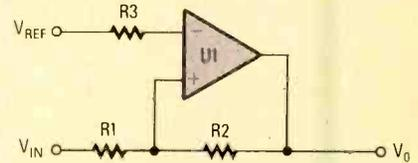
Fig. 3. In situations where the input signal is a slowly varying voltage, comparators with hysteresis—which would give a "snap action" to the output—are desirable.
