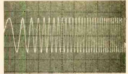
An expanded view of the frequency-sweep signal output by the Audio Sweep/Burst Generator. The signal starts (left) at a relatively low frequency (left), and increases at a rate determined by the operator, as the generator's output is swept through the audio spectrum.
