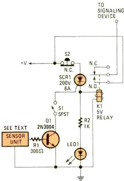
Fig. 4. At the heart of the Automated Entry Alarm circuit is a sensor (All Electronics Corp. part LSMD) that detects changes in ambient light and/or motion.
