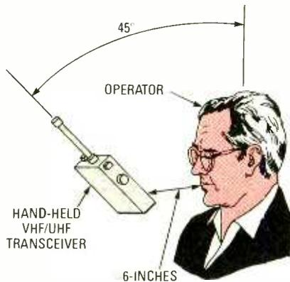
Fig. 2. When operating a handheld VHF/UHF transceiver, keep the unit at least six inches from your face and cocked at a 45° angle.
