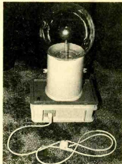
One of the author's many plasma displays. This one features a 6-liter flask and a metal ball-shaped electrode, and is filled with neon at a pressure of 70 mm Hg.
