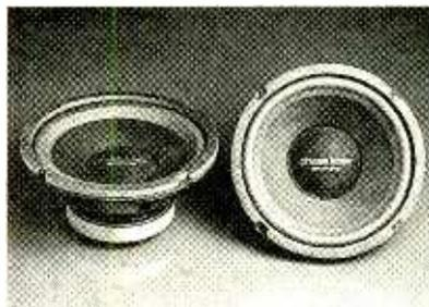
response is 20 Hz – 2.5 kHz, its efficiency is 93 dB (1 watt, 1 meter), and its impedance is 4 ohms. The *PLS1200* can accommodate crossover settings up to 200 Hz. The subwoofer features a hefty 40-ounce magnet with a bottom-load mounting depth of 148 mm and a top-load mounting depth of 135 mm.
