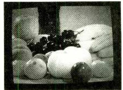
Fig. 2. Even at fringe-area signal levels (100 $\mu$ V), only a slight increase in background noise is evident.
