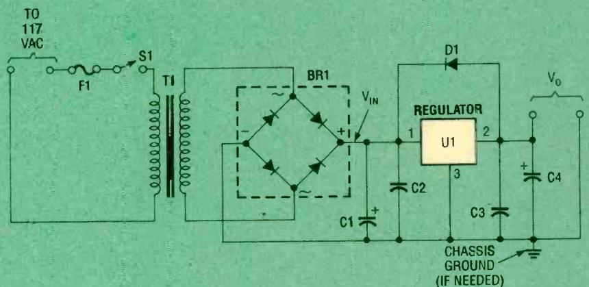
Fig. 2. This is a standard circuit for using a three-terminal voltage regulator. Note that D1 will dissipate the charge on C<sub>4</sub> when the supply is shut down.
