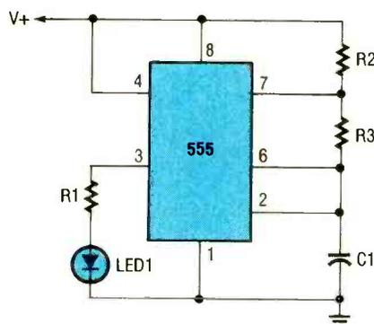
Fig. 1. When operated in the astable mode, the voltage on C1 oscillates between  $\frac{1}{3}V_{CC}$  (the internally set upper threshold level) and  $\frac{2}{3}V_{CC}$  (the internally set lower threshold level) as long as power is applied to the circuit.
