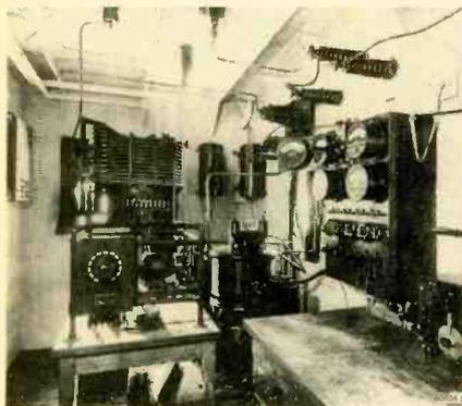
This Navy 5-kW shipboard arc transmitter/receiver station operated on a frequency from 100 to 250 kHz.
