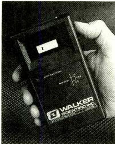
its 10-segment LED will illuminate to indicate the level of radiation present.
