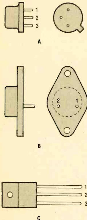
Fig. 3. Here are the most common package styles for voltage regulators. From top to bottom they are: (A) the "H" package (for up to 100 mA); (B) the "K" package (for 1 ampere maximum); and (C) the "T" package (to provide 750 mA).
