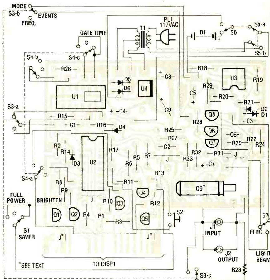
Fig. 3. When assembling the counter, first install IC sockets at the positions indicated for U1, U2, and U3, then the jumper connections and passive components (resistors, capacitors, etc.), followed by the semiconductor devices (diodes, transistors); do not install the IC's until the initial checkout has been performed.
