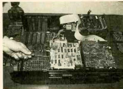
*To remove the diskette drive, unscrew the two mounting fasteners, either on the left side of drive A or on the right side of drive B. To remove the drive A screws, you will have to remove the nearby adapter cards first.*
