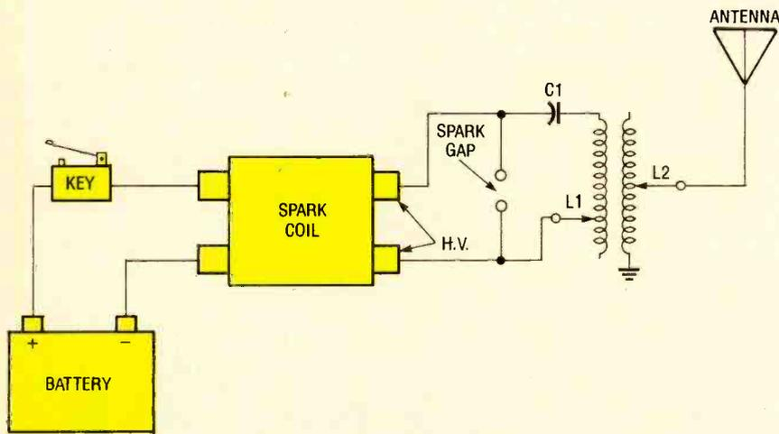
*Fig. 1. One of the earliest practical spark-gap transmitters used by experimenters and amateur-radio operators was this spark-coil design. Spark coils are high-voltage transformers, usually encased in wood or some other insulating material, that incorporate a vibrator or interrupter switch in the primary circuit.*
