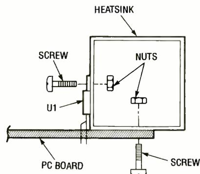
Fig. 5. Before you solder U1 in place, attach the heatsink as shown, so that the pre-drilled hole in the heatsink lines up with the one in U1.
