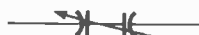
Fig. 9. This is the schematic symbol for split-stator capacitors. They often find application in antenna tuners.
