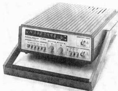
×20 input attenuator and low pass filter. Suggested applications range from general audio to amateur and business radio, cordless-phone repairs, rotational measurement, and tuning transmitters in the keyed state. Suitable for both bench and field use, the FC130A is useful for research and development, troubleshooting and repair, and equipment calibration.
