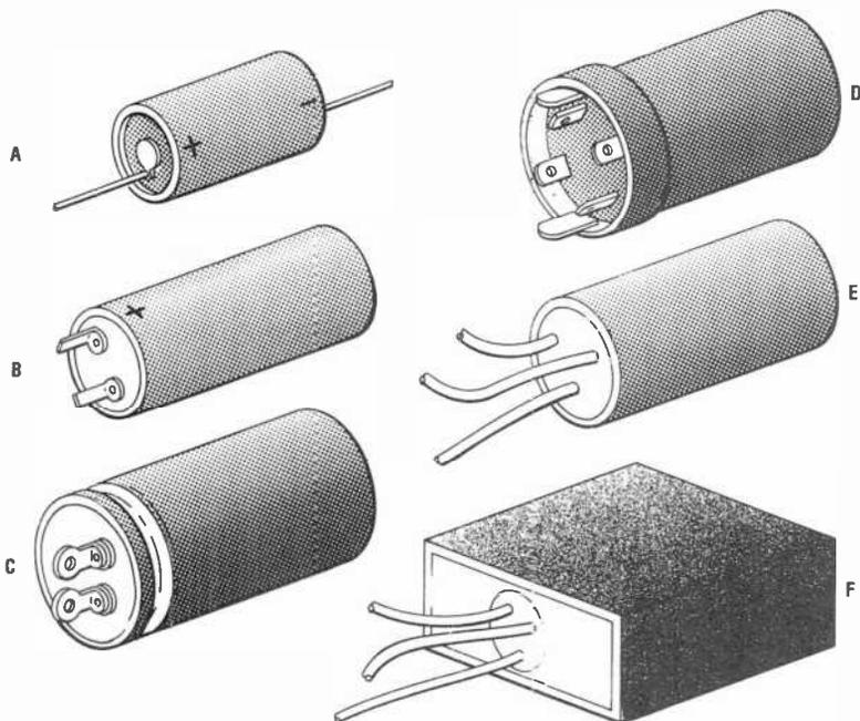
Fig. 5. These are various forms of aluminum-electrolyte capacitors: A) single-section tubular (axial leads); B) radial lead single-section tubular; C) Large value single-section; D) chassis mounted; E) multi-section tubular; and F) archaic "tubular" or "box" capacitor.
