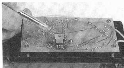
The printed-circuit board is secured to the case lid using machine screws, washers and tapped 1/2-inch spacers. Note that the 3-terminal regulator is soldered to the foil side of the board
