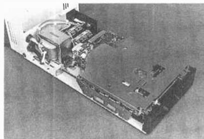
*This completely assembled 5-1/4-inch half-height floppy-disk drive is shown with the lid removed from its JMR 1SV5 case to reveal its power supply toward the unit's rear.*
