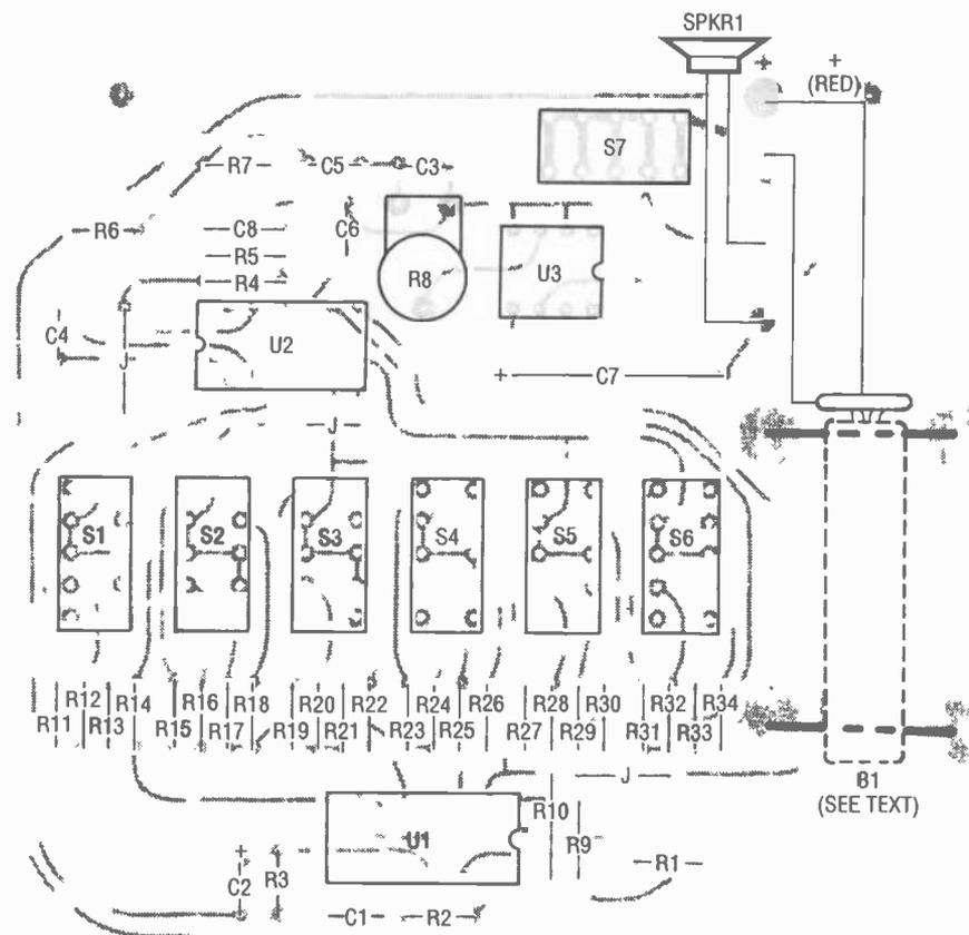
Fig. 3. Once you've collected the necessary parts, assemble the circuit using this parts-placement diagram as a guide. Note: The nine-volt transistor radio battery is not mounted to the component side of the board, but instead is held to the foil side of the board with wire brackets.
