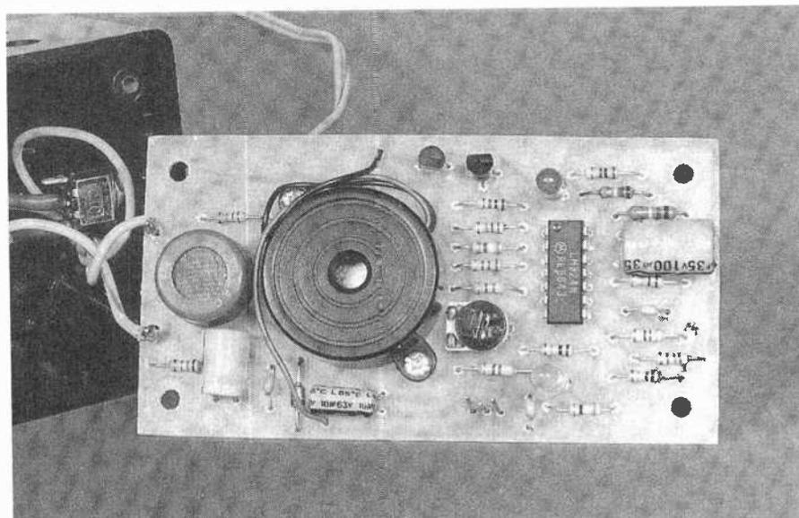
The three electrolytic capacitors are mounted horizontally on the printed-circuit board so that they clear the front panel. Note that the TGS 822 must be installed so that the top of the sensor is level with the piezo alarm.
