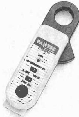
meter readings require either a 100-mV DC voltage range or a 1-volt DC voltage range. The clamp-on adapter requires a 9-volt battery source; an LED low-battery indicator is built-in. The CTA-600 is equipped with standard banana-jack outputs. It has a minimum load impedance of 40 Kohm/V and an operating temperature range from 0–40°C.
