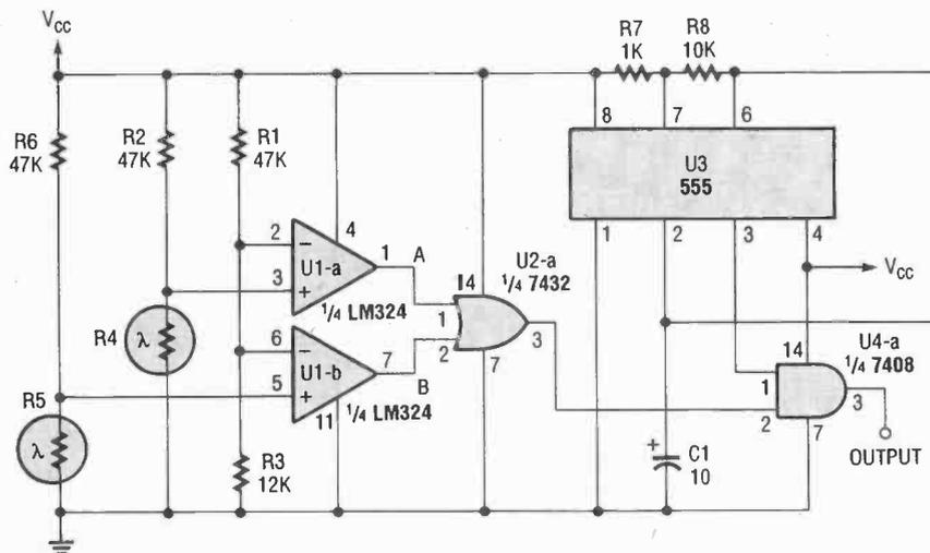
Fig. 1. Our sequential logic circuit consists of three familiar sub-circuits, with a few additions, which you should recognize: U2-a,  $\frac{1}{4}$  of a 7432 quad 2-input OR gate; U4-a,  $\frac{1}{4}$  of a 7408 quad 2-input AND gate; and a 555 oscillator.
