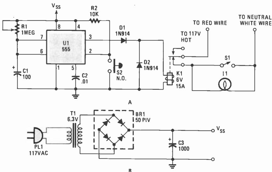
Fig. 2. The Universal Timer can be configured for makelbreak operation by connecting a second circuit to be controlled between the center and upper contacts of K1.
