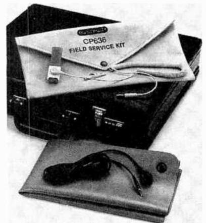
dissipative vinyl work surface, an elastic wristband, and two grounding cords. The 0.030-inch-thick work surface measures 18 x 22 inches and provides a surface resistivity of  $10^9$  ohms/sq.
