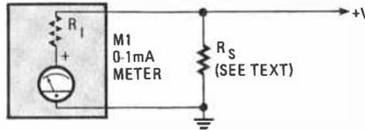
Fig. 5. In cases where the shunt resistance is very small, a length of wire can be wound to function as a resistor.
