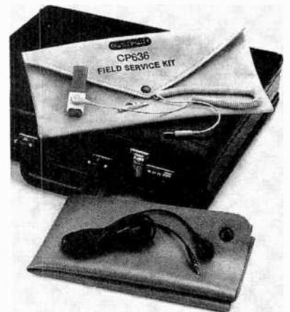
dissipative vinyl work surface, an elastic wristband, and two grounding cords. The 0.030-inch-thick work surface measures 18 x 22 inches and provides a surface resistivity of  $10^9$  ohms/sq.
