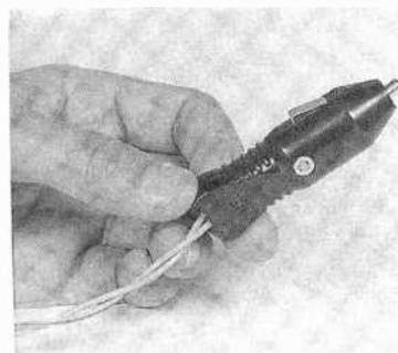
By wiring the power leads to a cigarette lighter plug, you can easily move the unit from vehicle to vehicle.
