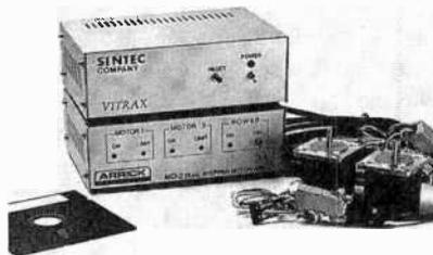
robotic arms, X-Y tables, telescopes, conveyors, and automatic-production equipment. The stepper-motor driver package is also available without the microcontroller, for programming directly from a PC.
