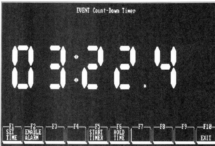
The event count-down timer screen is shown set for 3 hours and 22.4 minutes. Beeps that mark the seconds can be toggled on/off and a sound alarm option can be used to alert a nearby user. The event timer allows the user to count down the amount of time remaining in a given event. The count can be set from 1 to 99 minutes. It counts off the time in 1/10 second increments. The timer can be suspended at any time. When restarted, the timer begins with the suspended value.
