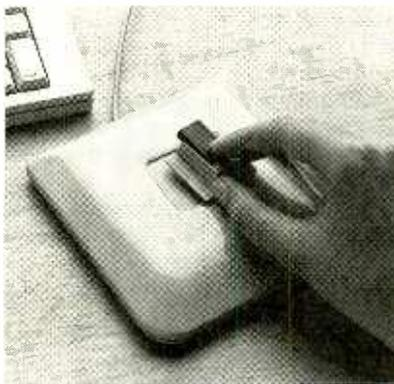
puters and is under development for IBM PC's, offers a greater degree of accuracy and speed than either mice or trackballs. The on-board microprocessor interprets the speed and direction of the floating button, automatically adjusting the precision to take into consideration the type of cursor movement—broad-stroke or fine-precision—that is being used.
