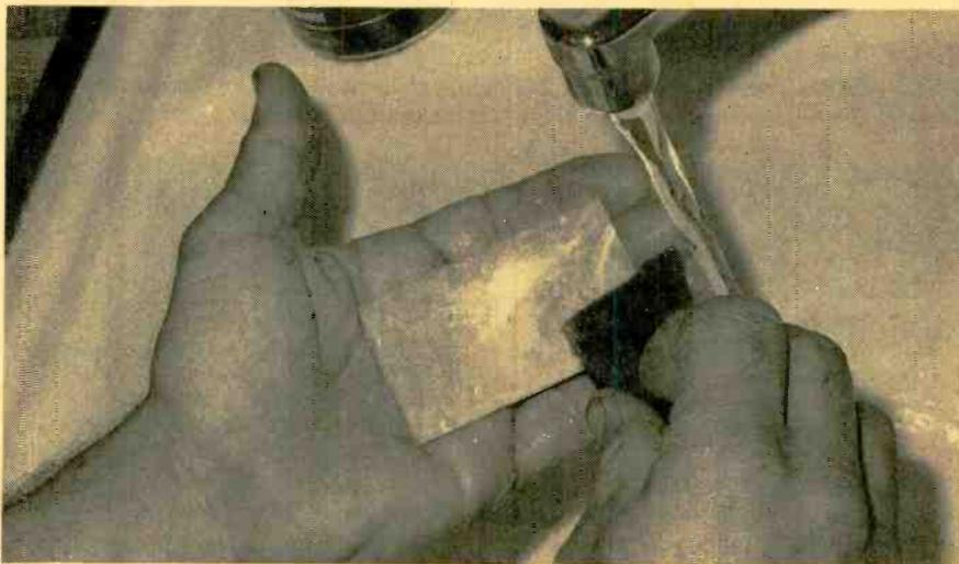
*Before attempting to transfer the printed-circuit pattern from the TEC-200 transparency, make certain that the copper-clad blank is thoroughly clean—free of oxidation, body oils, and anything else that might interfere with the consistency of the pattern being transferred.*
