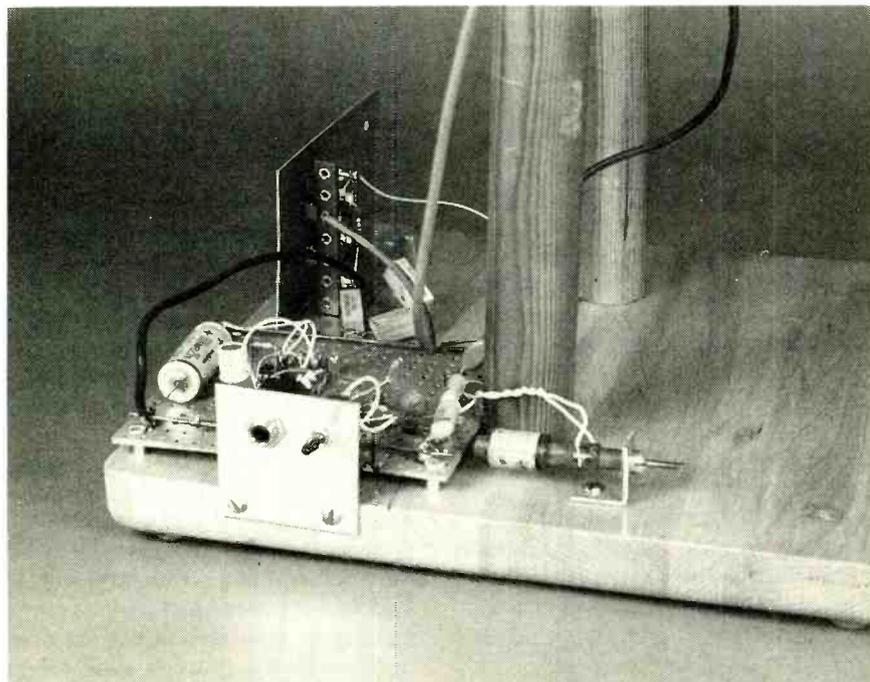
A major portion of the VLF transmitter circuit was assembled on a section of perfboard measuring  $4\frac{1}{4} \times 4\frac{3}{4}$  inches. The remaining circuit components—switches, coils, Q3 (the IRF511 hexFET)—were mounted on the wooden baseboard, and wired to the perfboard-mounted components.
