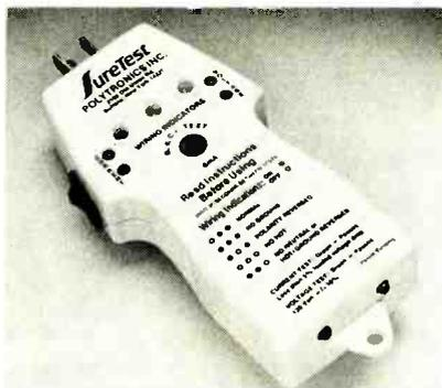
cuit interrupter. Intended for use by electricians, electronic equipment installers, and anyone who requires reliable information on electrical circuits, the SureTest Pro does the work of several individual testers. It features an easy to interpret go/no-go format, automatic test sequencing, microchip solid-state circuitry, and a retractable ground pin. Its proprietary circuitry avoids fuse of defect overheating during testing. An accessory kit is available optionally.
