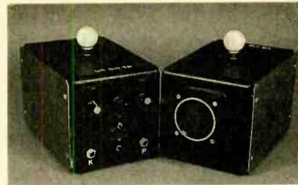
All of the transceiver controls, as well as the headphone output, antenna input, and the piezo transducer are mounted to the panels of the enclosure—the controls and input/output jacks on one end panel of the enclosure and the transducer on the opposite end.
