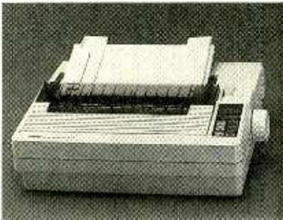
are not wasted, as paper is advanced to the tear-off position at the end of printing and automatically returns to the print position when printing resumes. A "paper-park" function allows fanfold paper or forms to remain in the printer while single-sheet paper or envelopes are printed.
