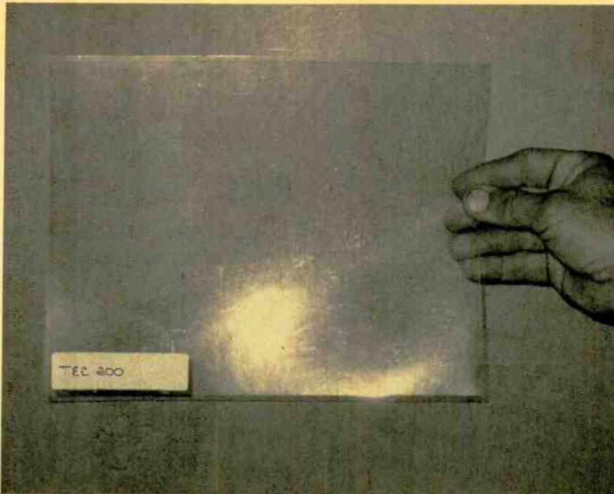
*With a sheet of TEC-200 plastic film, a plain paper copier, and an iron, you can produce a professional looking printed-circuit board.*
