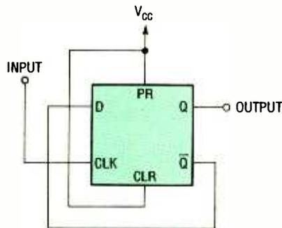
Fig. 4. The D-flip-flop can be configured to function as a toggle (T) flip-flop by connecting the D input to the  $\bar{Q}$  output, and connecting both the PR and CLR inputs to the positive supply rail, as shown here.
