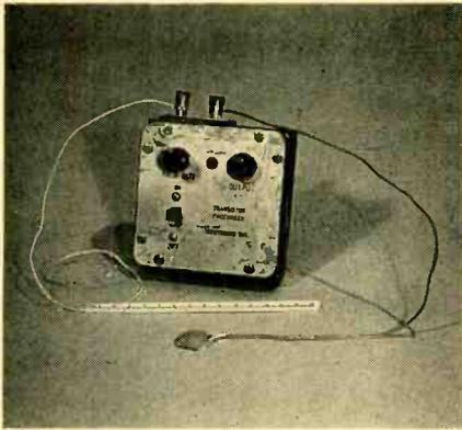
*The first wearable external pacemaker designed and assembled by Earl Bakken in 1957. The two knobs control pulse rate and the pulse's output amplitude. The quality of the construction appears very much like a hobbyist's project.*
