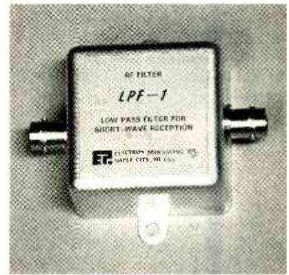
signals below 30 MHz are virtually unaffected. The device uses a two-stage low-pass filter network that requires no power. It is housed in a compact 2 × 2 × 1-inch metal enclosure with BNC female connectors provided for easy connection.
