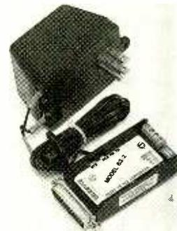
as high as 38,400 BPS, and can support Pin 2, TD (transmit data) and Pin 3, RD (receive data) RS-232 interface signals. Those signal can be interchanged using the unit's DTE-DCE selector switch to allow interfacing to CRT terminals, modems, or computers. "TD" and "RD" LED's indicate the unit's operating status. Power is supplied by a wall-mounted transformer.
