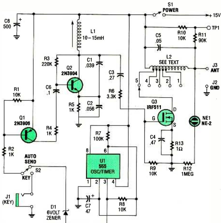
Fig. 1. The VLF Transmitter circuit is built around three transistors and a single 555 oscillator/timer, and requires an external 15-volt, 1-amp power supply. Transistor Q1 functions as a keying device, Q2 is configured as an inductor-tuned Colpitts oscillator, while Q3 is essentially an electronic switch.
