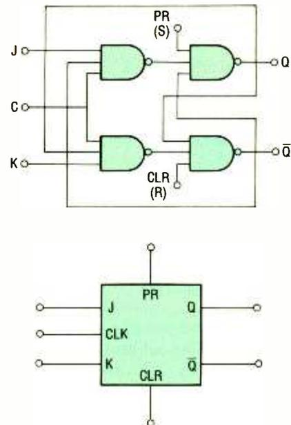
Fig. 5. The J-K flip-flop can be fabricated from a number of gate combinations. A J-K flip-flop assembled from NAND gates is shown in A. Note that the set (S) and reset (R) inputs are now called the preset (PR) and clear (CLR). The schematic symbol for a J-K flip-flop is shown in B.
