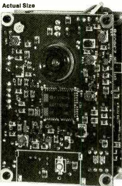
The Chinon CX-101 Monochrome Camera is so small, it can easily fit into a standard electrical outlet box. Its 4.5mm wide lens provides high resolution images of everything from loading docks to a baby's crib—all in lighting conditions as low as 2 lux. It can even view highly detailed subjects as close as 10mm from the lens. The CX-101 uses a composite video signal and a standard 12 volt DC power supply for easy hook up to any TV monitor.
