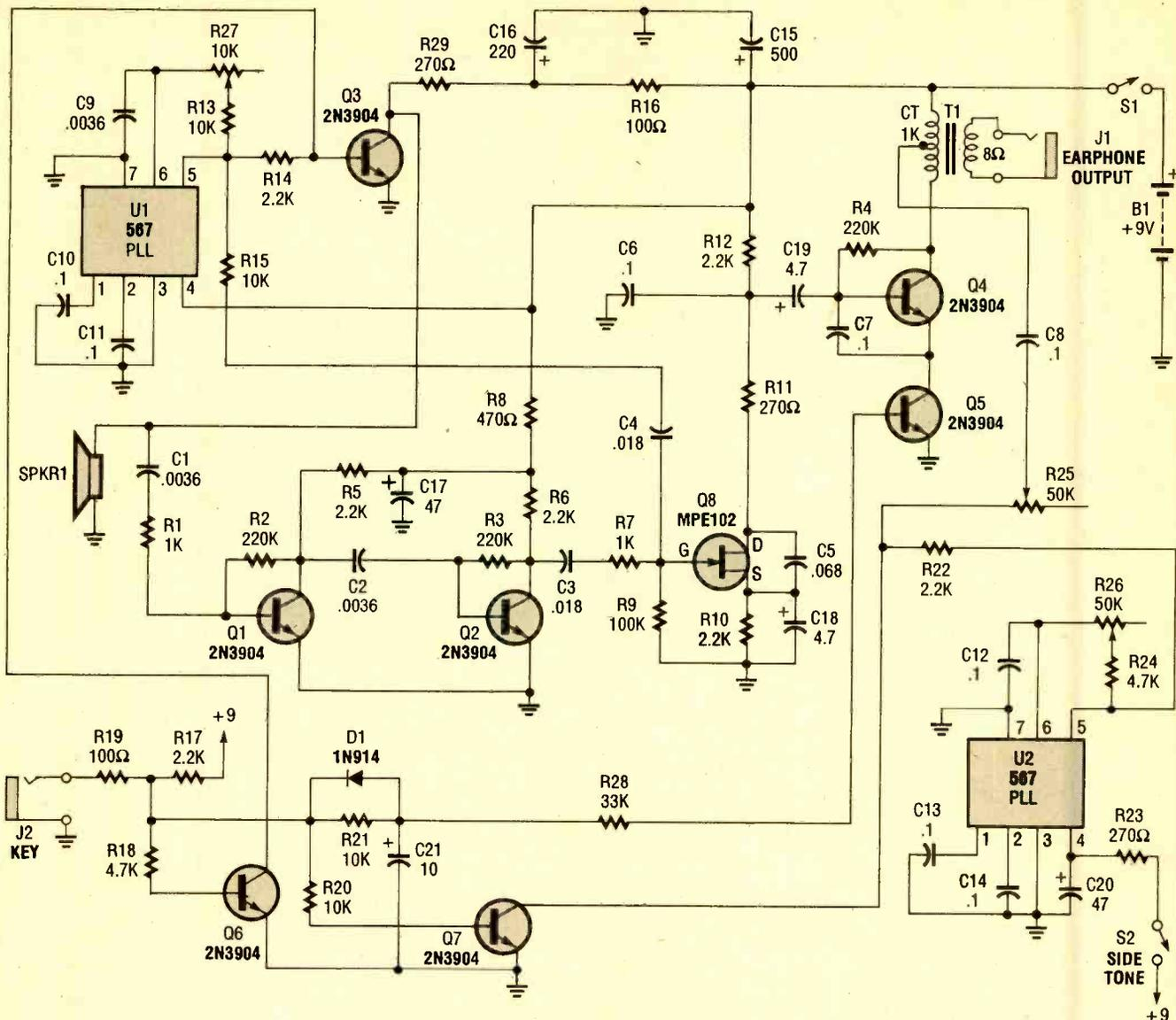
Fig. 1. The Ultrasonic CW Transceivers consist of little more than a pair of 567 phase-locked loop IC's and eight transistors—seven 2N3904 general-purpose NPN silicon transistors and one MPE102 N-channel JFET. The remaining circuit elements are nothing more than support components.
