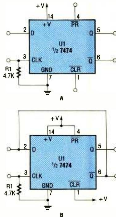
Fig. 8. You will need to duplicate these circuits to follow our experimental procedure. The circuit in A will help you learn about normal D-type flip-flop operation, while the one in B will turn the IC into a T-type.
