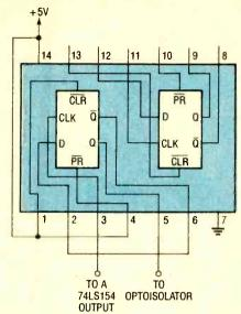
Fig. 3. You can configure any of the outputs for toggled operation by adding a D-type flip-flop as shown. (Note only one flip-flop in the package is wired ready for use.)
