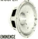
12" woofer made in the USA by Eminence Paper cone and dust cap with treated cloth surround. 80 oz magnet. 2-1/2" vented voice coil. 8 ohm, 170W RMS 235W max 40-4.5KHz response
