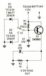
Fig. 4. This simple regulator circuit uses a power transistor in a common- or grounded-base configuration.
