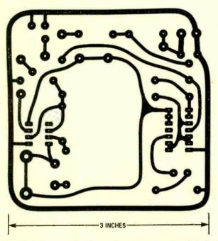
Fig. 2. While there is nothing critical about the construction of the  $3 \times 3$  Alarm to preclude its being built on perfboard, printed-circuit construction is recommended for ease of assembly. Here's the author's printed-circuit board foil pattern.
