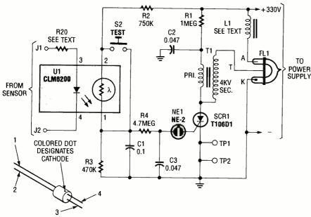
Fig. 1. The SentryStrobe is built around a trigger transformer, a Xenon flash lamp, an SCR, and a neon lamp (which is used to trigger the SCR). A CLM6200 optoisolator/coupler accepts trigger inputs from an external signal source to fire the strobe circuit.
