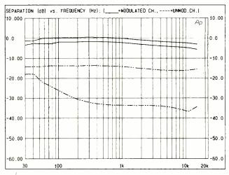
Fig. 5. With strong input signals (outer traces), stereo separation reached more than 33 dB at mid-frequencies. For weaker signals (inner traces), at 45 dBf of input, separation decreased to just over 10 dB.
