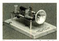
The author's prototype of the SentryStrobe was mounted on stand-offs to block of wood for testing. The dark object between the two capacitors is the 500-ohm, 25-watt ceramic power resistor (R6) used in the power-supply circuit.
