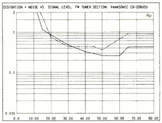
Fig. 4. This plot shows distortion plus noise versus input signal strength. The solid trace is for mono; the dashed trace is for stereo.
