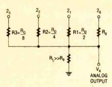
Fig. 1. The analog output voltage  $(V_A)$  of our resistor divider can be most easily found through Millman's theorem, which states that the voltage appearing at any node in a resistive network is equal to the sum of the currents entering the node divided by the sum of the conductances connected to the node.
