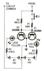
Fig. 3. The AC/DC Indicator can help you in your electronics lab by distinguishing between AC and DC signals, and more.
