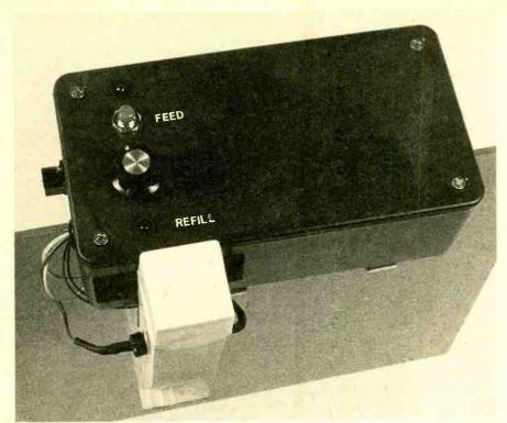
Four holes were drilled in the lid of the enclosure to accommodate SI (MANUAL FEED), LEDI (POWER ON), LED3 (REFILL), and RIO (FEED ADJUST).
