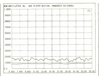
Fig. 10. Using WRMS weighting (lower trace), wow-and-flutter was measured at 0.08%. Using IEC weighting (upper trace) wow-and-flutter averaged about 0.15%.
