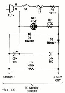
Fig. 2. The power supply for the SentryStrobe is a simple voltage doubler/rectifier circuit, which provides 330 volts DC to the primary winding of the trigger transformer in the strobe circuit.
