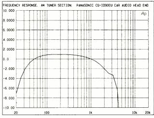
Fig. 6. While the AM frequency response could and should be much better, this tuner still outperformed most AM-tuner sections found in this type of equipment.
