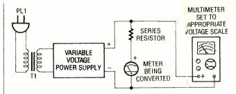
Oops! The multimeter was shown connected incorrec'ly in Fig. 2A of last month's column. Here's the proper method.
