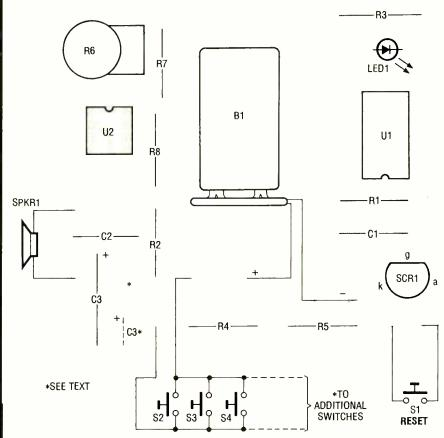
Fig. 3. Once you've obtained the relatively few parts that comprise the  $3 \times 3$  Alarm and etched your circuit board, assemble the project using this figure as a guide.
