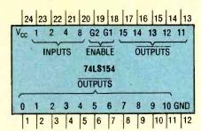
Fig. 1. Here's the 74LS154 demultiplexer's pinout diagram. They decode the output from the computer.
