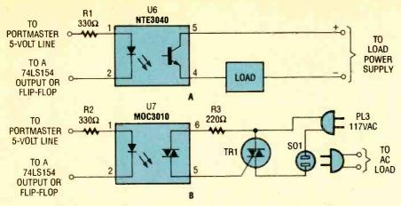
Fig. 4. To control a CMOS-compatible DC load, connect the circuit shown in A. To control an AC device, with or without flip-flop assistance, use the circuit in B.
