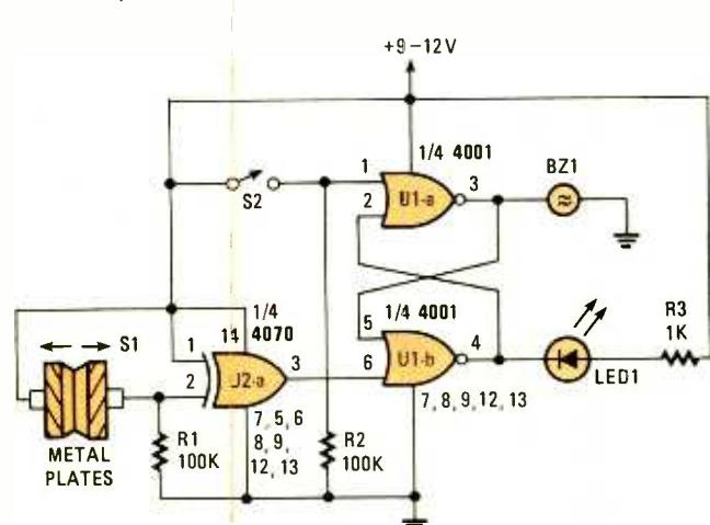
Fig. 9. When this alarm latches, it activates its own buzzer. Note the use of the NOR-implemented R-S latch.
