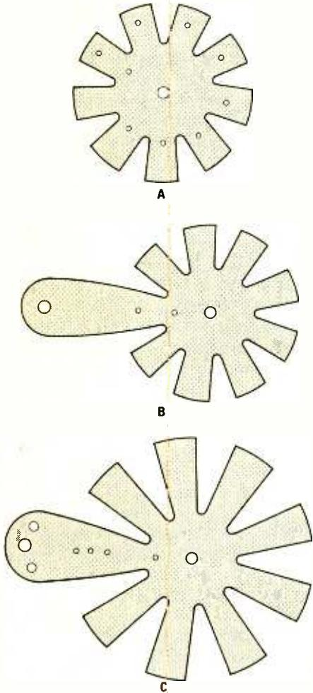
*Fig. 6. Templates for the three coil forms on which the L1-L3 are wound are shown here at half size. The circles on the forms indicate the relative size and locations on the form where holes are drilled to accommodate the coil wires and coil-mounting hardware.*
