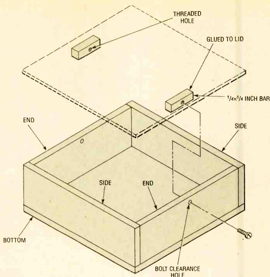
*Fig. 5. Another way to handle lid mounting is to cement lengths of an acrylic bar to the lid on both ends, and drill screw holes through the side or end panels of the enclosure and the acrylic bar.*
