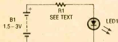
*Fig. 2. Here is the simple circuit that comprises the electrical portion of the Electronic Fish Lure. Note: The resistor (R1) may or may not be needed; that will have to be determined by experimentation.*
