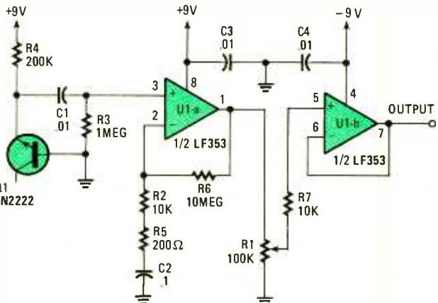
Fig. 10. There are times when noise is useful. This circuit can drive noise signals into any reasonable impedance because of the special op-amps it contains.
