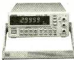
waveforms with crest factors up to 3. Frequency measurements range from 5 Hz to 300 kHz, with a maximum 30,000 count and up to 0.01-Hz resolution.
