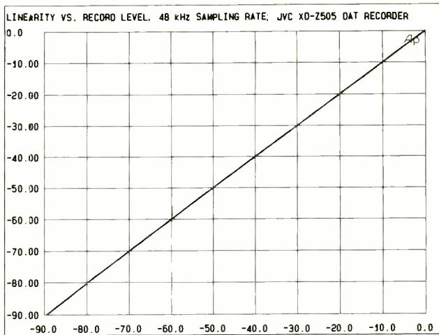
*Fig. 4. One problem with all digital-audio gear is that distortion tends to increase at low levels. However, applying 48-kHz sampling-rate signals to the digital input of this DAT recorder resulted in only a 0.48-dB deviation from perfect linearity at -90 dB.*
