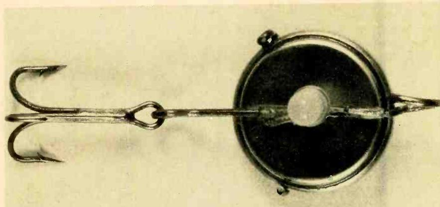
*Here is the finished lure. Under some circumstances, depending on the conductivity of the waters you fish, it may be necessary to insulate the electrical portion of the unit. Should insulating be necessary, a coat or two of fingernail polish works well.*
