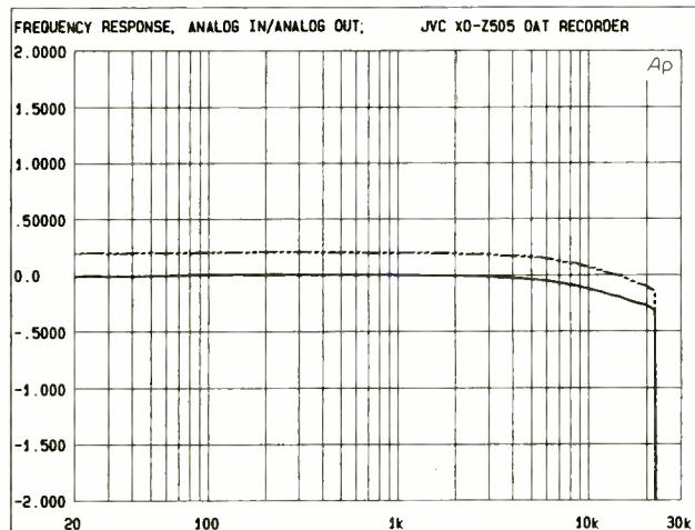
*Fig. 1. The frequency response using the analog inputs was essentially flat out to 22 kHz. At that frequency, response was down only 0.25 dB.*
