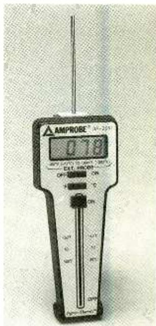
table sensor with a range of -50°F (-46°C) to 300°F (149°C). It has both degrees Fahrenheit and degrees-Centigrade capabilities.
