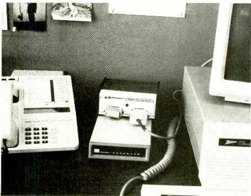
The MSD is shown sitting on top of an ADC MD1202 modem. Its small footprint takes minimal space. The MSD can be situated out of sight since, once installed, it needs no human direct control. Its front-panel LED is useful only during installation and orientation.
