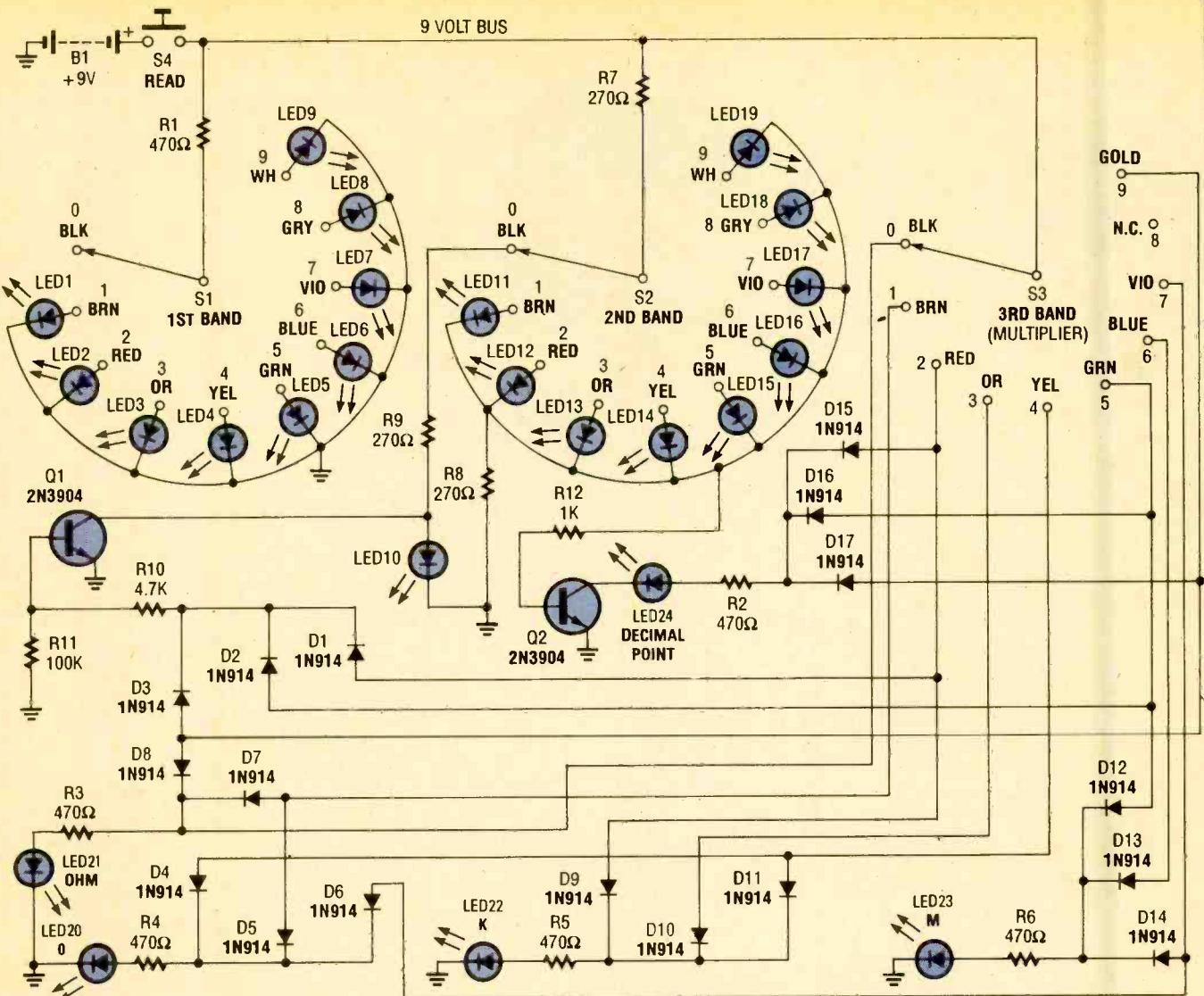
*Fig. 1. Sure-luck Ohms is little more than a well-thought-out switching arrangement—comprised of three single-pole 10-position (SP10T) rotary switches—and LED's to decipher the resistor color code that's stamped on a resistor's body.*
