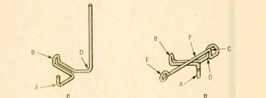
*Fig. 3. Follow this clip-bending diagram to form the battery holder for the Electronic Fish Lure. Starting with a straightened large paper clip, make a bend at point A (A), follow by the bend at point B (B), and then the bend at point D (C). Then form a loop at point C and another at point E (D).*
