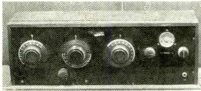
Fig. 3. This 1920's vintage tuned radio-frequency (TRF) receiver has a nice wooden cabinet. Many TRF radios on the market are not communications receivers.
