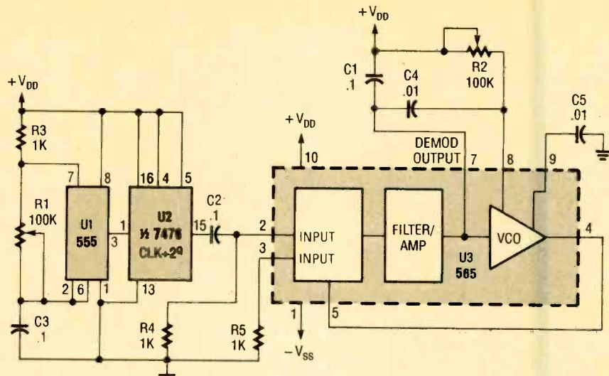
*Fig. 3. A 555 oscillator/timer configured for astable operation supplies a reference signal, which is fed through a flip-flop that's used to divide the signal by a factor of two before it is applied to the PLL. Varying the output frequency of the oscillator will cause a corresponding change in the oscillating frequency of the PLL's VCO.*
