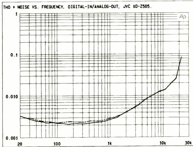
*Fig. 3. Using a 44.1-kHz sampling rate, THD plus noise was approximately 0.002% for a 1-kHz test signal. While distortion did increase with frequency, at worst it never exceeded 0.08%.*
