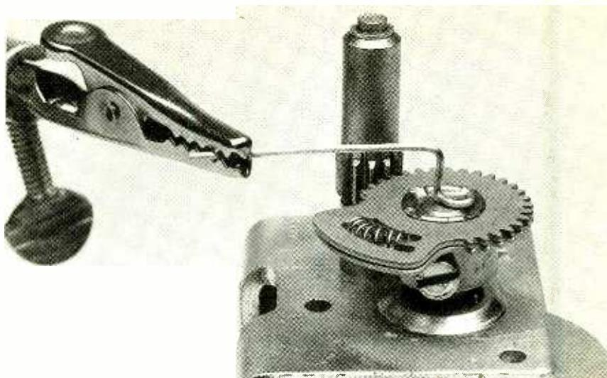
Fig. 3. The dial pointer on the variable capacitor is made from a piece of bare bus wire and is shaped as outlined in the text. The dial pointer is affixed to a gear mechanism with a bit of solder.
