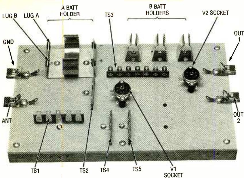
*Fig. 2. Once the terminal strips, Farnsworth clips, battery holders, and vacuum-tube sockets have been mounted, the baseboard of your radio should look something like this. Refer to this illustration for the general layout of the baseboard and the locations of the terminal strips to which the interconnecting wires and components are connected.*
