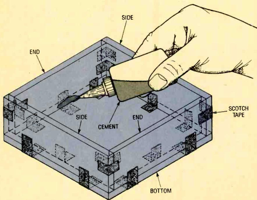
*Fig. 2. Once you have all the parts cut, tape the sides, ends, and the bottom together, making sure that all the joints are tight and square. Then use liquid-acrylic cement to make the joints permanent.*
