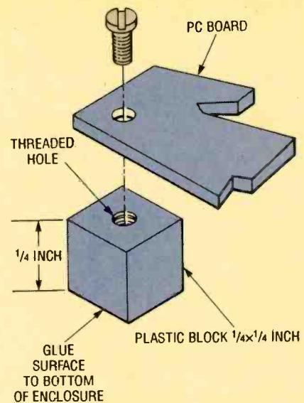
*Fig. 3. Printed-circuit mounts can be added to the enclosure by first screwing 1/4-inch square scraps of acrylic to the board, applying a little acrylic cement to the bottom surfaces of the acrylic squares, and placing the assembly in the desired location within the enclosure.*
