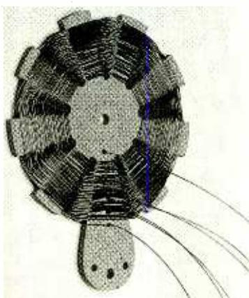
*The rear surface of L2 should look something like this before it is mounted to the frame of the radio. Remember that the taps after turns 48 and 66 consist of two wires each, one coming from and one going to the coil form. The start wire extends up from the small hole on the left. The finish wire is pushed through the small hole on the right after turn 74.*
