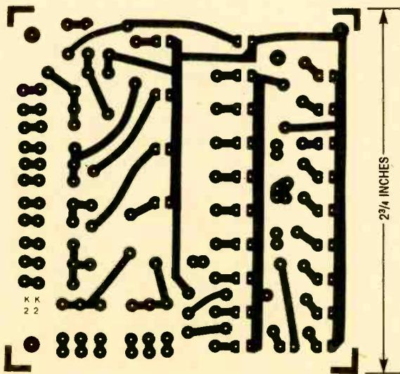
*Fig. 2. To simplify assembly and reduce the possibility of error, printed-circuit construction is recommended. Here's a template for the circuit-board layout used by the author.*
