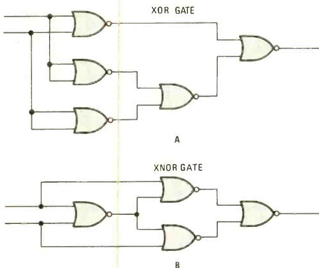
*Fig. 4. The logic required to make an XOR is not only a little complex, it requires five gates, as shown in A. The logic required to make an XNOR gate from NOR gates is a little complex, but we show such a circuit in B.*
