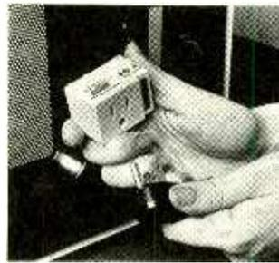
within one nanosecond to protect electronic equipment from hazardous overvoltages, surges, spikes, and transients. It provides protection on all three lines—hot, neutral, and ground. Special hybrid circuitry allows the EG3C to clamp voltages as low as 345 volts, and provides protection from surges up to 6,000 volts.
