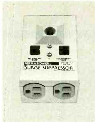
equipment from all power if the device's power-line surge-suppressor element wears out or burns out.
