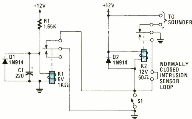
Fig. 5. Most alarms will continue to wail after a power failure whether or not the system has been breached. This circuit just lets you know when power has failed and returned, and it resets itself.
