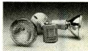
homeowner. It detects motion as far as 70 feet away, providing an effective coverage area of 4000 square feet. The SL-5411 is designed to control up to 500 watts of outdoor incandescent or halogen lighting. Motion-sensor control uses pulse-count technology, which enables it to "take a second look" at the moving object before switching the lights on. That significantly reduces the likelihood of false alarms due to falling snow, blowing leaves, or wind.
