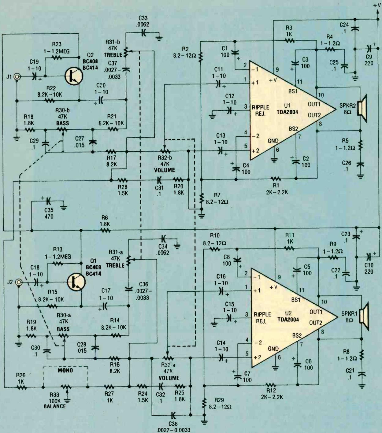
Fig. 1. The 20-watt stereo audio power amplifier is built around a pair of TDA2004 integrated amplifiers. It also has a pair of transistors with a few support components as a preamplifier.
