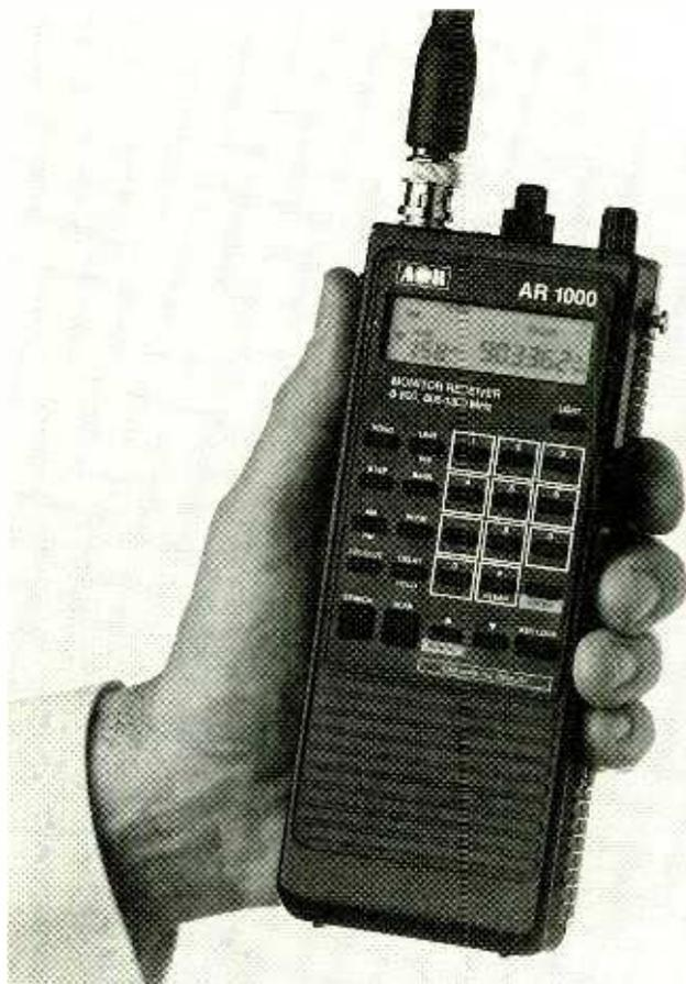
channels. Pairs of upper and lower limits for bands to be searched can be stored in ten separate search-memory locations. All information is stored in permanent memory. Other features include selectable single-channel priority, keyboard lock-out, BNC antenna connector, and a backlit display for night use. The LCD readout offers 21 separate prompting annunciators to make the unit easier
