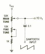
Fig. 3. Here's an alternate tuning network for the spectrum analyzer.
