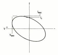
Fig. 6. This curve is typical of a reactance, whether a capacitor or inductor. The three important data points are marked here.
