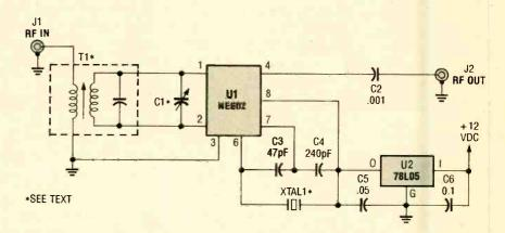
Fig. 5. A quick one-chip converter circuit can be made with the NE602 IC. It requires few components for support and can work over a broad range of frequencies.
