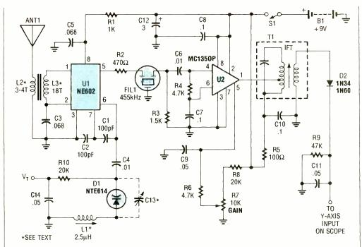
Fig. 2. The schematic diagram for the spectrum analyzer circuit. The circuit is built around an NE602N, which is supported by several semiconductors and passive components.
