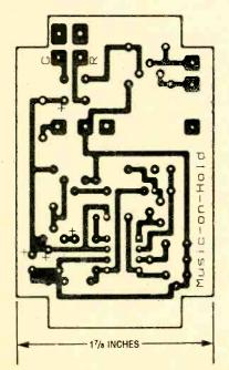
Fig. 2. Here is a full-size template of the printed-circuit artwork for the Music-On-Hold Box's circuit board.
