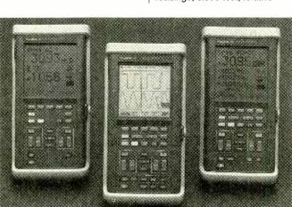
and percent-relative modes; dBm, dBV, and dBW readings; touch hold; and autoranging. Using the included probes, the instruments can make floating high-voltage measurements to 600 volts RMS.
