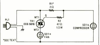
Fig. 6. When this Triac circuit senses current flow through SO1-a, it activates the device plugged into SO1-b. The values of the resistors must be chosen for the specific devices to be plugged in.
