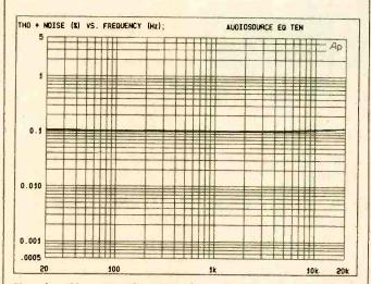
This plot of harmonic distortion plus noise versus frequency showed that the THD plus noise remained virtually constant throughout the test-frequency range. At 0.1% it was certainly acceptable, although considerably higher than the ,008% claimed by the manufacturer.
