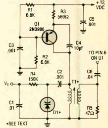
Fig. 6. You can make the circuit of Fig. 5 tunable by replacing its crystal-based local oscillator with this voltage-controlled oscillator. The operating frequency is determined by the voltage at V<sub>T</sub>
