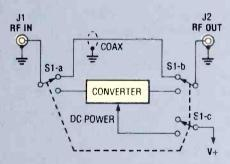
Fig. 2. A converter can be switched in and out of the RF path (between the antenna and receiver) in this fashion.
