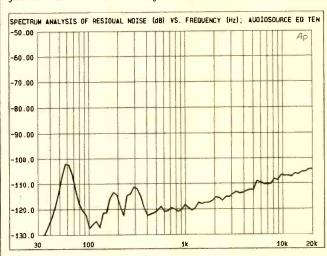
This spectrum analysis of residual noise shows that noise levels are so low as to be inaudible under normal use.
