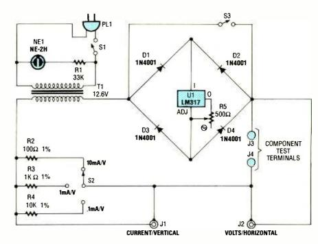
Fig. 2. In the actual EZ-Curve circuit a transformer is the signal generator, a voltage regulator acts as a current limiter, and the precision resistor is switch selectable.
