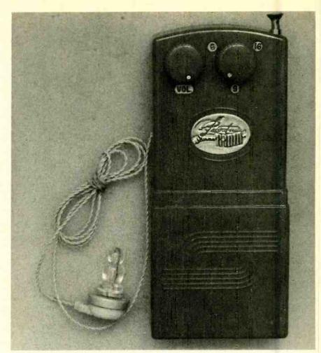
The Privat-Ear pocket radio, measuring only  $5^{15}/_{16} \times 2^{9}/_{16}$ -inches, could easily fit in a pocket for listening on the go.
