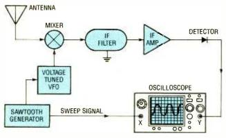
Fig. 1. Block diagram of a spectrum analyzer.
