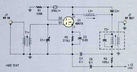
Fig. 3. The mixing of the local-oscillator and tuned RF frequencies occurs in QI in this circuit. The signal is then filtered by T2 to yield only the desired output frequency.
