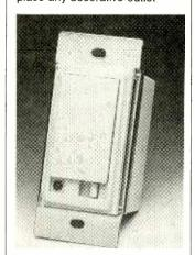
cover over it. Once the switch is activated, the lights begin flashing 24 seconds before turning off. You can keep the lights on continuously by pressing the switch for a slightly longer period of time. The switch controls up to 500 watts of incandescent lighting. It is intended for indoor use only, and cannot be used with three-way circuits.
