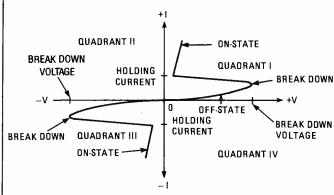
Fig. 2. This is the characteristic curve of a Triac without gate current. It is a plot of the voltage across the main terminals versus the current through them.
