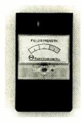
been linked to exposure to low-frequency electromagnetic fields (EMF), Theta Sciences' HFS-Model IV field-survey meter can put your mind to rest. It warns you of the locations and strengths of electromagnetic fields in your home and office, and tells you how far away you should keep to be safe. The battery-operated, handheld unit is easy to use to test everything from your alarm clock to your microwave oven.
