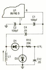
Fig. 4. Using this circuit as the V, input to the spectrum analyzer results in more linear tuning for the circuit.
