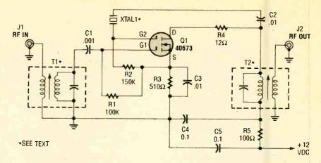
Fig. 4. This circuit is similar to that shown back in Fig. 3, but there is an additional filter used to attenuate the local-oscillator output.
