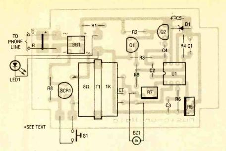
Fig. 3. After you've etched and drilled your board, and obtained the parts listed in the Parts List, assemble the circuit using this diagram as a guide.
