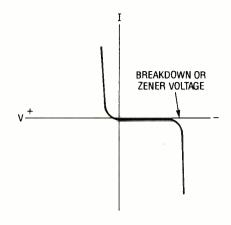
Fig. 5. Zener diodes look like diodes with a poor breakdown region when reverse biased. The breakdown voltage should be approximately the diode's specified Zener voltage.
