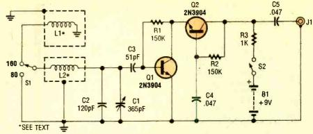
Fig. 1. The Dual-Band Loop Antenna consists of little more than three large loops of wire (LI and L2), two transistors, and a few additional components.
