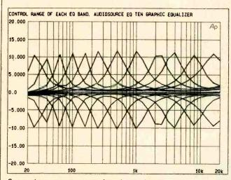
Successive sweeps were used to plot the boost and cut range of each of the EQ Ten's 12 bands. The center frequencies of each band corresponded very closely to the control center points specified.
