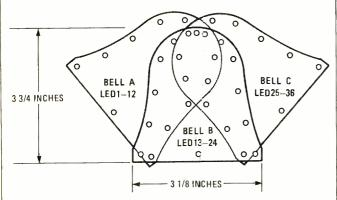
Fig. 2. The 36 LED's of the bell animation circuit are grouped by 12 and arranged to form three bell outlines. Here is the layout of the basic overlapping three-bell outline.
