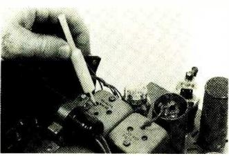
IF transformer tuning screws (here being adjusted, as is proper, with non-conductive tool) may shock a beginner who touches them with a metal screwdriver.
