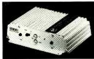
cleaner output. When bass boost is selected, it is fully adjustable from 0-18 dB, centered at 45 Hz. Input sensitivity ranges from 190 mV to 3.5 volts, signal-to-noise ratio is 91 dB, and the damping factor is greater than 80. Maximum current consumption is 10 amps. The amplifier is fully bridgeable,
