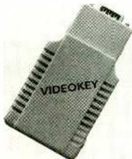
of the on-board VGA card, the Videokey allows any program to be viewed in a large, color format using readily available TV sets and broadcast-standard monitors. The device supports video modes of resolutions up to 640 x 480 with 256 colors. Interconnection is via RCA jacks or S-VHS connectors for improved resolution. All necessary cables and software drivers are included.
